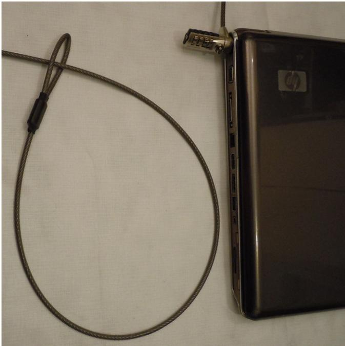
**FIGURE 8-5** Cable lock for a laptop.
