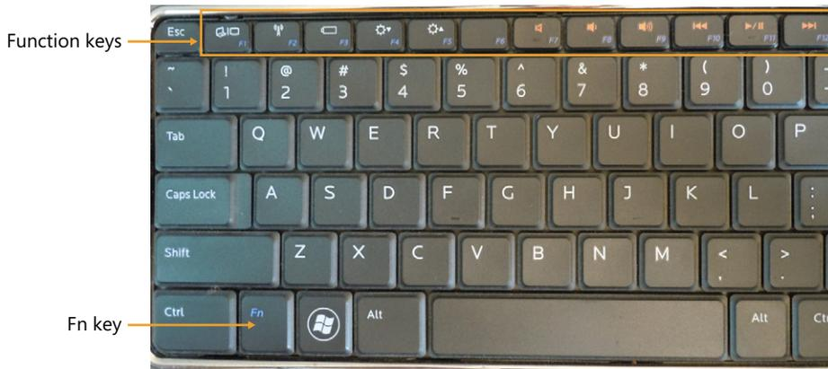
**FIGURE 8-1** Laptop keyboard with Fn and function keys.
