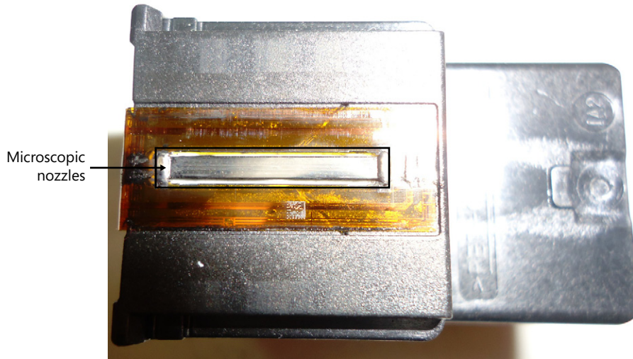
FIGURE 7-13 Inkjet printer print head.
