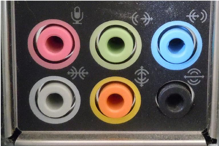
**FIGURE 5-7** Sound connectors for 7.1 system.
