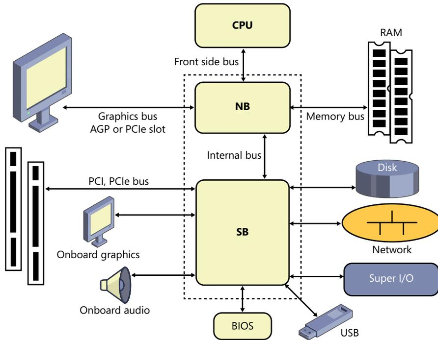
**FIGURE 2-6** North bridge and south bridge chipset.
