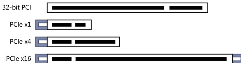
**FIGURE 2-5** PCI and PCIe expansion slot comparison.
