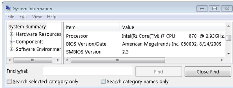
**FIGURE 2-14** Viewing the BIOS version in System Information dialog box.
