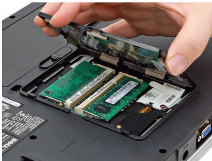
• Figure 26.46 Removing a RAM panel
