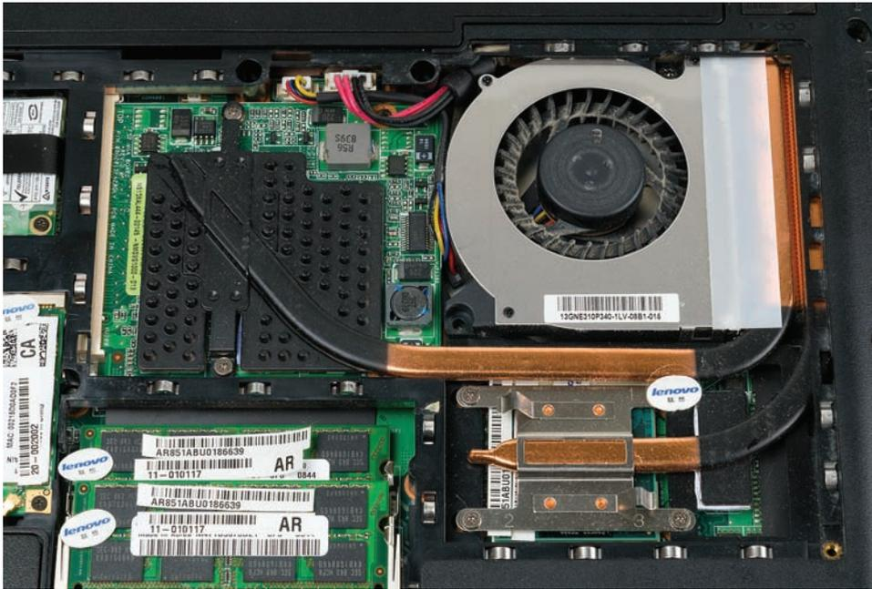
• **Figure 26.53** CPU heat-sink and fan assembly exposed
