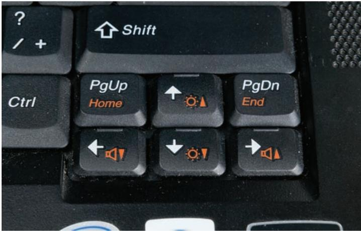
• **Figure 26.36** Keys for adjusting screen brightness
