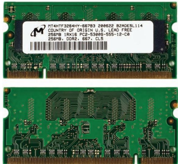
• **Figure 26.45** 200-pin SO-DIMM stick (front and back)
