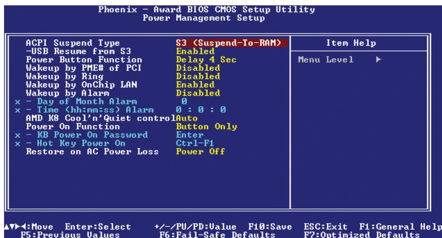
• **Figure 26.31** CMOS with ACPI setup option
