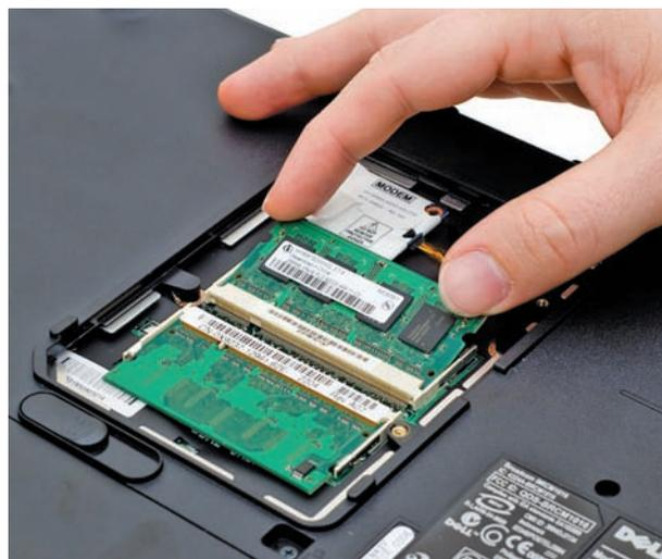
• Figure 26.47 Releasing the RAM
