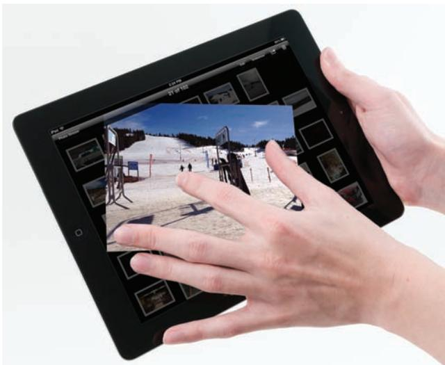
• **Figure 27.5** Resizing and rotating an image using two fingers
