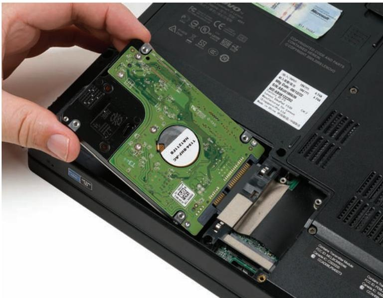
• **Figure 26.50** Inserting a replacement drive
