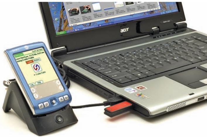
• **Figure 26.24** Devices attached to USB on a portable PC
