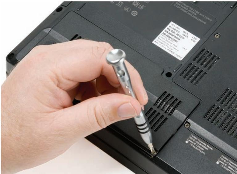
• **Figure 26.49** Removing the drive compartment cover
