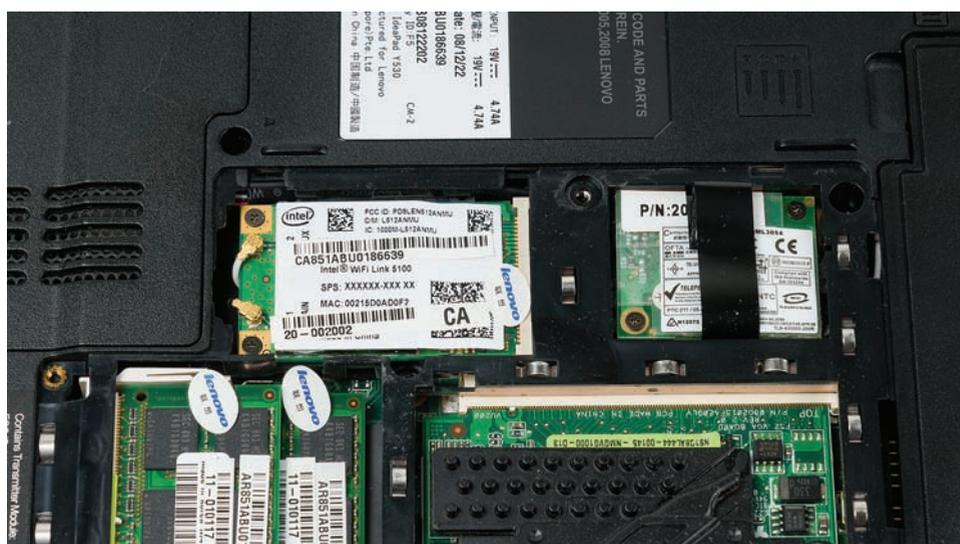
• **Figure 26.52** Mini-PCIe expansion slot on laptop
