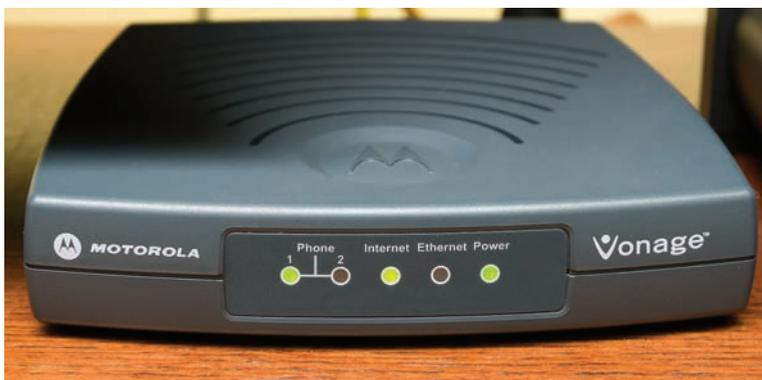
• **Figure 24.47** Vonage Box VoIP phone adapter
