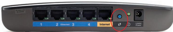
• **Figure 23.10** WPS button on an e2500 Router
