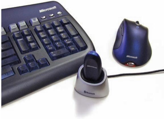
• **Figure 23.6** External USB Bluetooth adapter, keyboard, and mouse
