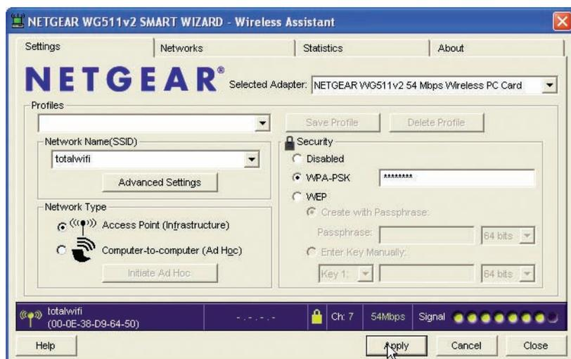
• Figure 23.12 Selecting infrastructure mode in a wireless configuration utility
