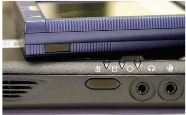
• **Figure 23.1** Infrared transceiver ports on a laptop and PDA
