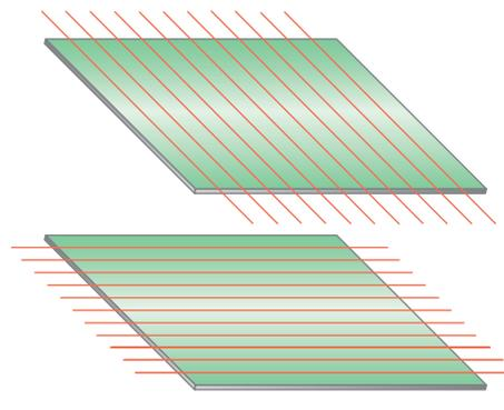
• **Figure 21.17** An LCD matrix of wires
