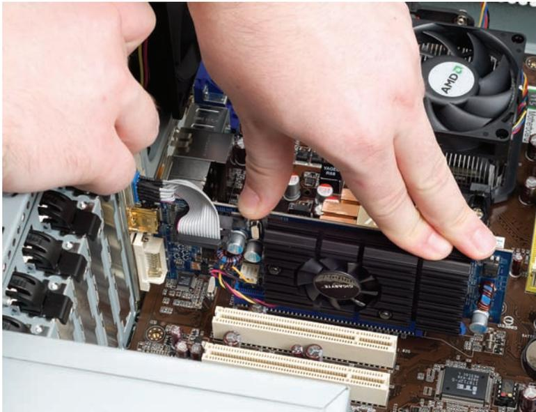
• **Figure 21.50** Installing a video card
