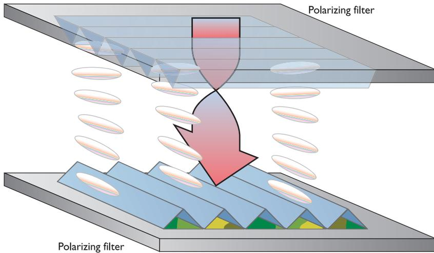
• **Figure 21.13** No charge, enabling light to pass
