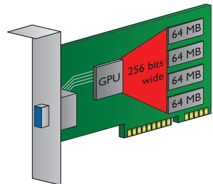
• Figure 21.42 Wide path between video processor and video RAM
