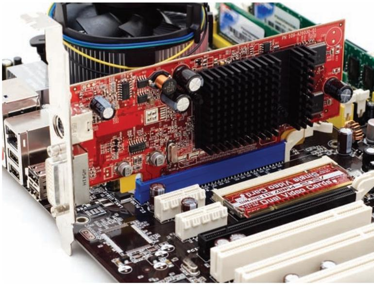
• **Figure 21.40** PCIe video card connected in PCIe slot
