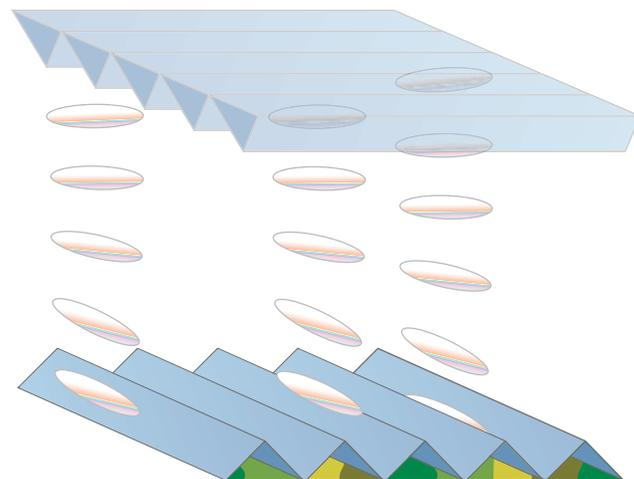
• **Figure 21.12** Liquid crystal molecules twisting
