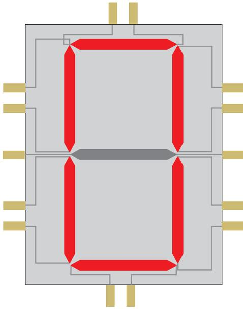
• **Figure 21.16** Single character for static LCD numeric display
