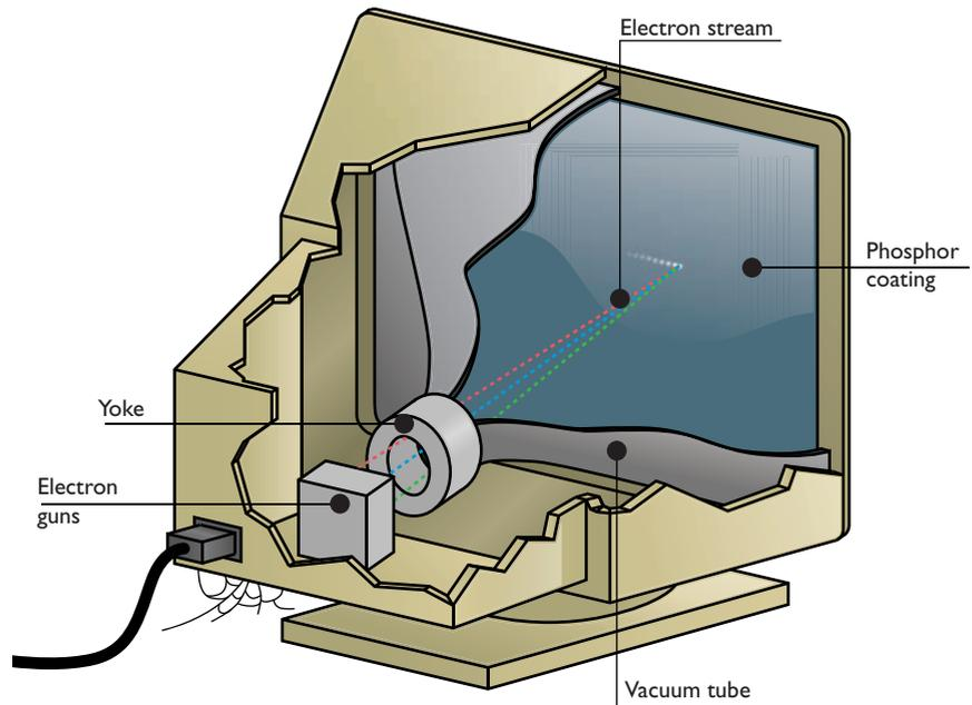
• **Figure 21.2** Electron stream in the CRT
