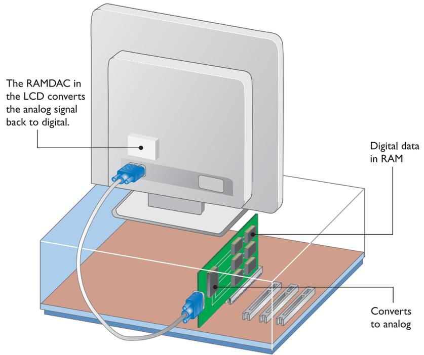
• **Figure 21.30** Converting analog back to digital on the LCD
