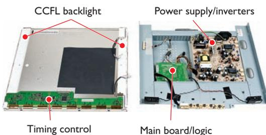
• **Figure 21.77** LCD components labeled
