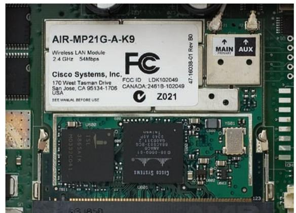
• Figure 9.29 Tiny card in Mini-PCI slot. See the contacts at the bottom of the picture?
