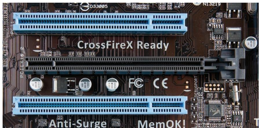
• **Figure 9.30** PCIe  $\times 16$  slot (black) with PCI slots (blue)
