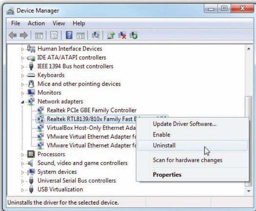
• **Figure 9.37** Uninstalling a device
