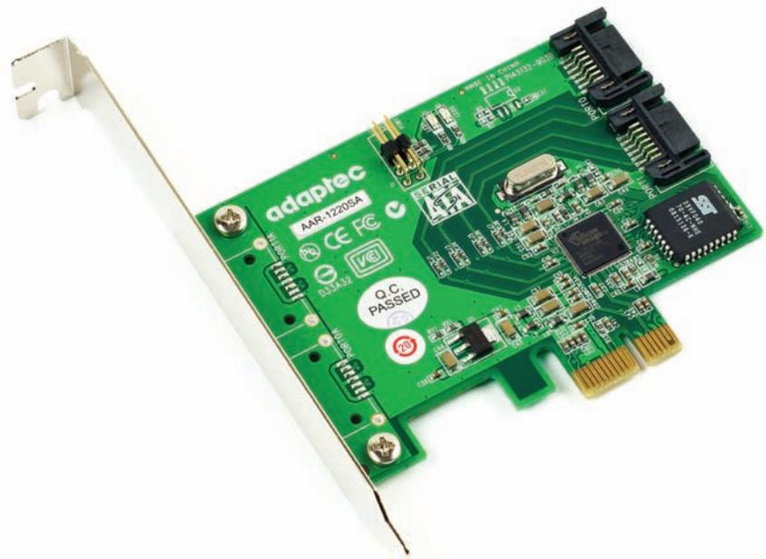
• **Figure 9.51** Adaptec PCIe SATA card
