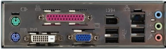
• **Figure 9.8** ATX ports
