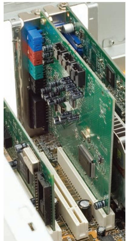
• **Figure 9.35** Properly seated expansion card; note the tight fit between case and mounting bracket and the evenness of the card in the slot.
