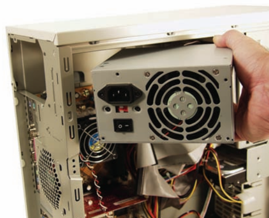
• Figure 10.28 Removing power supply from system unit
