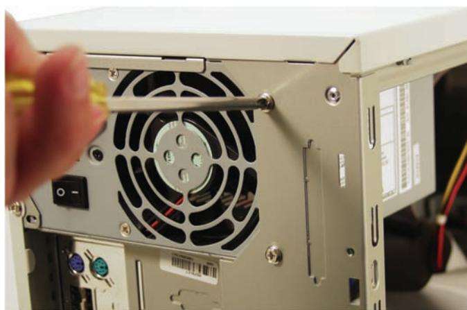
• Figure 10.27 Mounting screws for power supply
