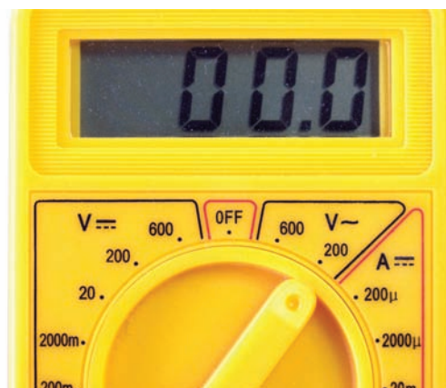
• Figure 10.6 Multimeter featuring DC and AC symbols
