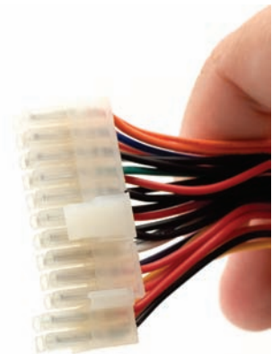
• Figure 10.23 Convertible motherboard power connector
