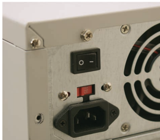
• Figure 10.29 On/off switch for an ATX system
