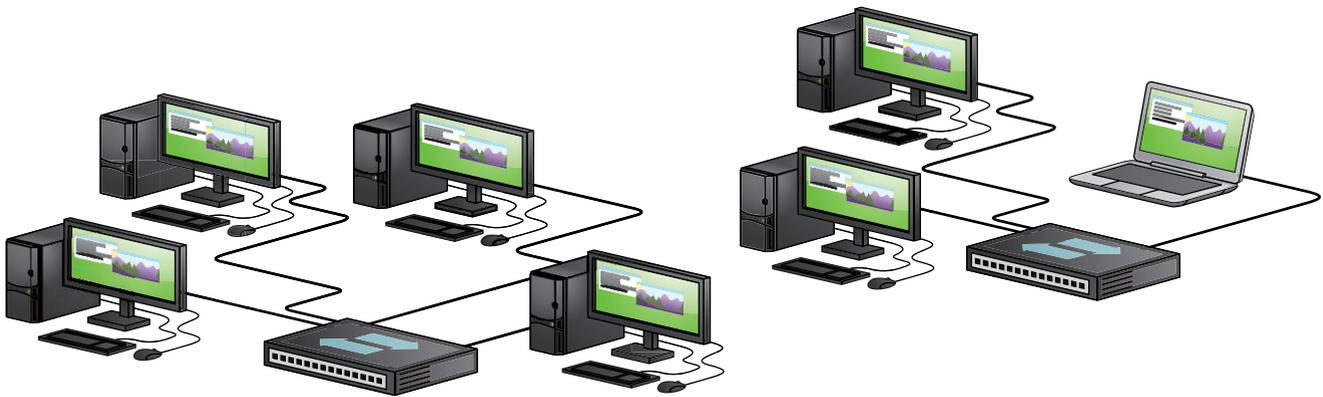
• **Figure 5.15** Two broadcast domains—two separate LANs
