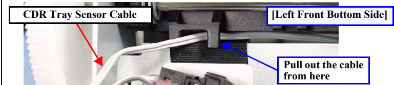
Figure 1-112. Routing the CDR Tray Sensor Cable
