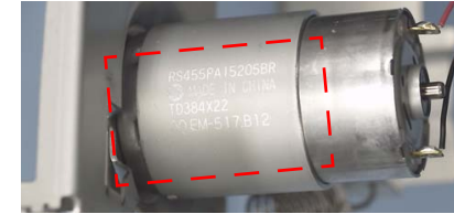
Figure 1-89. Reinstalling the CR Motor
