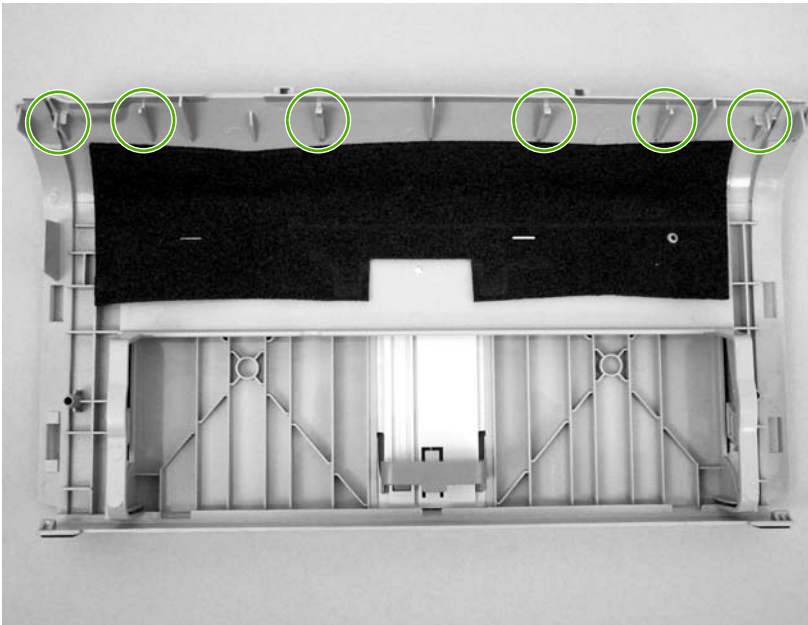
Figure 5-18 Remove the front cover (1 of 3)
