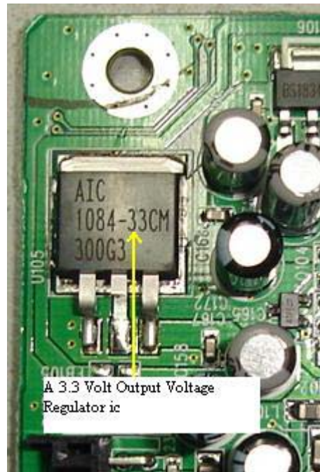
A 3.3 Volts Voltage regulator
