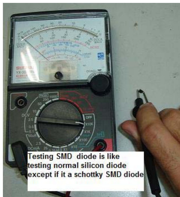
Set to X10K Ohm to test SMD diode
