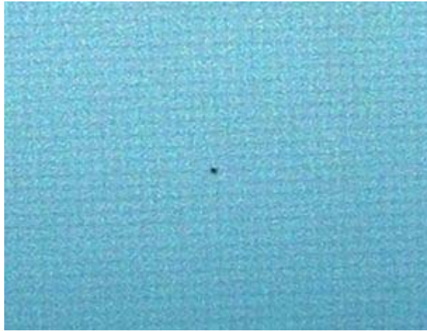
A Dead pixel in LCD Screen
