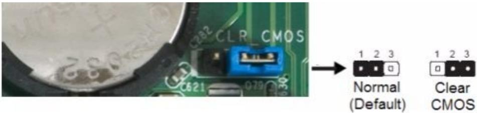
**Method 2:** Another method is to remove the CMOS battery from the system. Removing the battery is usually the second method as it may take anywhere from 15 minutes to 8 hours in order for the CMOS to lose the settings, For immediate clearing Short the Battery terminals on Motherboard. Once the CMOS is clear, you should know by the “BIOS checksum error, press F1 to continue “, or “CMOS Checksum Error - Defaults Loaded” message at bootup.
