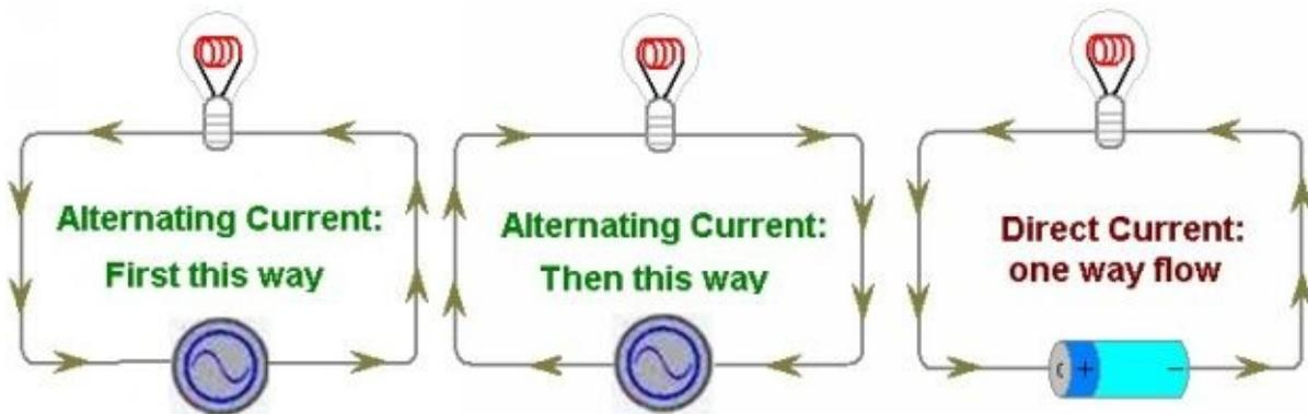
**AC Sources:** 1. Mains, 2. Output from Stabilizer, UPS and Inverter, 3. Generator etc
