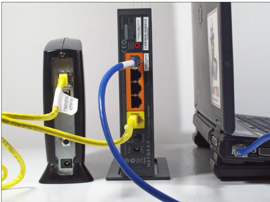
**Figure 3-3:** The laptop, router, and cable modem all hooked up.
