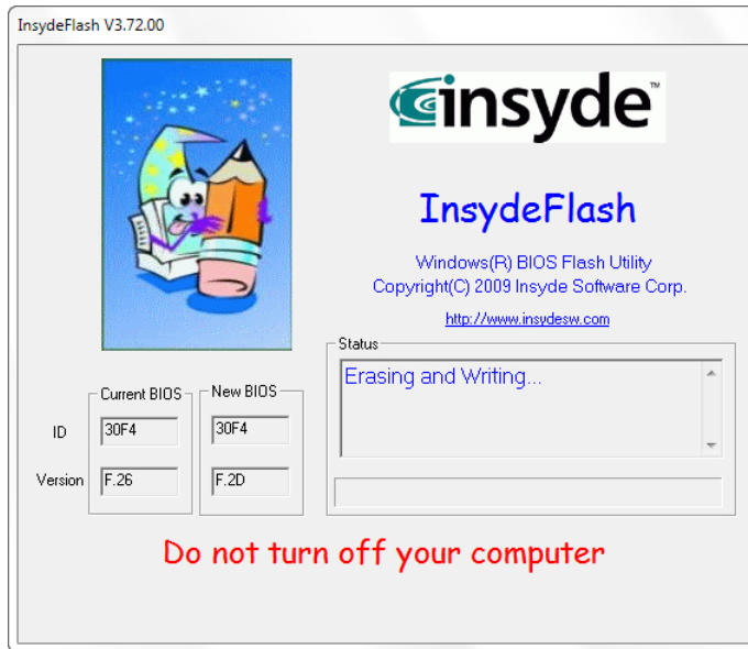
FIGURE 2-15 Flashing the BIOS with a program from the manufacturer.
