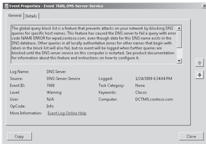
FIGURE 15-27 Event 7600 logged when a query to a name contained in the block list is seen
