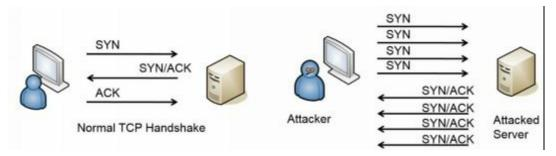
Figure 7.2: TCP handshake and SYN flood attack
