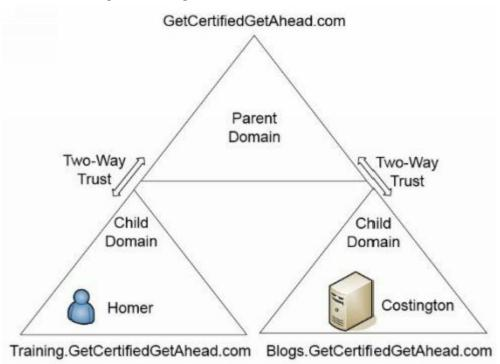
Figure 1.2: An LDAP transitive trust used for SSO
