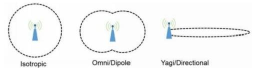
Figure 4.4: Directional and omnidirectional antennas
