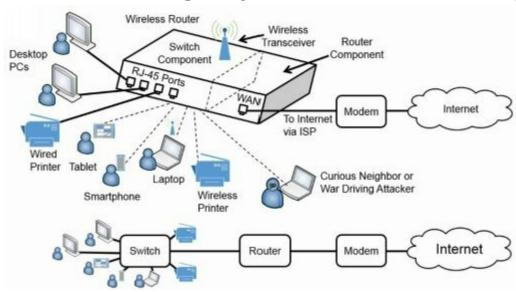
Figure 4.3: Wireless access point with routing capabilities (wireless router)
