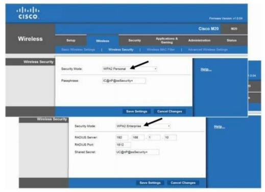
Figure 4.6: Configuring wireless security
