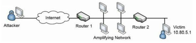
Figure 7.1: Smurf attack through an amplifying network
