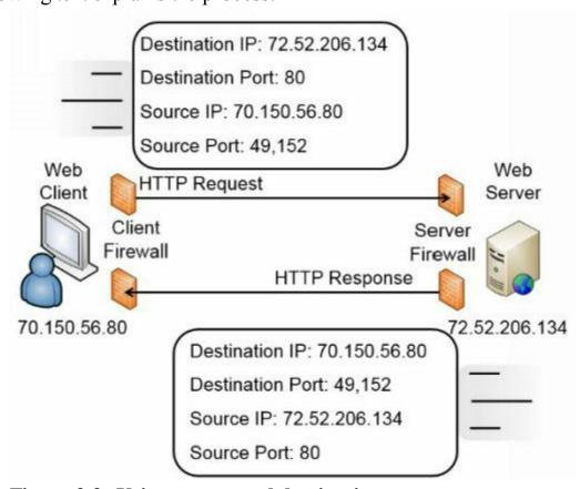
Figure 3.3: Using source and destination ports
