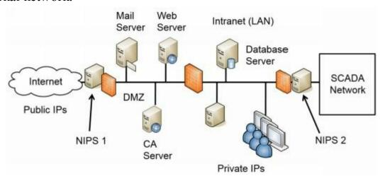
Figure 4.2: NIPS used to detect and prevent attacks
