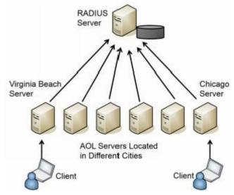
Figure 1.3: Remote Authentication Dial-In User Service (RADIUS) configuration
