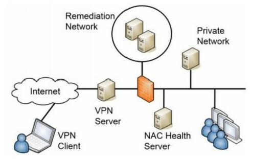
Figure 4.9: Using network access control
