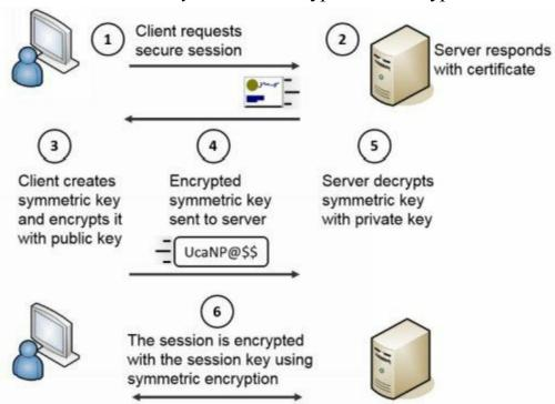
Figure 10.8: Simplified handshake process used with HTTPS
