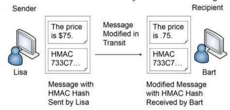
Figure 10.3: Using HMAC
