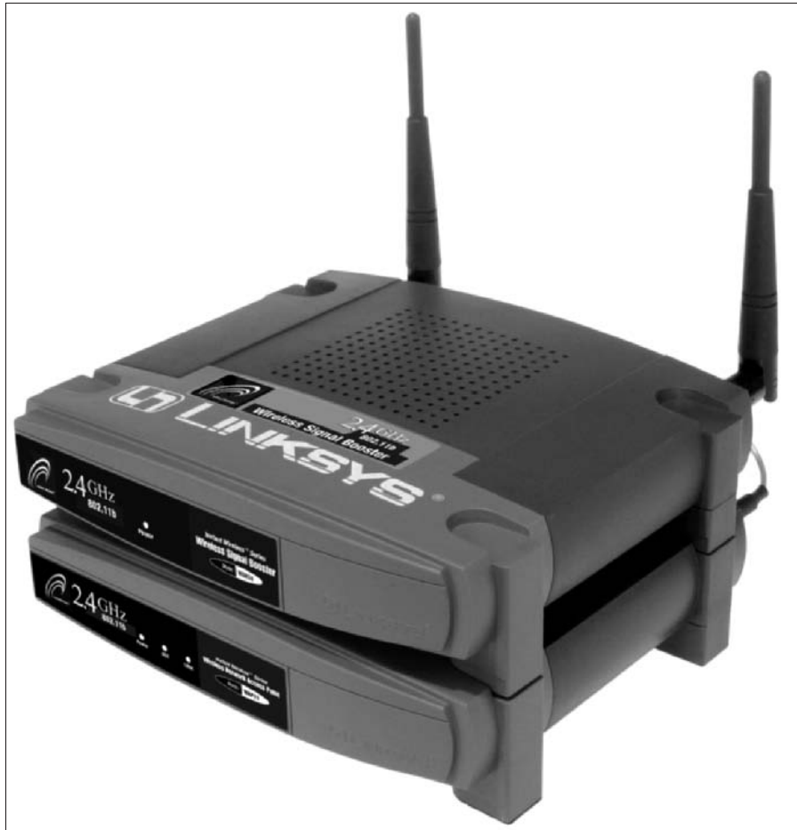
Figure 18-1: The Linksys WSB24 mated to a Linksys wireless access point.
