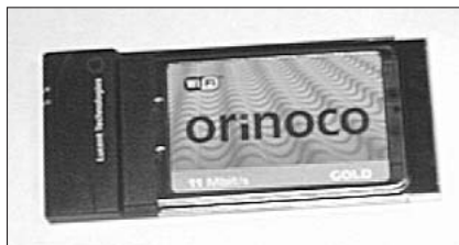
Figure 1-4: A PC Card wireless network interface adapter.
