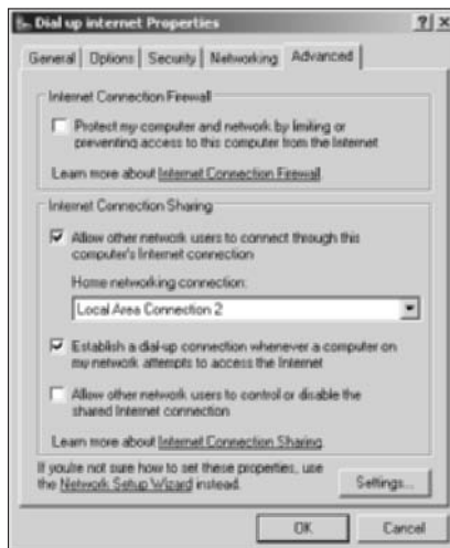
Figure 9-12: Enable Internet connection sharing in Windows XP.
