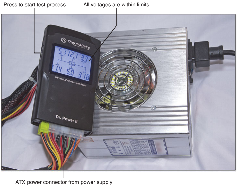
Figure 7.4 This power supply works and provides correct voltage levels.
