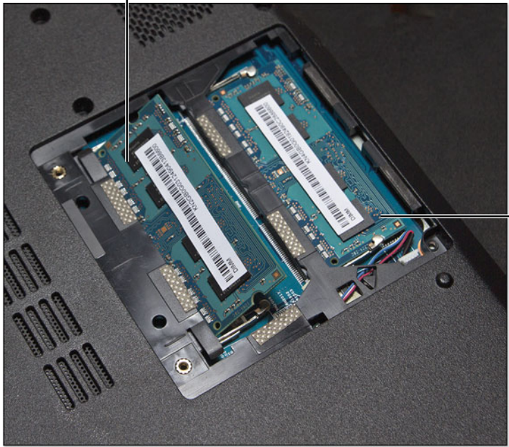
Figure 15.9 Preparing to remove an SODIMM from a laptop.
