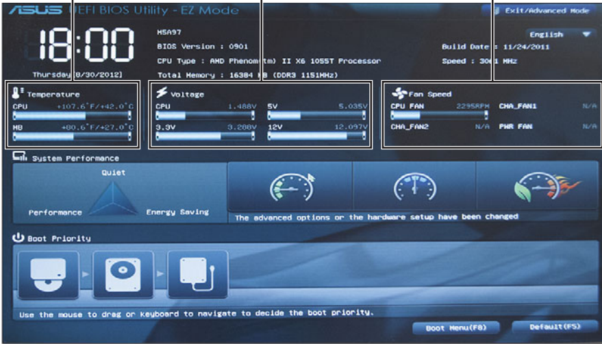
Figure 7.7 A system that displays the system monitor as soon as you start the UEFI BIOS setup program.
