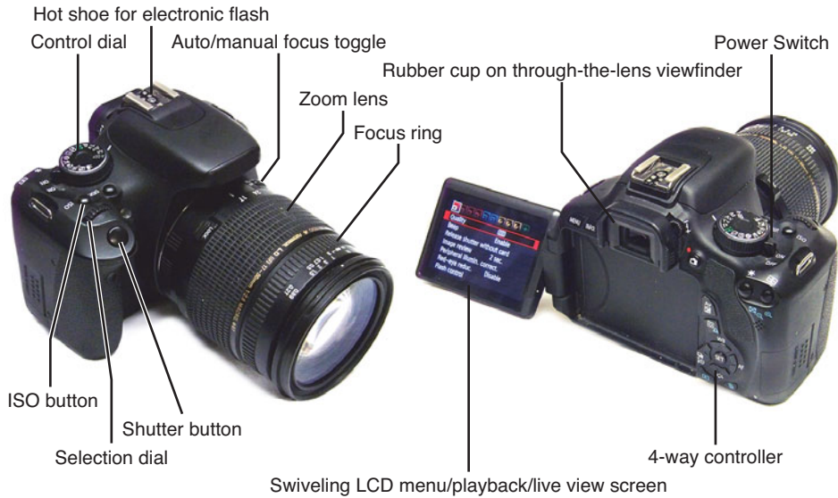
Figure 1.48 Features of a typical digital SLR camera.
