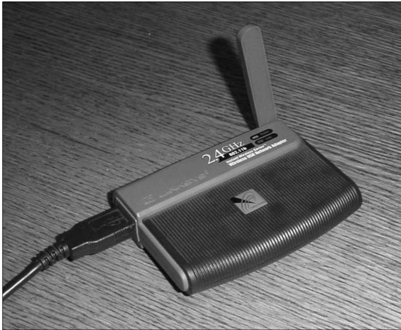
Figure 1-3: A typical wireless networking adapter.
