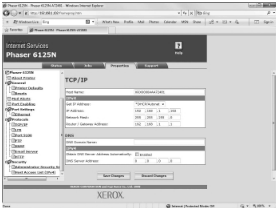
Figure 6-4: Changing network settings via a printer's Web interface.
