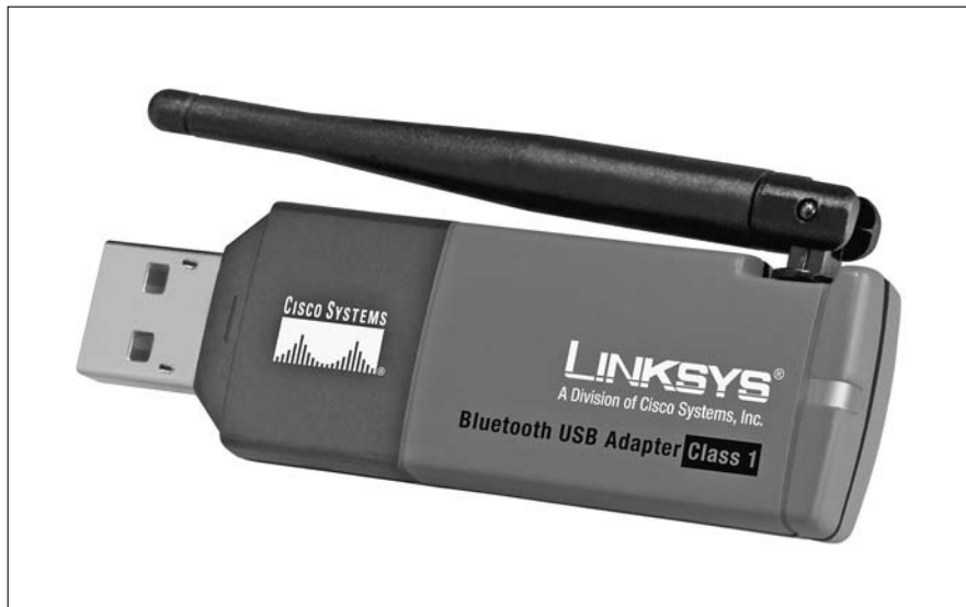
Figure 5-1: A typical USB Bluetooth adapter.
