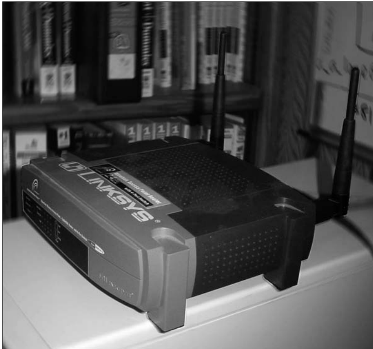
Figure 1-5: A typical wireless router.
