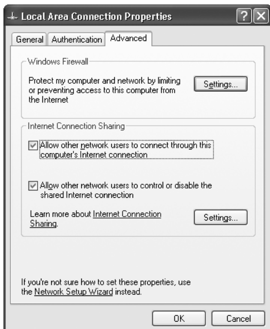
FIGURE 22-10 The Advanced tab of the Local Area Connection Properties dialog box showing Internet Connection Sharing
