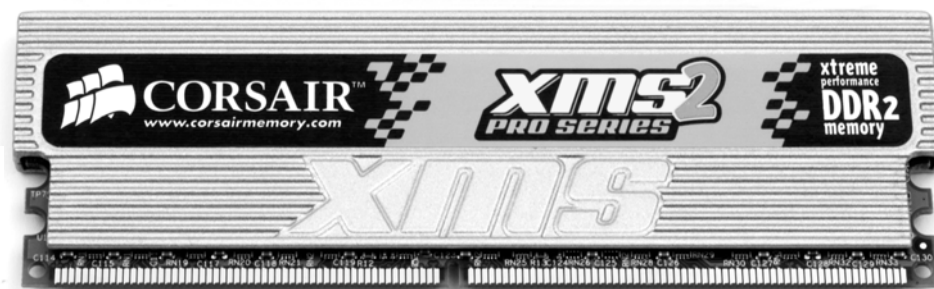
FIGURE 4-7: A 240-pin DDR2 DIMM
