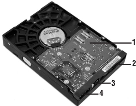
FIGURE 9-5: The external parts of a hard drive
