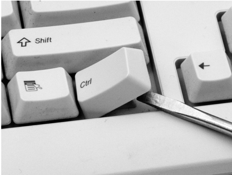
FIGURE 16-3 Removing the CTRL key with a screwdriver
