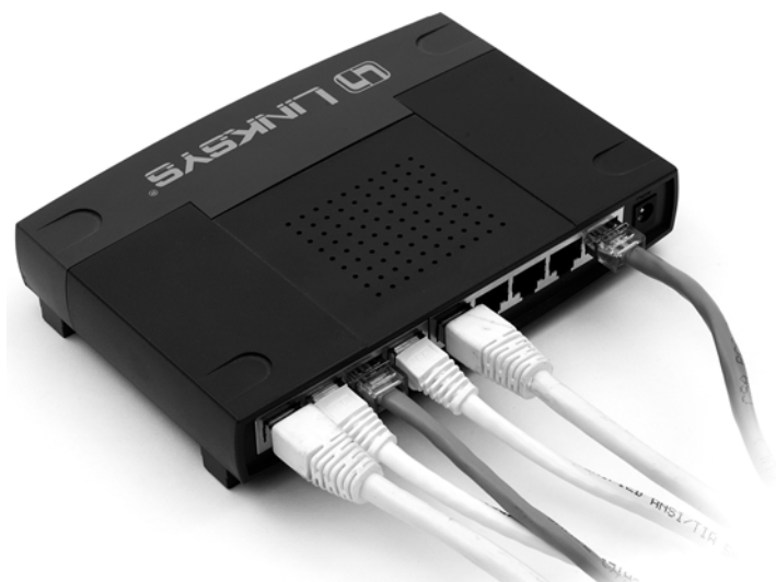
FIGURE 21-2 A LAN hub with multiple cables/devices attached
