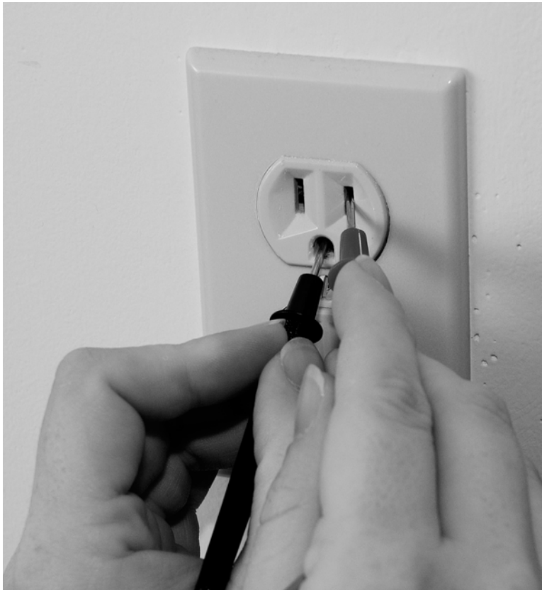
FIGURE 8-4 Multimeter probe locations when testing an AC outlet's hot-to-ground circuit
