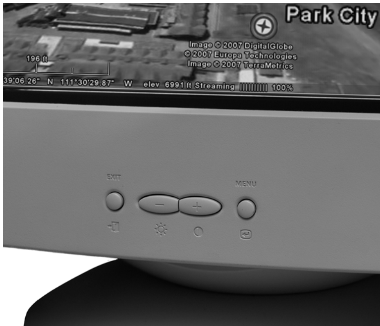
FIGURE 17-3 Front controls on a CRT monitor
