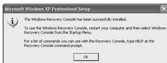
FIGURE 15-15 Completing the Recovery Console installation
