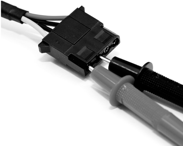
FIGURE 8-7 Measuring the voltage in a Molex connector
