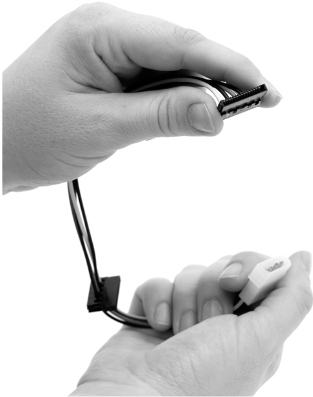
FIGURE 9-7: Molex-to-SATA power adapter
