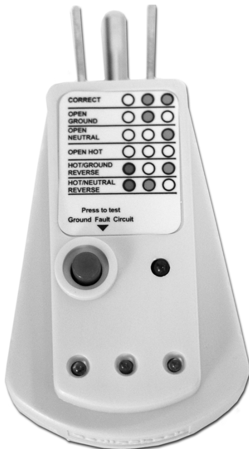
FIGURE 8-2 A circuit tester for AC electrical outlets
