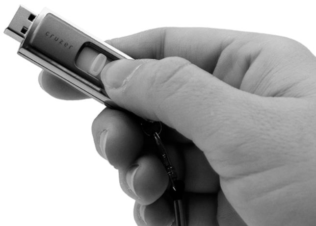
FIGURE 11-5 A USB thumb drive with a retractable connector
