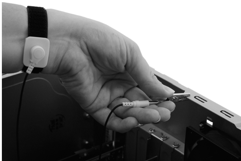
FIGURE 2-7 Proper use of an anti-static wrist strap
