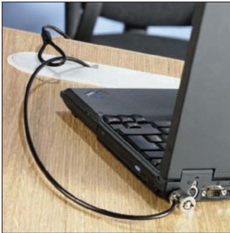
Figure 19-29 Use a cable lock system to secure a notebook computer to a desk to help prevent it from being stolen Courtesy of Kensington Technology Group
