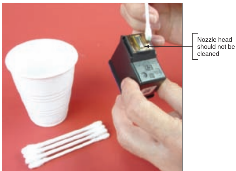
Figure 22-49 Clean the area around the nozzle plate with a damp cotton swab Courtesy: Course Technology/Cengage Learning
