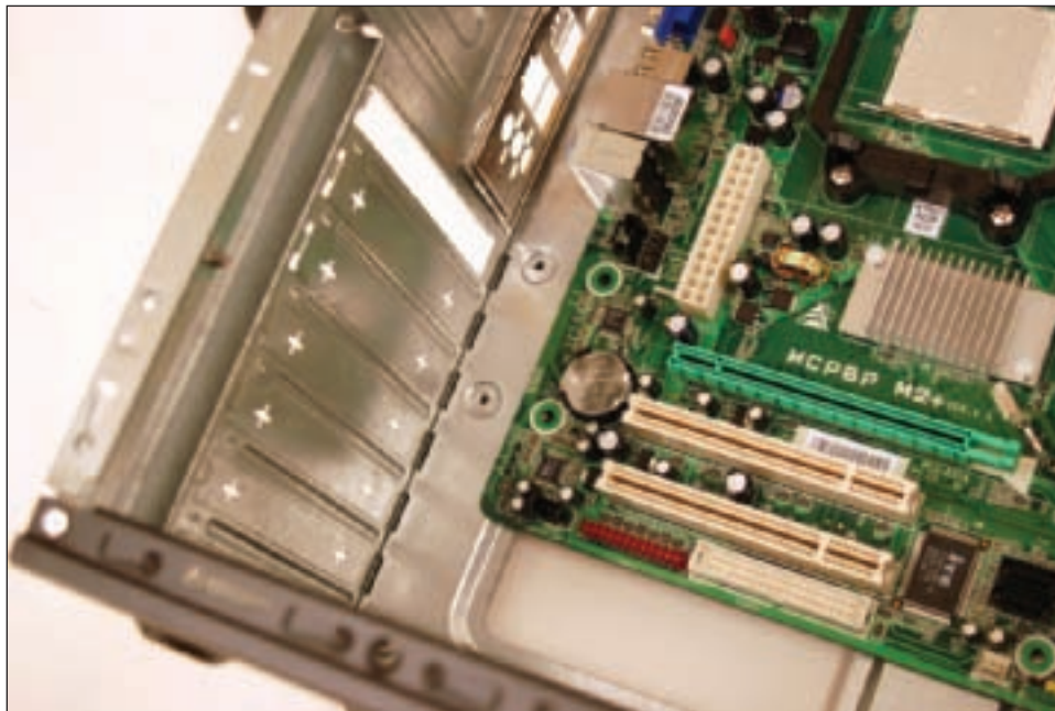
Figure 5-47 Align screw holes in the case with those on the motherboard Courtesy: Course Technology/Cengage Learning
