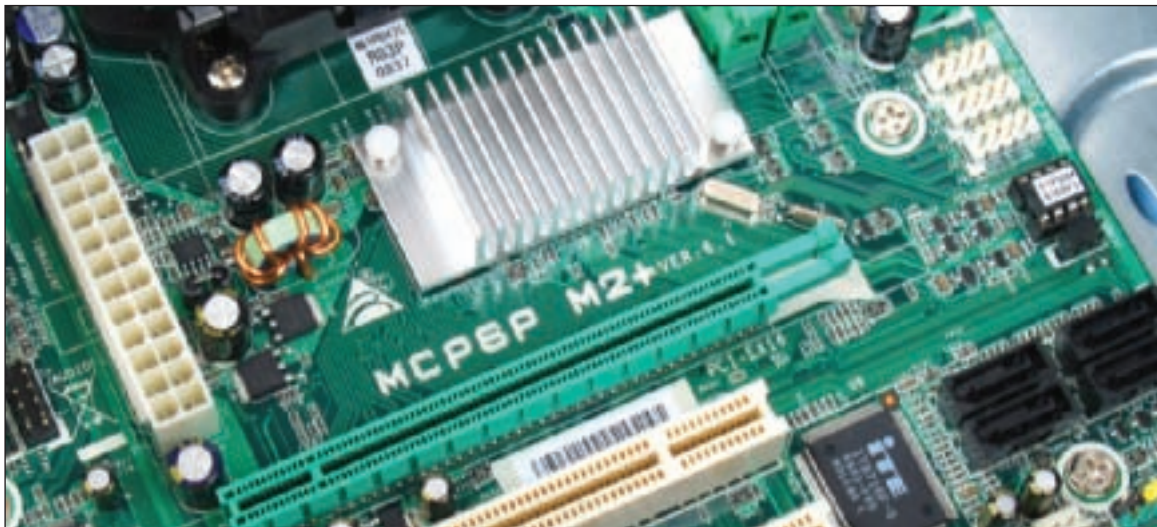
Figure 5-39 The motherboard brand and model are imprinted somewhere on the board Courtesy: Course Technology/Cengage Learning
