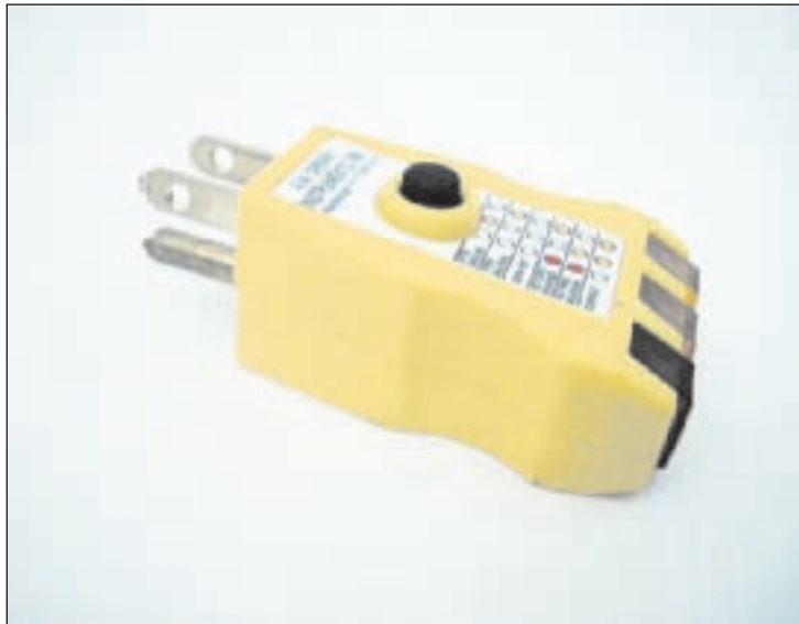
Figure 4-17 Use a receptacle tester to verify that hot, neutral, and ground are wired correctly Courtesy: Course Technology/Cengage Learning
