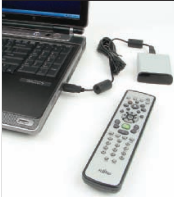
Figure 9-16 This remote control is an infrared device that uses an IR transceiver connected to a notebook by way of a USB port Courtesy: Course Technology/Cengage Learning
