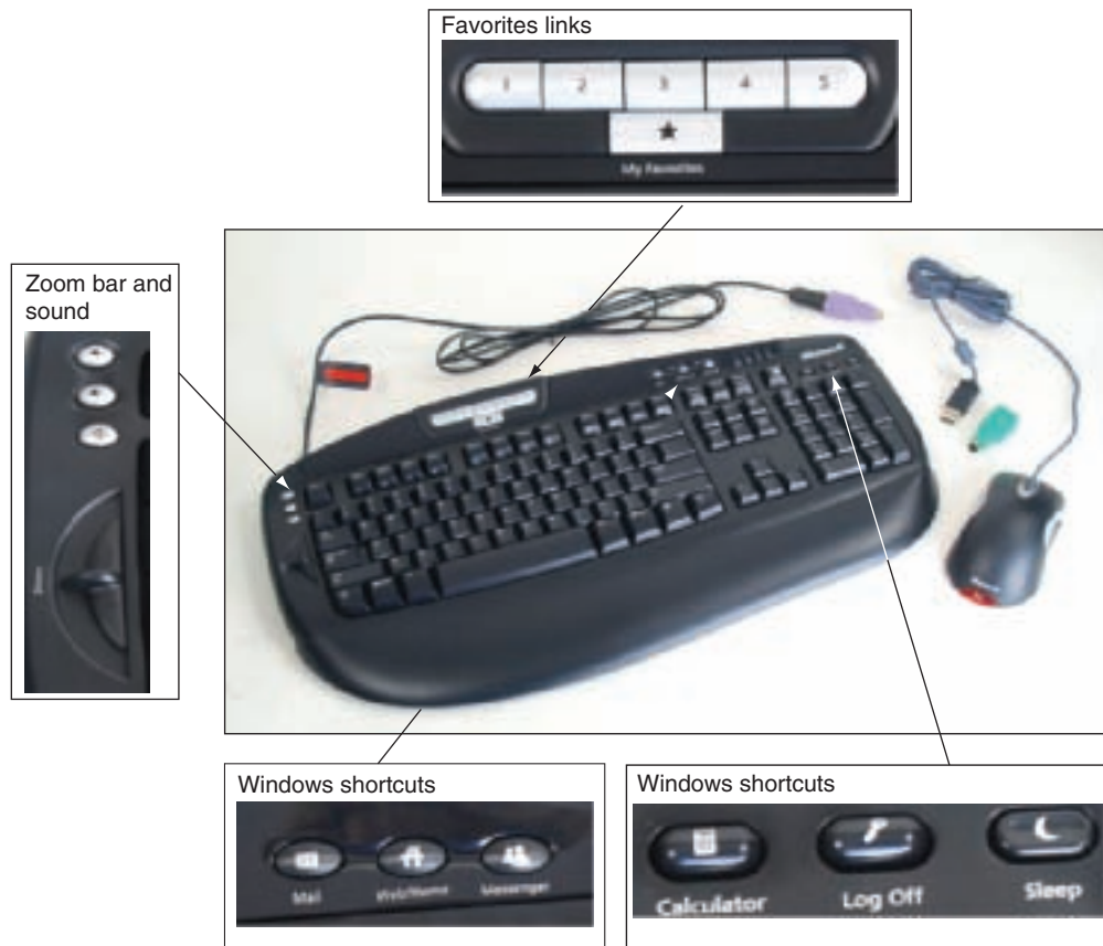
Figure 9-42 The mouse and keyboard require drivers to use the extra buttons and zoom bar Courtesy: Course Technology/Cengage Learning
