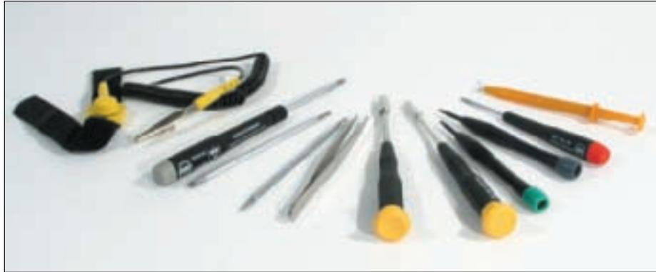
Figure 21-56 Tools for disassembling a notebook computer Courtesy: Course Technology/Cengage Learning
