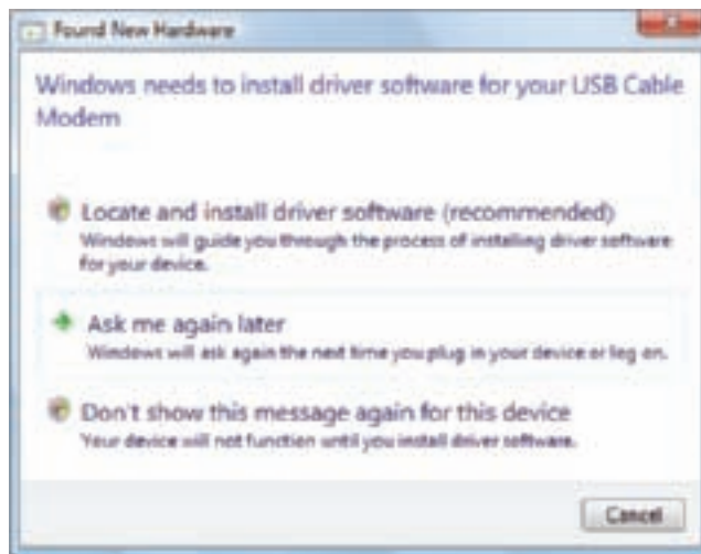
Figure 18-5 When using a USB cable to connect to the cable modem, the Found New Hardware Wizard will install the cable modem drivers Courtesy: Course Technology/Cengage Learning
