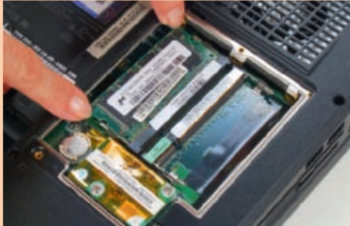
Figure 21-50 Push down on the SO-DIMM until it pops into the clips Courtesy: Course Technology/Cengage Learning
