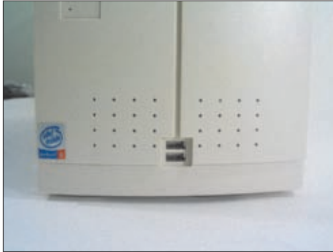
Figure 9-4 One or more USB ports on the front of a computer case make for easy access Courtesy: Course Technology/Cengage Learning
