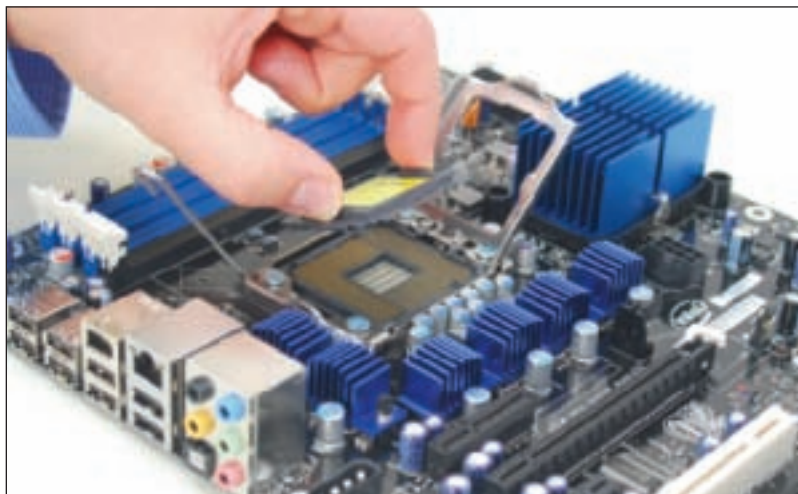
Figure 6-22 Remove the socket protective cover Courtesy: Course Technology/Cengage Learning
