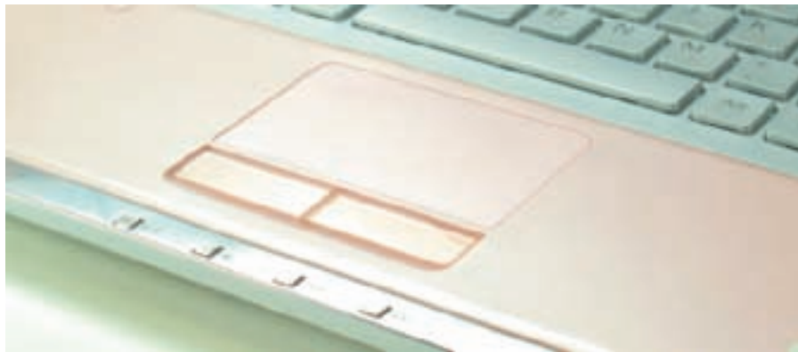
Figure 21-37 The touch pad is the most common pointing device on a notebook Courtesy: Course Technology/Cengage Learning
