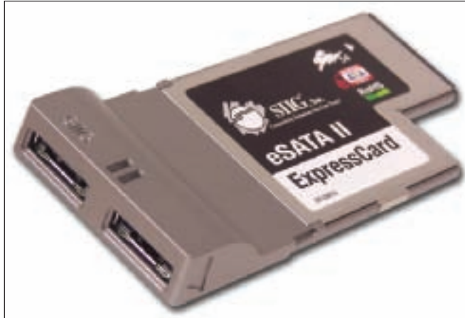
Figure 21-20 This ExpressCard/54 card supports two eSATA drives Courtesy of SIIG, Inc.
