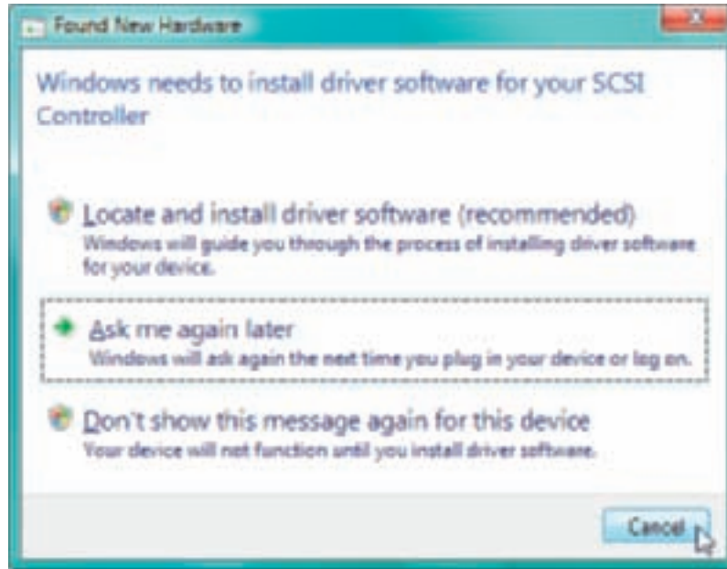
Figure 9-81 Vista wants to install drivers for the device it just found Courtesy: Course Technology/Cengage Learning
