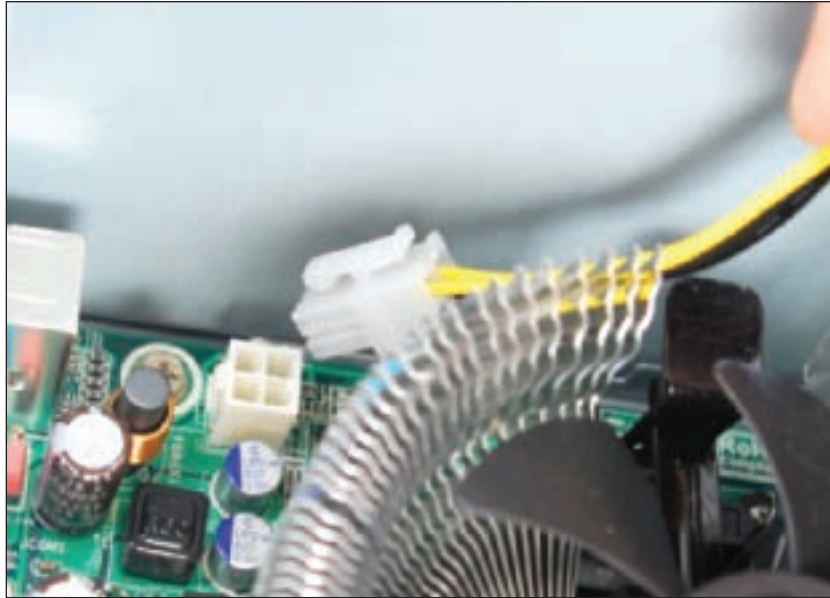
Figure 5-50 The auxiliary 4-pin power cord provides power to the processor Courtesy: Course Technology/Cengage Learning
