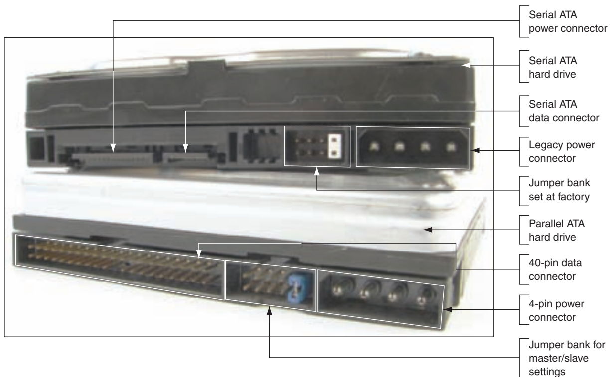
Figure 8-20 Rear of a serial ATA drive and a parallel ATA drive Courtesy: Course Technology/Cengage Learning
