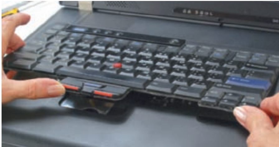
Figure 21-63 Pry up and lift the keyboard out of the notebook case Courtesy: Course Technology/Cengage Learning
