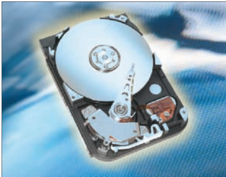
Figure 1-15 Hard drive with sealed cover removed Courtesy: Seagate Technologies LLC
