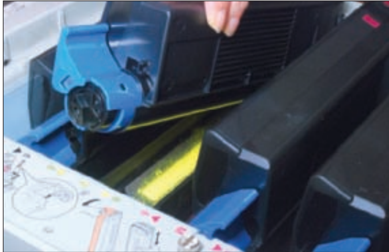
Figure 22-40 Remove the toner cartridge Courtesy: Course Technology/Cengage Learning
