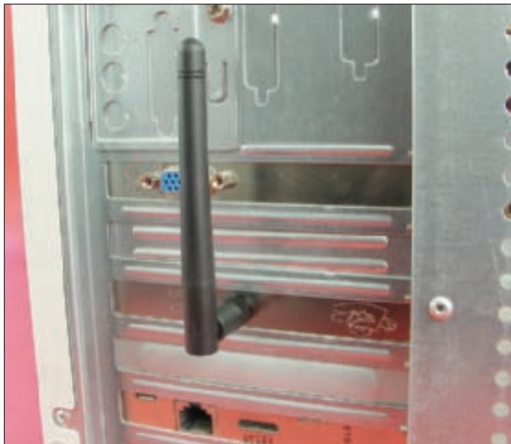
Figure 17-62 Raise the antenna on a NIC to an upright position Courtesy: Course Technology/Cengage Learning
