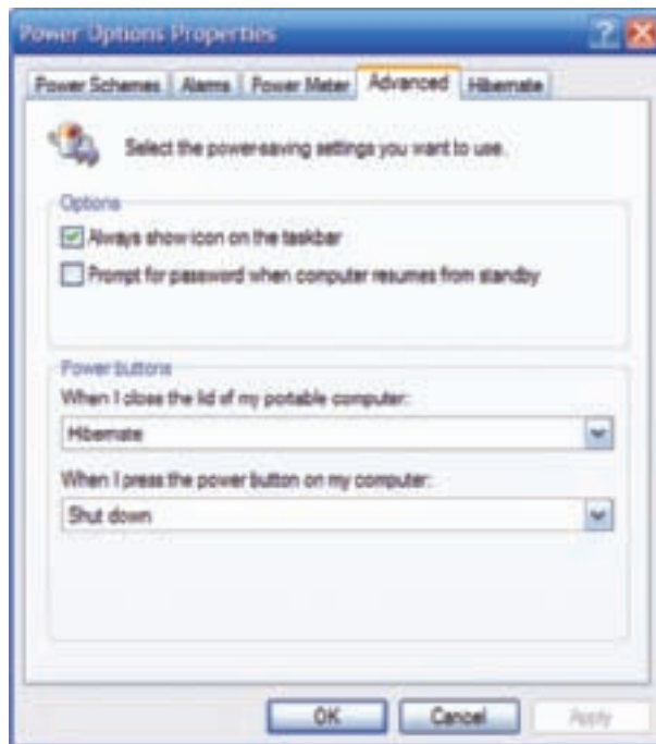
Figure 21-35 The Advanced tab of the Power Options Properties dialog box allows you to control the behavior of the power button and what happens when you close the lid of your notebook Courtesy: Course Technology/Cengage Learning
