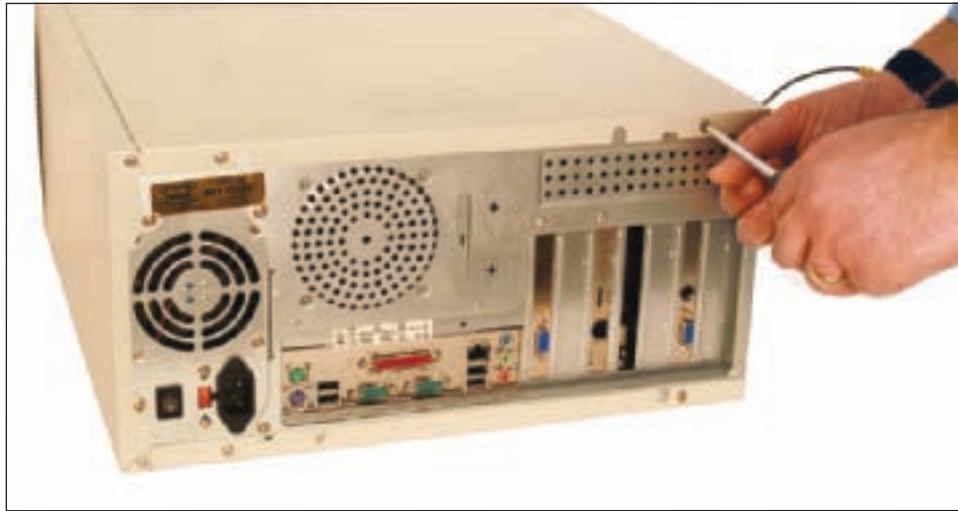
Figure 4-36 Locate the screws that hold the top cover in place Courtesy: Course Technology/Cengage Learning
