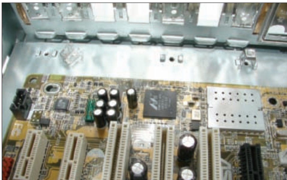
Figure 4-51 This motherboard connects to a case using screws and spacers that keep the board from touching the case Courtesy: Course Technology/Cengage Learning
