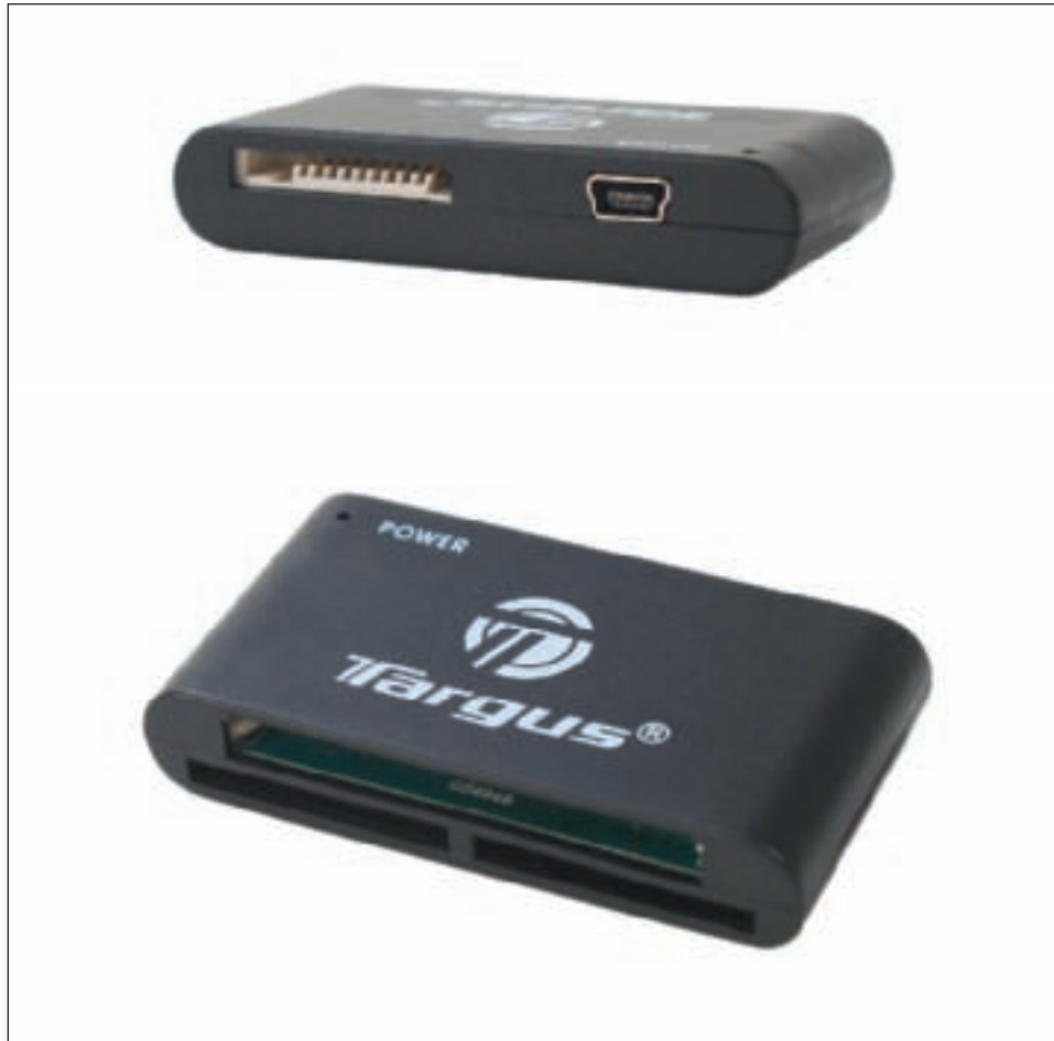
Figure 10-31 This Hi-Speed USB card reader/writer by Targus can read CompactFlash I and II, MicroDrive, SDHC, SD, MMC, xD, Memory Stick, PRO Duo, and Mini SD cards Courtesy: Course Technology/Cengage Learning
