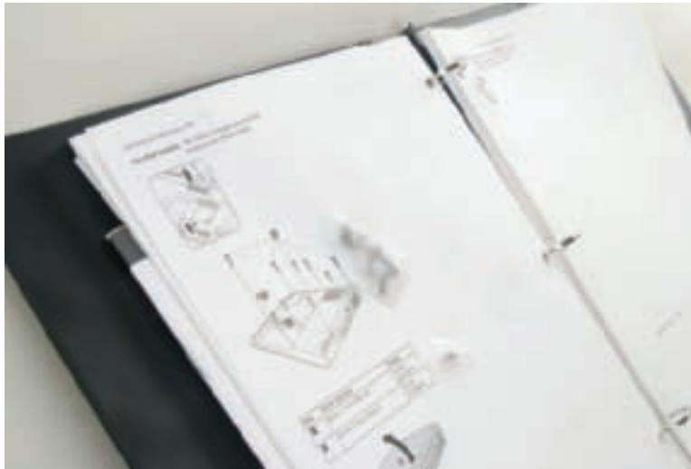
Figure 21-59 Tape screws beside the step in the manufacturer documentation that told you to remove the screw Courtesy: Course Technology/Cengage Learning
