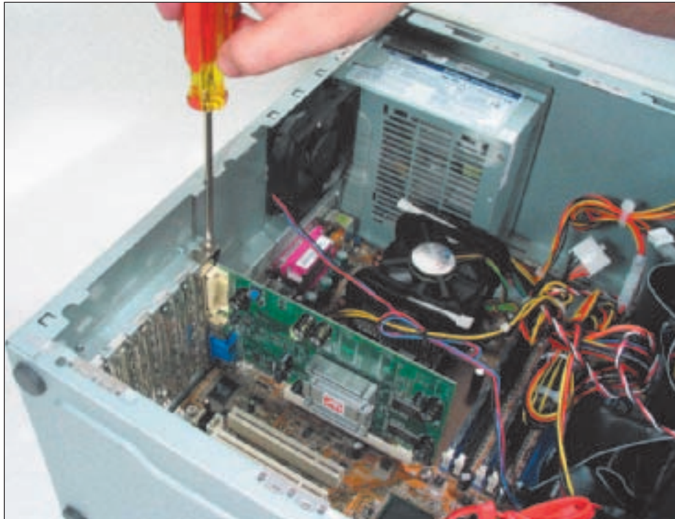
Figure 9-67 Secure the card to the case with a single screw Courtesy: Course Technology/Cengage Learning
