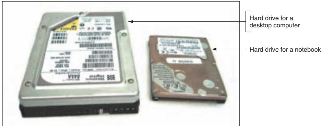
Figure 21-51 Hard drives for notebooks are smaller than hard drives for desktop computers Courtesy: Course Technology/Cengage Learning
