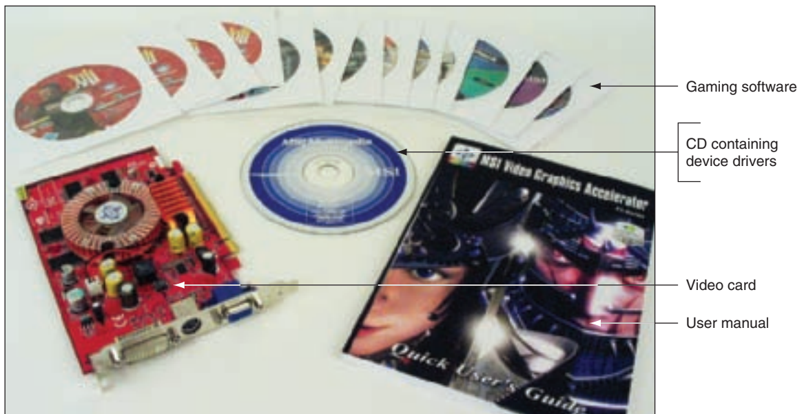
Figure 2-13 A device such as this video card comes packaged with its device drivers stored on a CD; alternately, you can use device drivers built into the OS Courtesy: Course Technology/Cengage Learning
