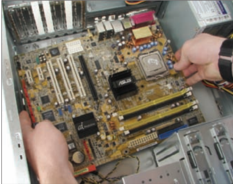
Figure 5-46 Place the motherboard in the case Courtesy: Course Technology/Cengage Learning
