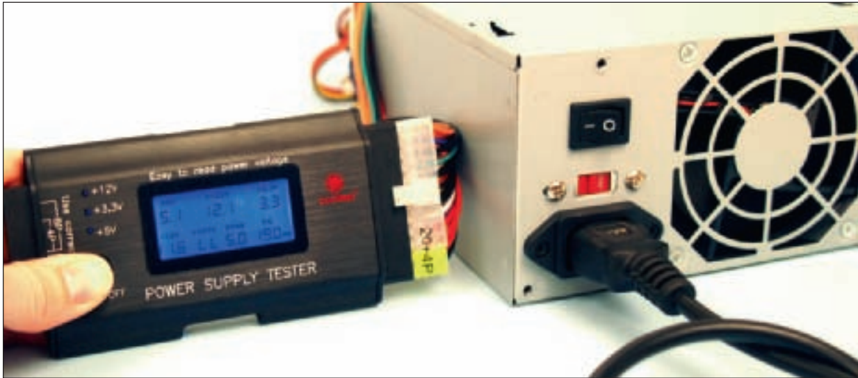
Figure 4-33 Use a power supply tester to test the output of each power connector on a power supply Courtesy: Course Technology/Cengage Learning
