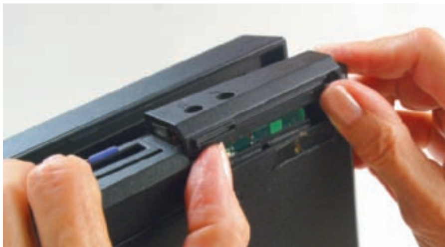
Figure 21-54 Push the drive out of its bay Courtesy: Course Technology/Cengage Learning
