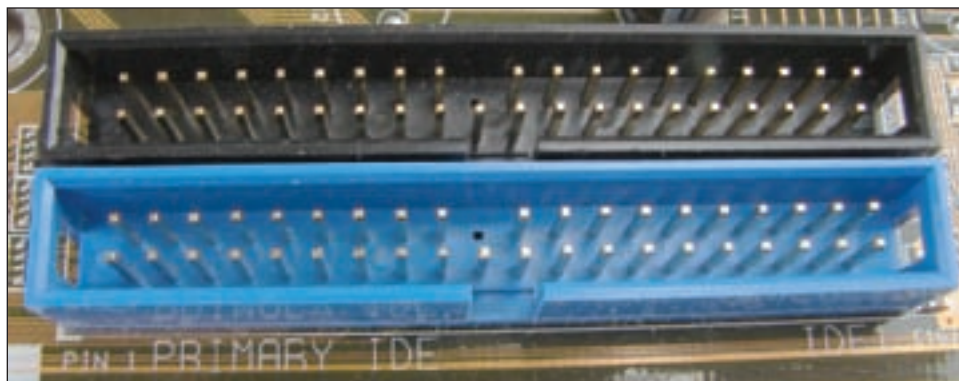
Figure 8-35 The primary IDE channel connector is often color-coded as blue Courtesy: Course Technology/Cengage Learning
