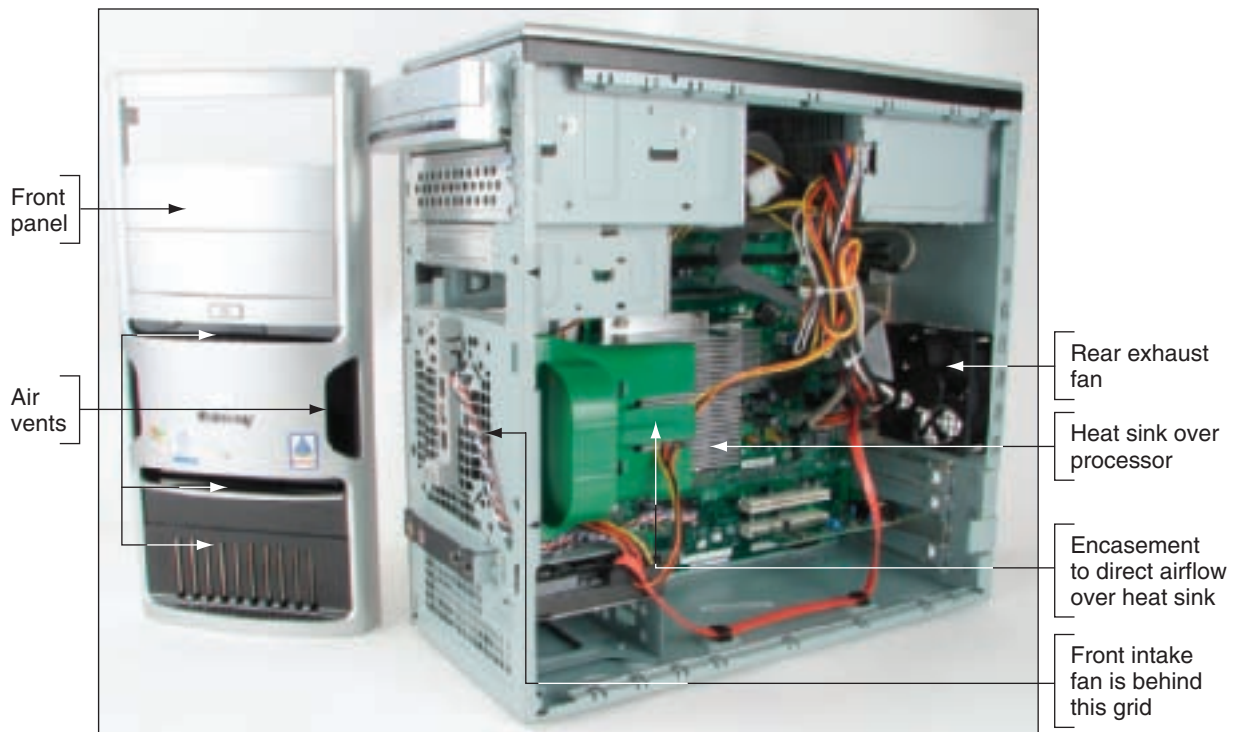
Figure 4-9 A Gateway BTX system is designed for optimum airflow Courtesy: Course Technology/Cengage Learning
