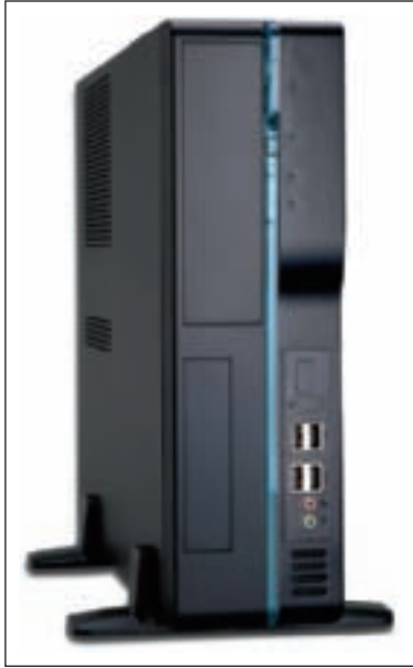
Figure 4-12 This slimline case by ENlight supports a MicroATX motherboard Courtesy of ENlight Corp
