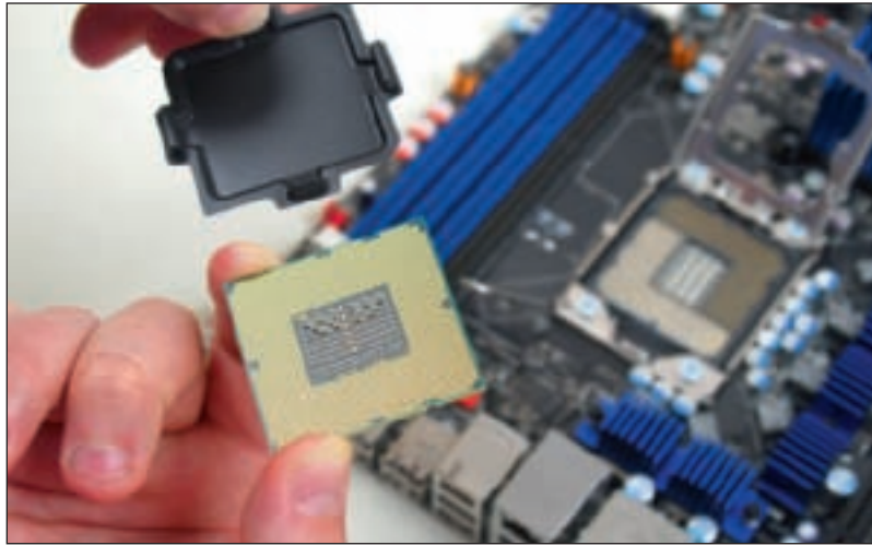
Figure 6-23 Remove the protective cover from the processor Courtesy: Course Technology/Cengage Learning
