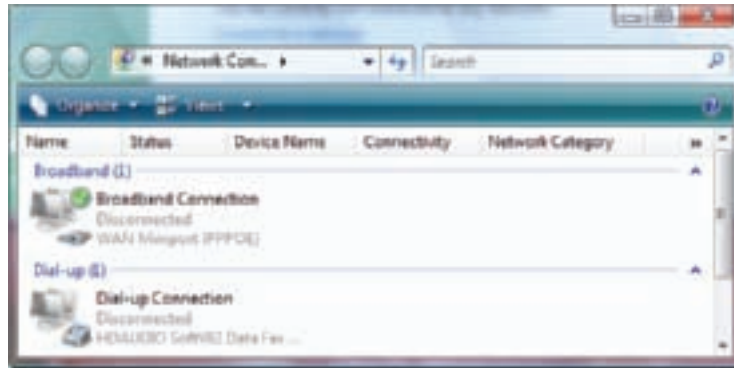
Figure 18-15 Use the Network Connections window to manage these connections Courtesy: Course Technology/Cengage Learning
