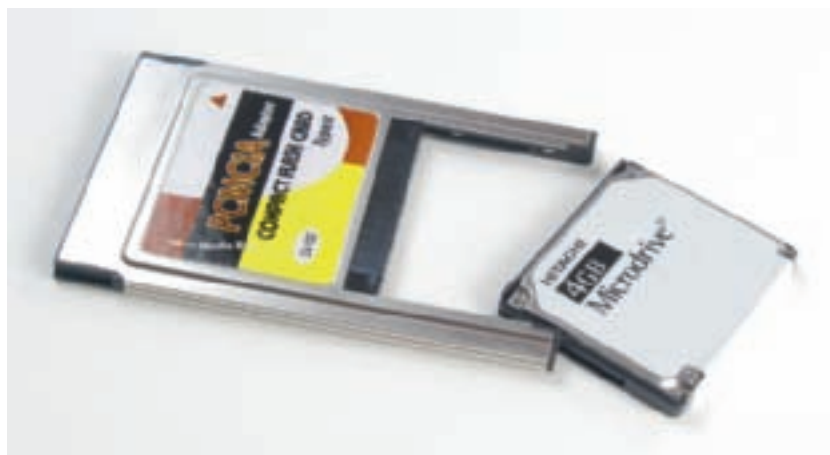
Figure 21-15 A Type II PC Card adapter for a Microdrive device Courtesy: Course Technology/Cengage Learning
