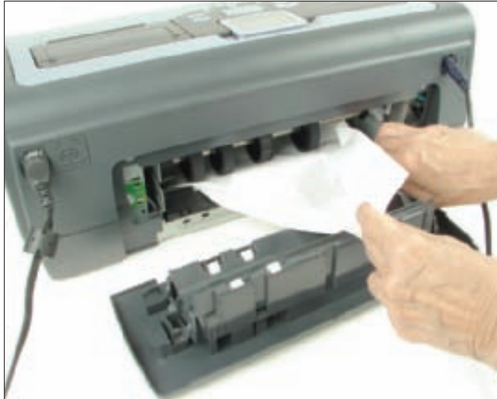
Figure 22-60 Open the door on the back of an inkjet printer to remove jammed paper Courtesy: Course Technology/Cengage Learning
