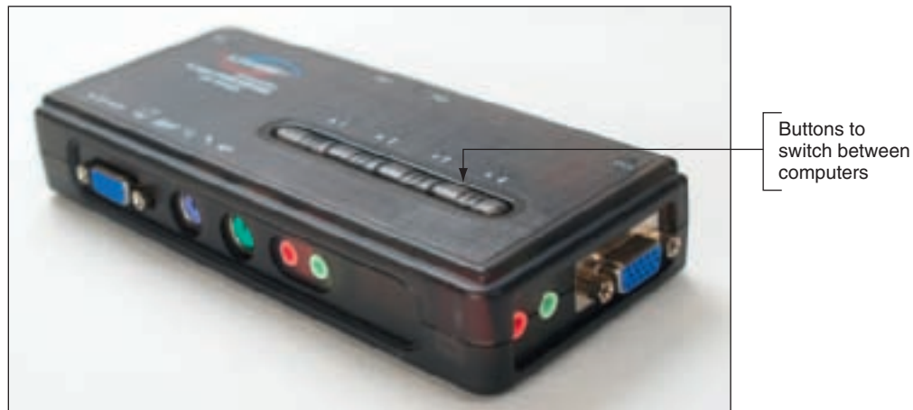
Figure 9-51 This KVM switch supports up to four computers, uses PS/2 ports for the keyboard and mouse, and provides microphone and speaker ports for sound Courtesy: Course Technology/Cengage Learning
