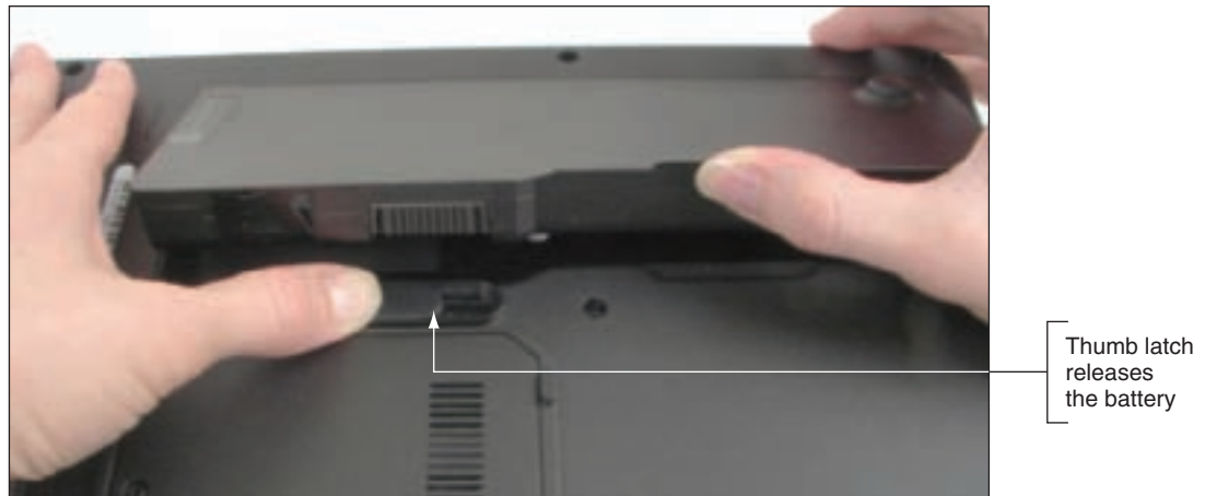
Figure 21-26 Release a latch to remove the battery from a notebook Courtesy: Course Technology/Cengage Learning
