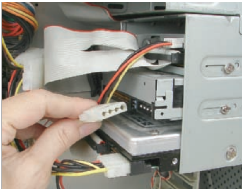
Figure 8-43 Connect a power cord to each drive Courtesy: Course Technology/Cengage Learning
