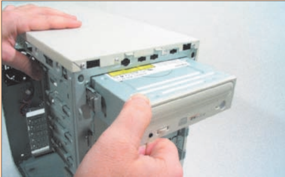
Figure 10-37 Slide the optical drive into the bay Courtesy: Course Technology/Cengage Learning
