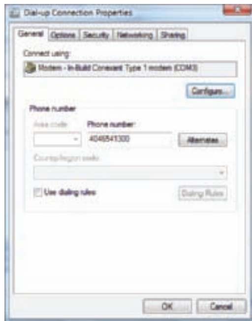
Figure 18-19 Configure an Internet connection using the Properties window of the connection icon Courtesy: Course Technology/Cengage Learning
