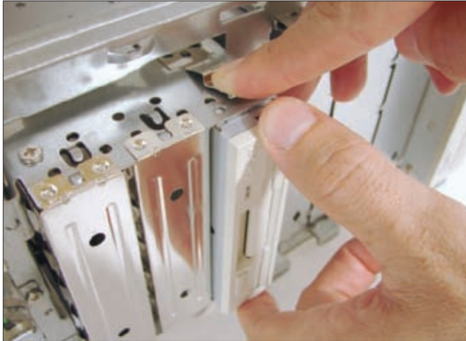
Figure 4-55 Push down on the clip and then slide the removable bay forward and out of the case Courtesy: Course Technology/Cengage Learning
