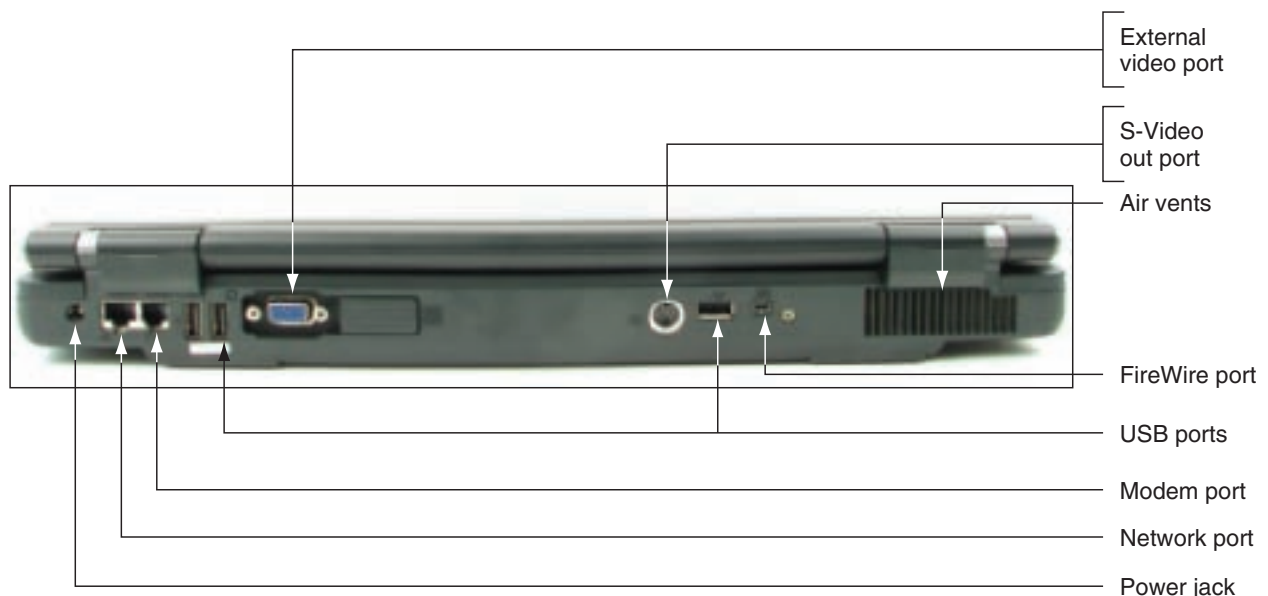
Figure 21-8 Ports on the back of a notebook Courtesy: Course Technology/Cengage Learning
