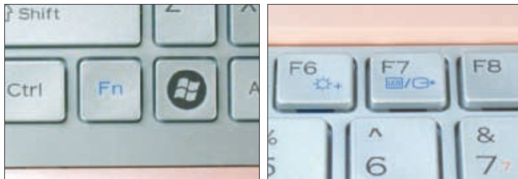
Figure 21-43 Use the Fn key and the F7 key to toggle between display devices Courtesy: Course Technology/Cengage Learning
