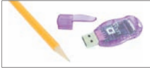
Figure 1-23 This flash drive, called the JumpDrive by Lexar, snaps into a USB port Courtesy: Course Technology/Cengage Learning
