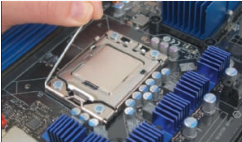
Figure 6-26 Return the lever to its locked position Courtesy: Course Technology/Cengage Learning
