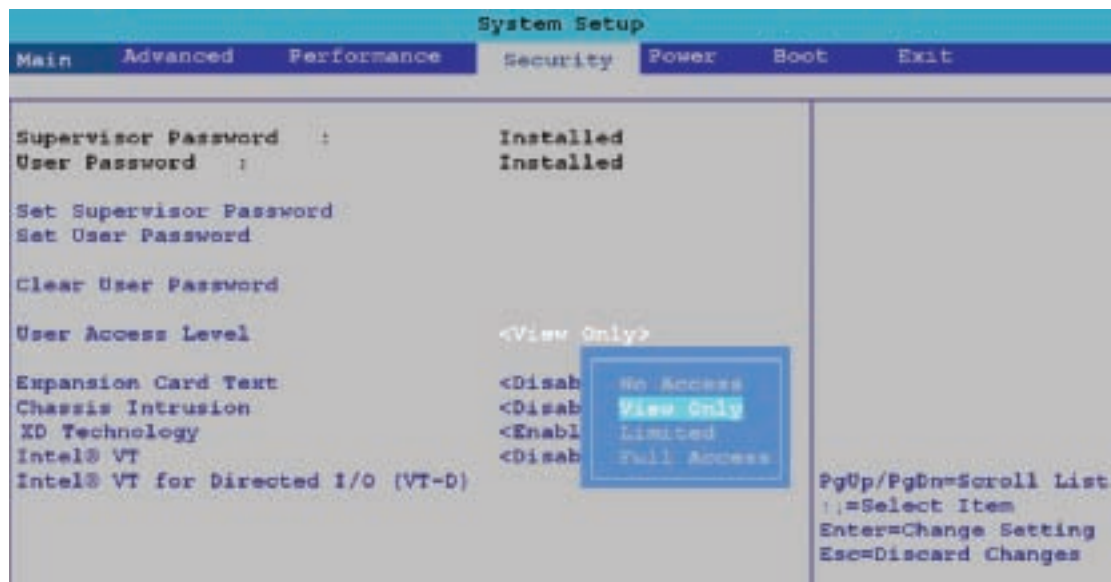
Figure 19-9 Set supervisor and user passwords in BIOS setup to lock down a computer Courtesy: Course Technology/Cengage Learning
