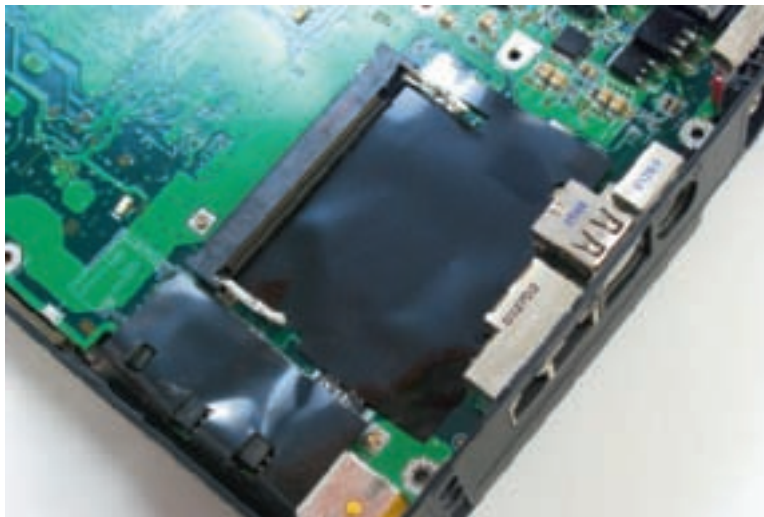
Figure 21-68 A Mini PCI slot follows PCI standards applied to notebooks Courtesy: Course Technology/Cengage Learning
