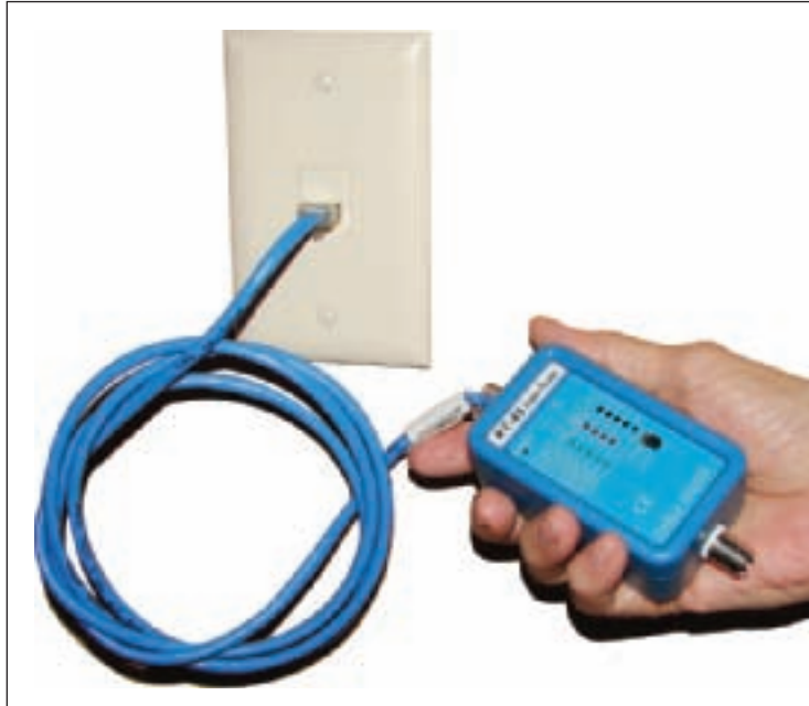
Figure 18-48 Use cable testers to trace network cables through a building Courtesy: Course Technology/Cengage Learning
