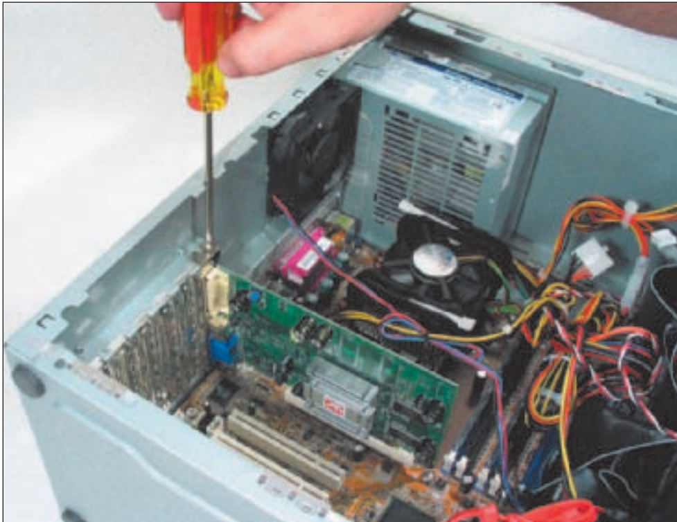
Figure 4-47 Remove the screw holding an expansion card to the case Courtesy: Course Technology/Cengage Learning
