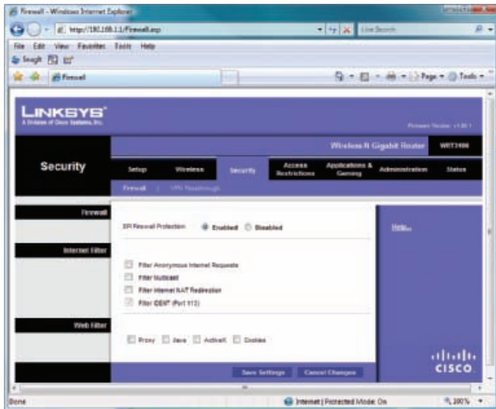
Figure 18-35 Configure the router's firewall to prevent others on the Internet from seeing or accessing your network Courtesy: Course Technology/Cengage Learning
