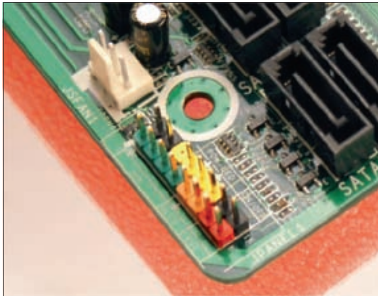
Figure 5-53 Front panel header uses color-coded pins Courtesy: Course Technology/Cengage Learning
