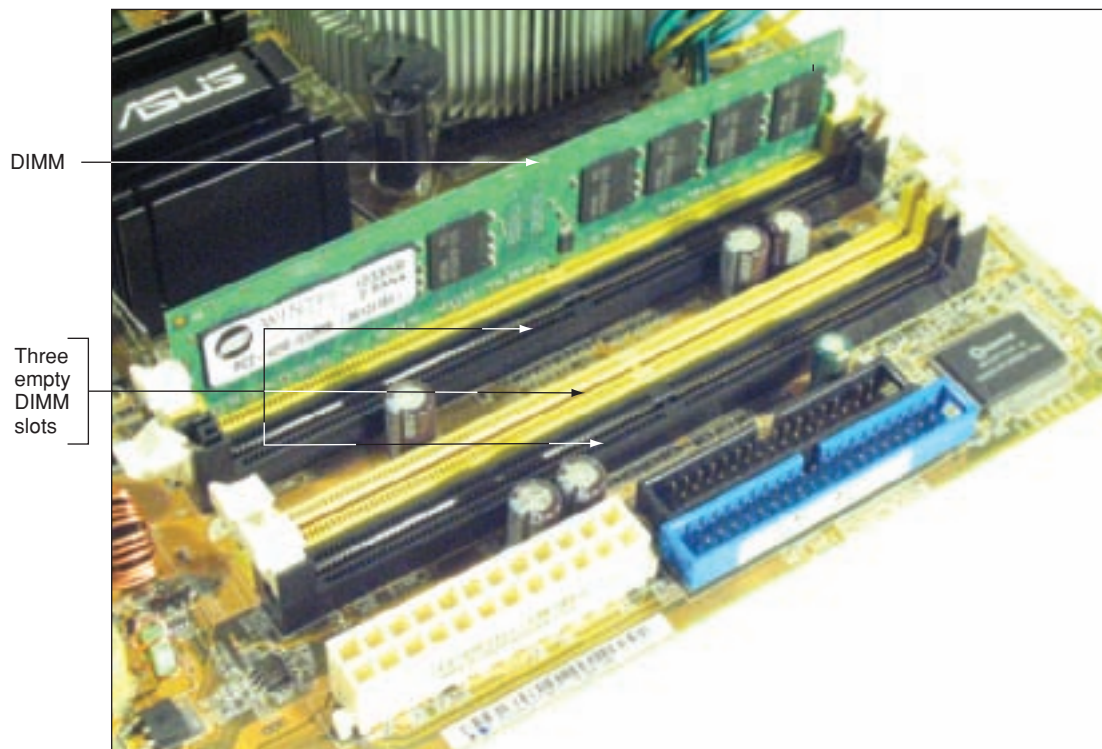
Figure 1-13 A DIMM holds RAM and is mounted directly on a motherboard Courtesy: Course Technology/Cengage Learning
