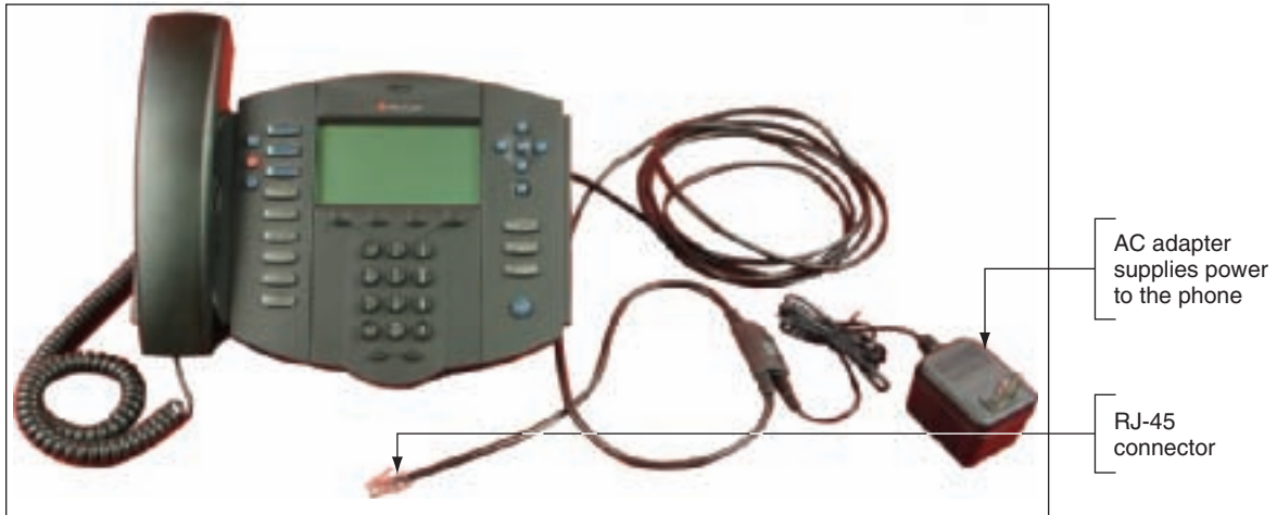
Figure 18-75 This digital telephone has a network port to connect to a network Courtesy: Course Technology/Cengage Learning
