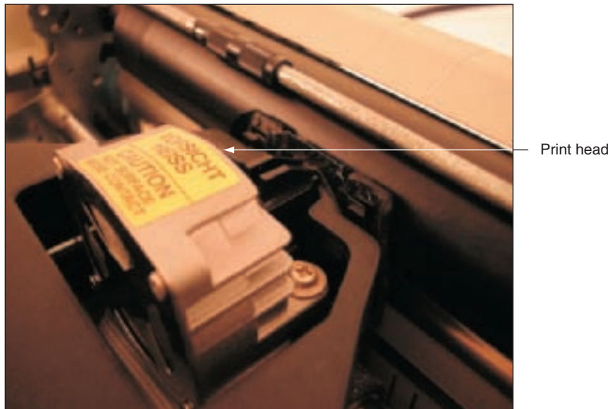
Figure 22-5 Keep the print head of a dot matrix printer as cool as possible so that it will last longer Courtesy: Course Technology/Cengage Learning
