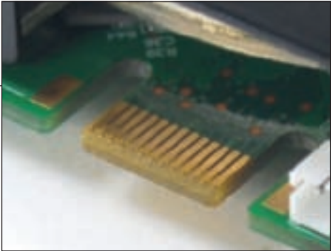
Figure 9-37 This video card is SLI compliant and can be installed with a second matching video card in a system Courtesy: Course Technology/Cengage Learning
