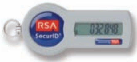
Figure 19-13 A smart card such as this SecurID key fob is used to authenticate a user gaining access to a secured network Courtesy of RSA Security
