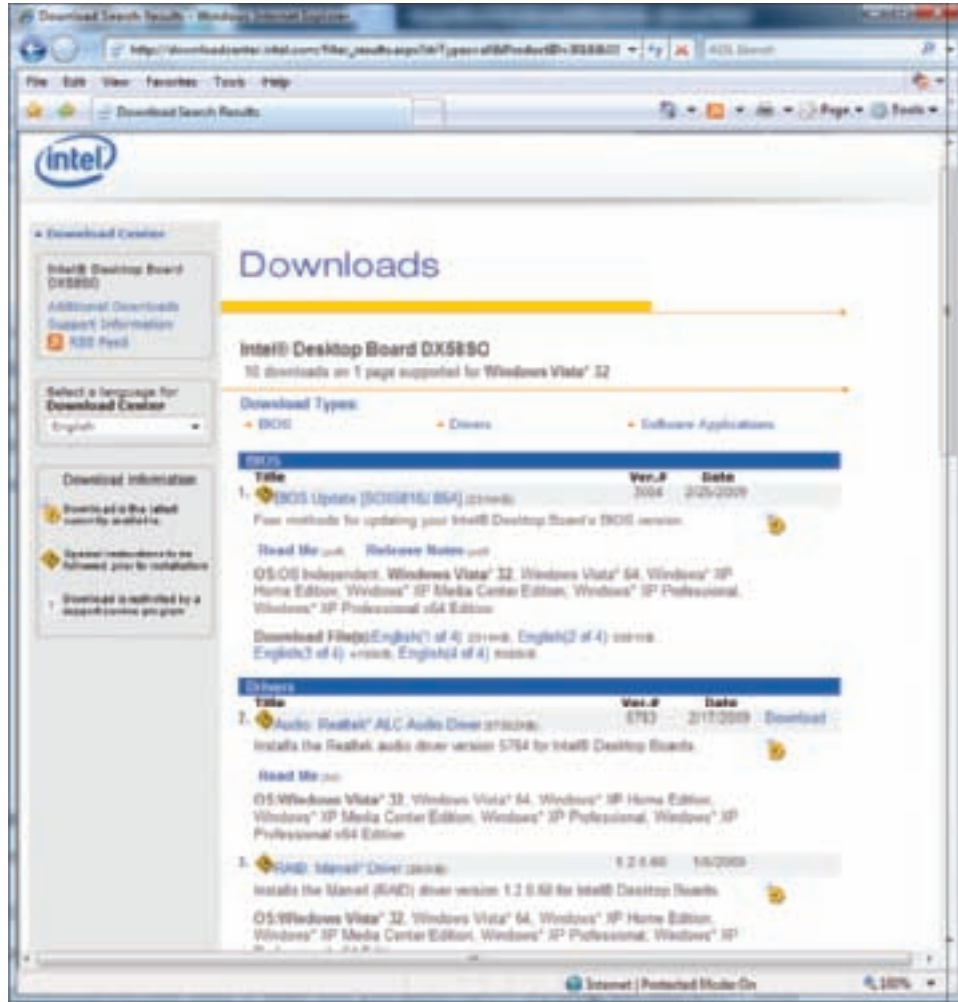
Figure 5-38 Download BIOS and driver updates from the motherboard Web site Courtesy: Course Technology/Cengage Learning
