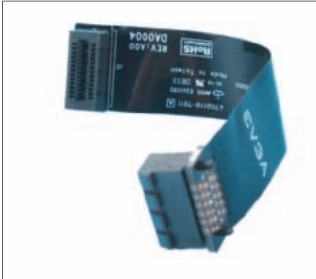
Figure 9-38 SLI bridge connects two SLI video cards Courtesy: Course Technology/Cengage Learning
