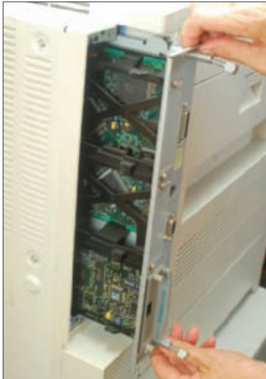
Figure 22-45 Remove the formatter board from the printer Courtesy: Course Technology/Cengage Learning
