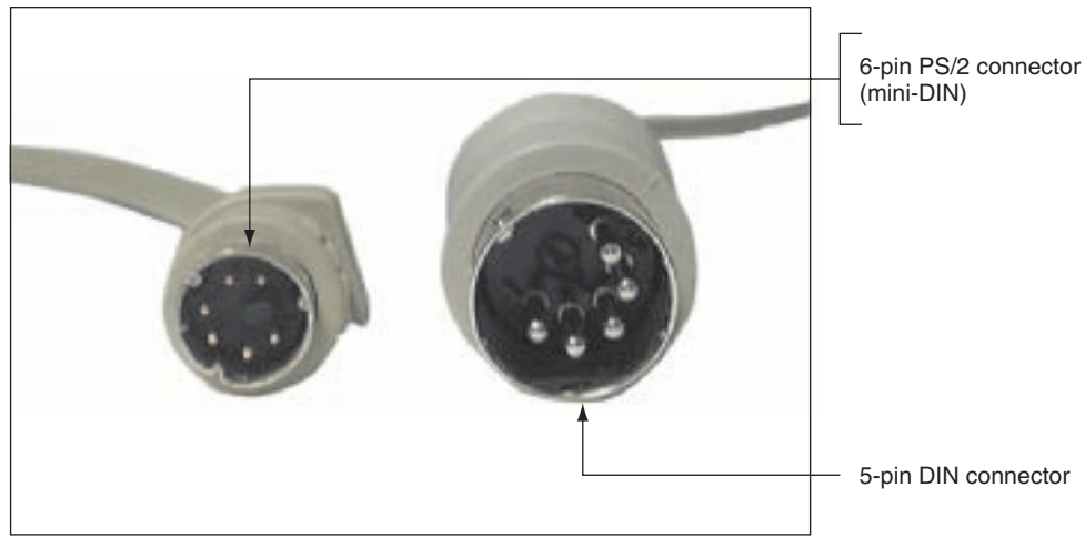
Figure 9-40 Two PS/2 and DIN connectors used by keyboards and mice Courtesy: Course Technology/Cengage Learning
