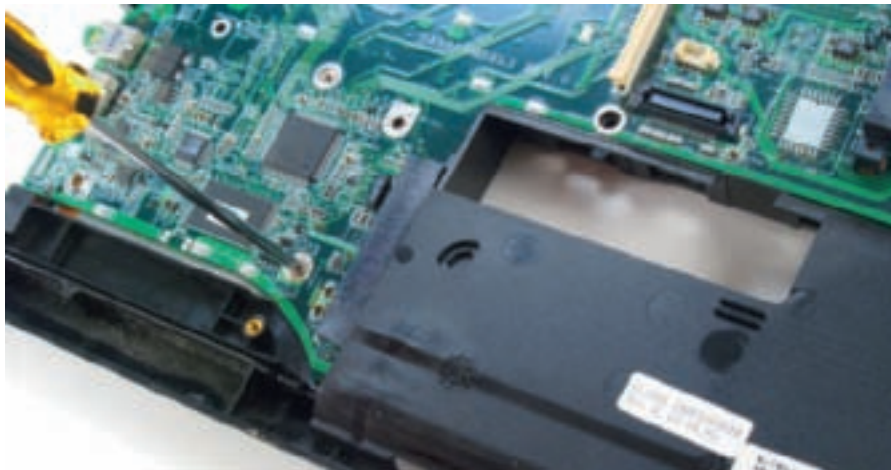
Figure 21-82 Remove the single screw attaching the motherboard to the case Courtesy: Course Technology/Cengage Learning
