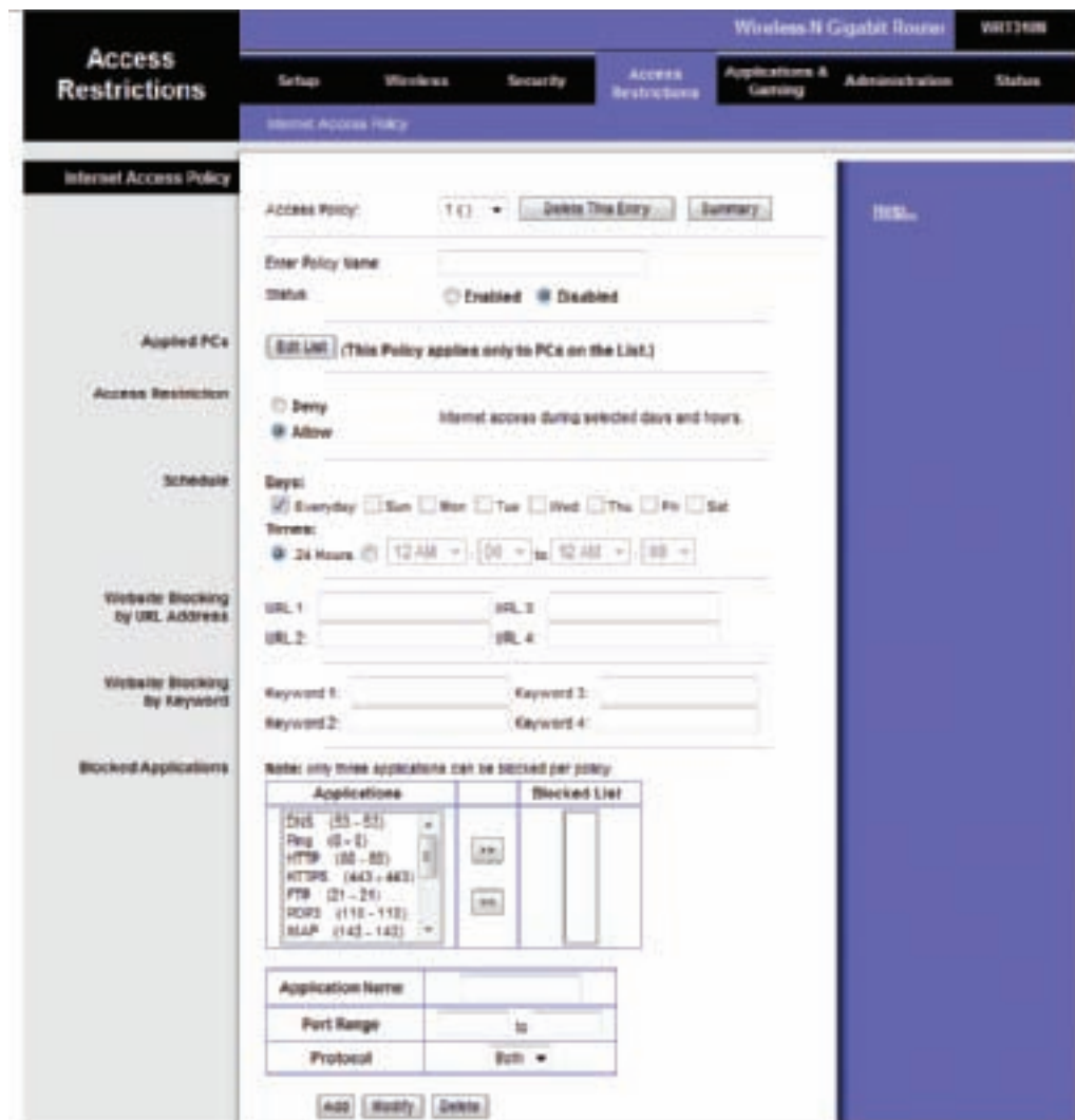
Figure 18-36 Configure the router's firewall to limit Internet access from within the network Courtesy: Course Technology/Cengage Learning
