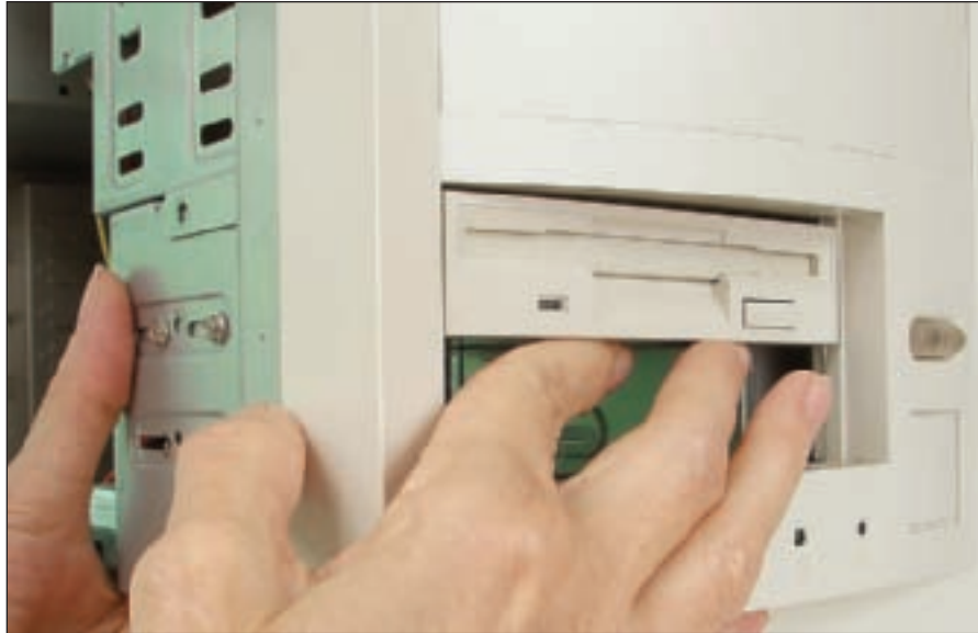
Figure 8-38 Line up the floppy drive in the removable bay so it's flush with the front of the case Courtesy: Course Technology/Cengage Learning
