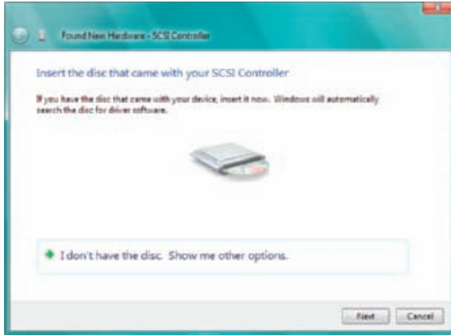
Figure 9-82 Insert the drive CD to continue the installation Courtesy: Course Technology/Cengage Learning
