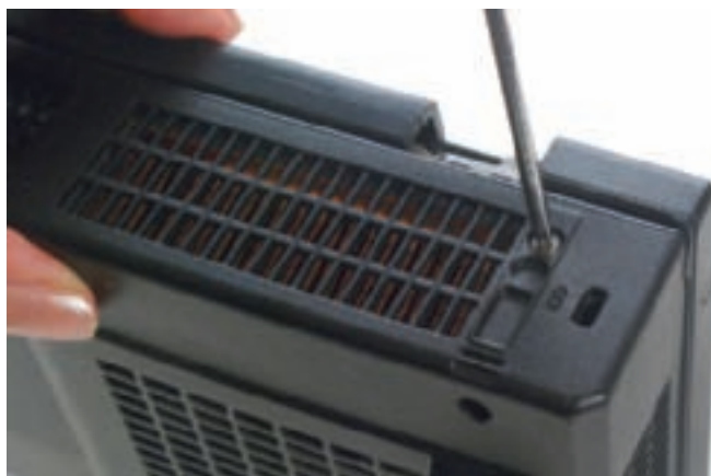
Figure 21-73 Remove two screws on the back of the notebook Courtesy: Course Technology/Cengage Learning
