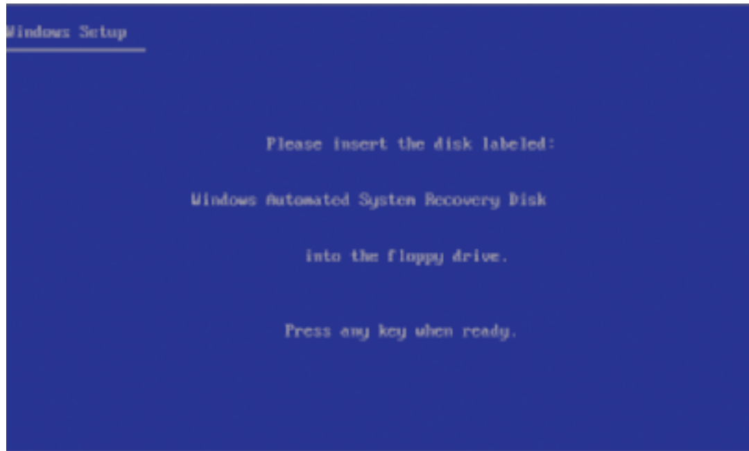
Figure 13-40 Automatic System Recovery process must have the ASR floppy disk Courtesy: Course Technology/Cengage Learning
