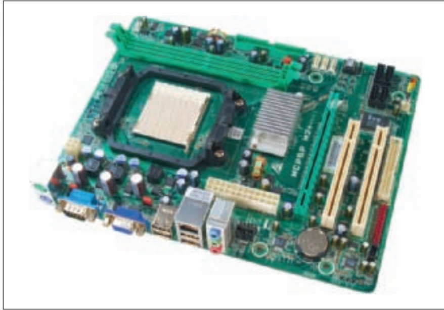
Figure 4-7 This MicroATX motherboard by Biostar is designed to support an AMD processor Courtesy: Course Technology/Cengage Learning
