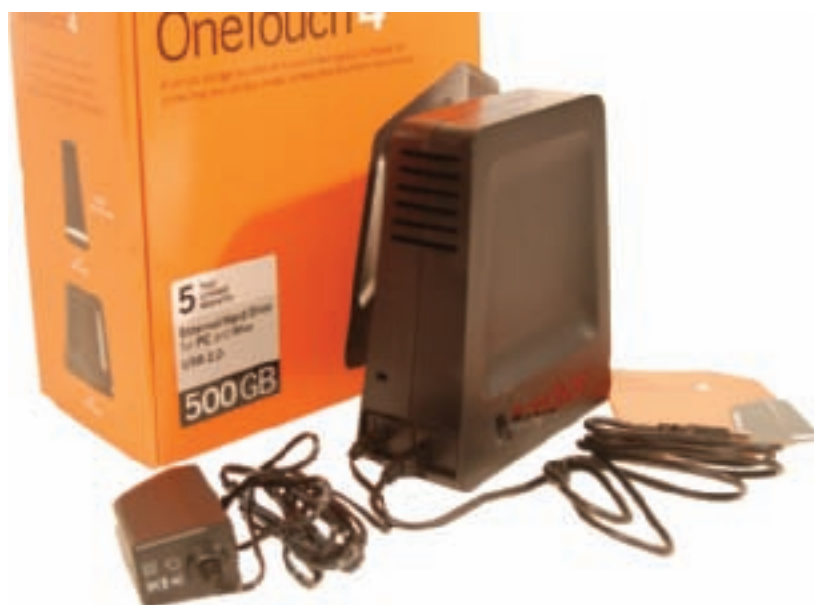
Figure 13-19 This external hard drive by Maxtor uses a USB port and comes bundled with backup software Courtesy: Course Technology/Cengage Learning
