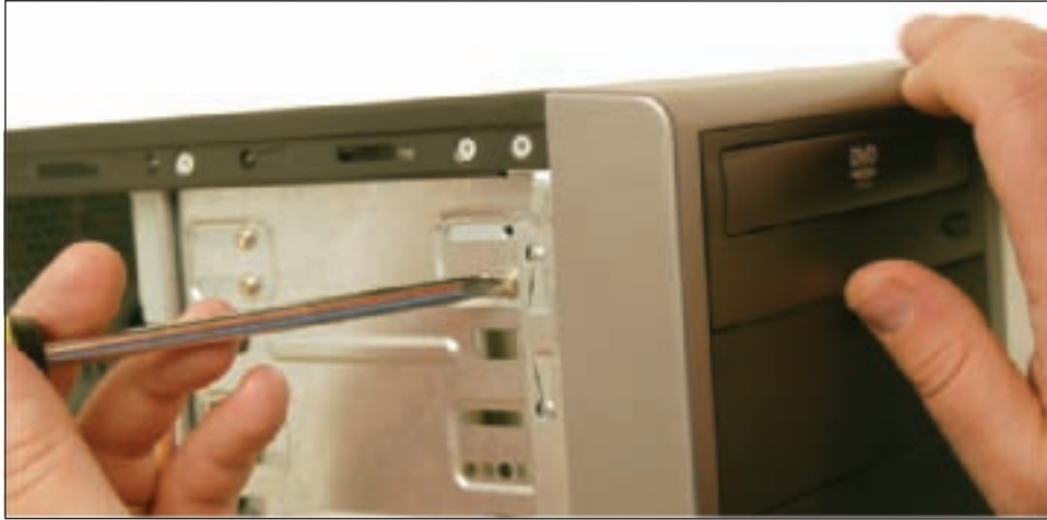
Figure 4-57 Align the front of the drive flush with the case front and then anchor with a screw Courtesy: Course Technology/Cengage Learning
