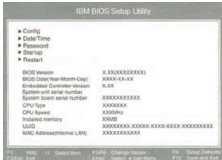
Figure 5-64 BIOS setup main menu for an IBM computer Courtesy: Course Technology/Cengage Learning
