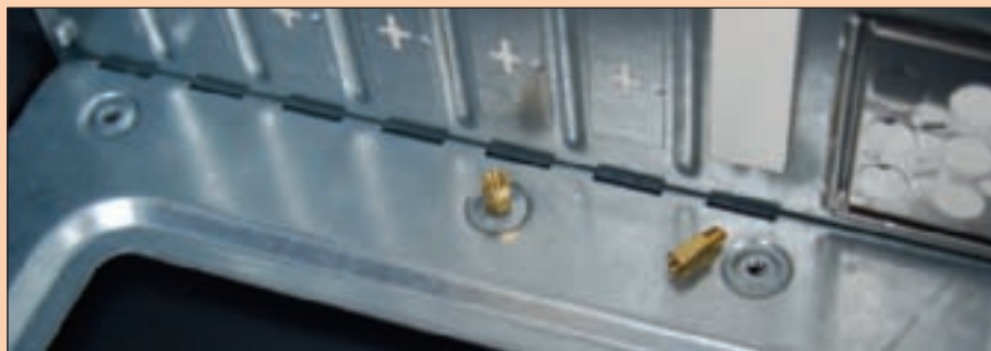
Figure 6-50 Spacers installed in case holes keep the motherboard from causing a short Courtesy: Course Technology/Cengage Learning
