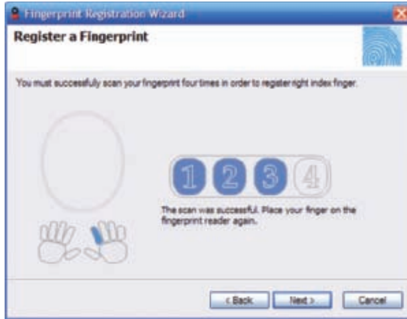
Figure 9-50 A fingerprint is registered after it is recorded four times Courtesy: Course Technology/Cengage Learning
