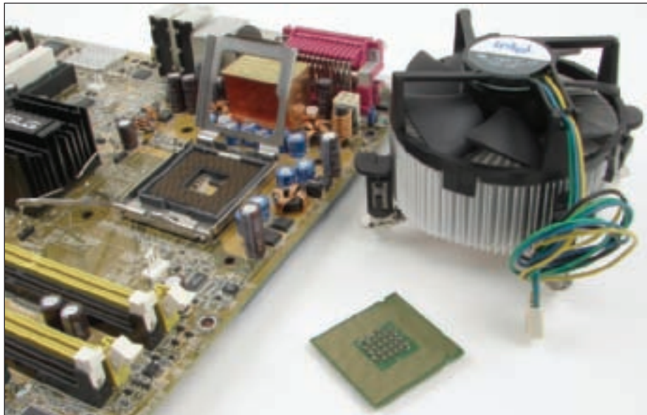
Figure 6-34 A Pentium, cooler, and open socket 775 Courtesy: Course Technology/Cengage Learning
