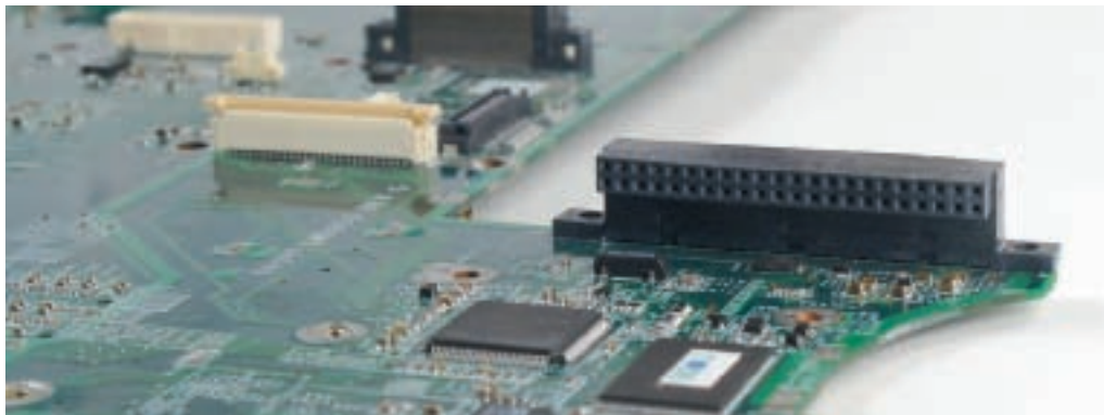
Figure 21-52 A 44-pin IDE connector on a notebook motherboard Courtesy: Course Technology/Cengage Learning
