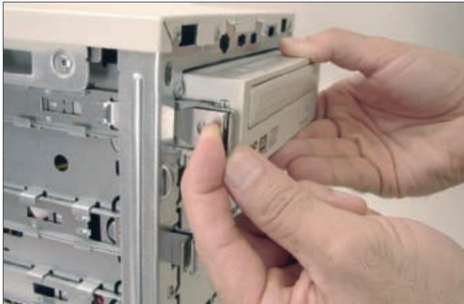
Figure 4-54 To remove this CD drive, first pull the clip forward to release the drive from the bay Courtesy: Course Technology/Cengage Learning
