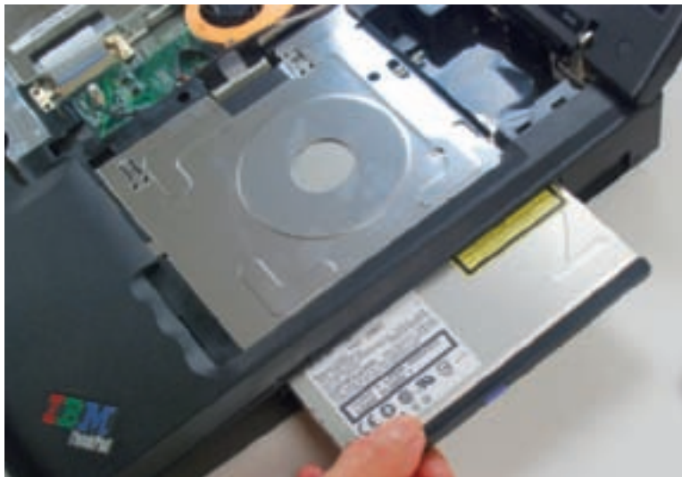
Figure 21-66 Slide the drive out of the bay Courtesy: Course Technology/Cengage Learning
