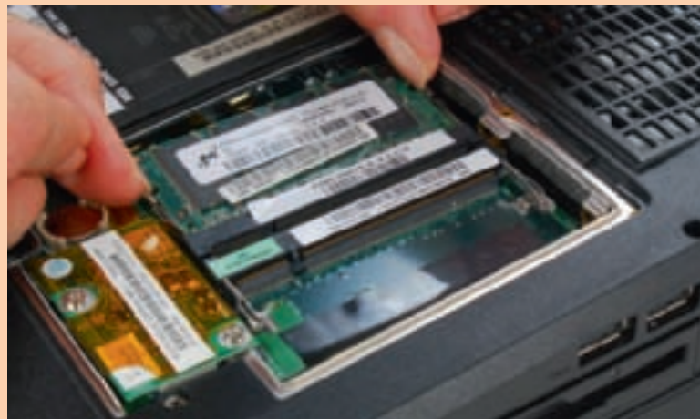
Figure 21-48 Pull apart the clips on the memory slot to release the SO-DIMM Courtesy: Course Technology/Cengage Learning
