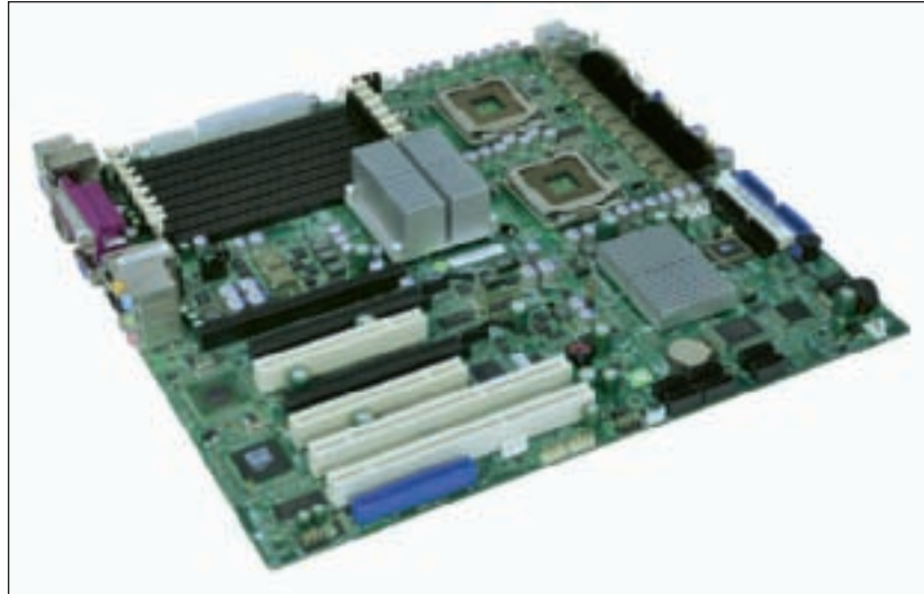
Figure 5-13 The two long green PCI-X slots can support PCI cards Courtesy of Super Micro Computer Inc.
