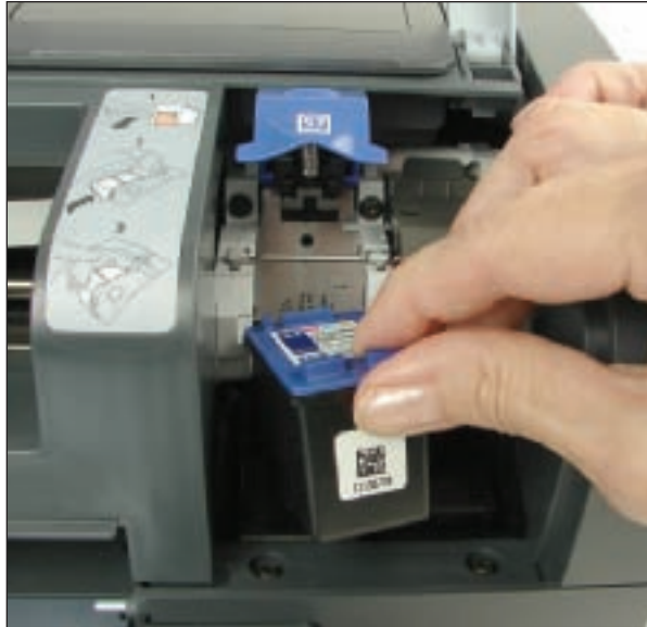
Figure 22-33 Installing an ink cartridge in an inkjet printer Courtesy: Course Technology/Cengage Learning
