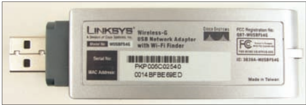
Figure 17-70 The MAC address is printed on the back of this USB wireless adapter Courtesy: Course Technology/Cengage Learning
