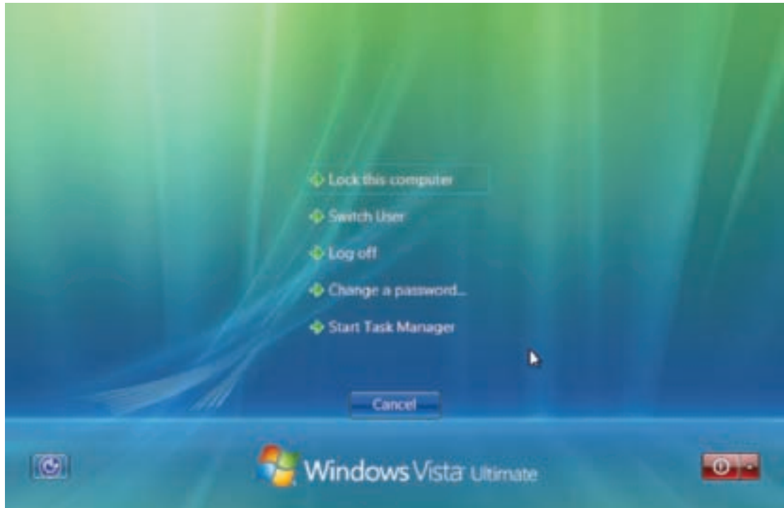
Figure 19-31 Results of pressing Ctrl-Alt-Del when a user is already logged on Courtesy: Course Technology/Cengage Learning
