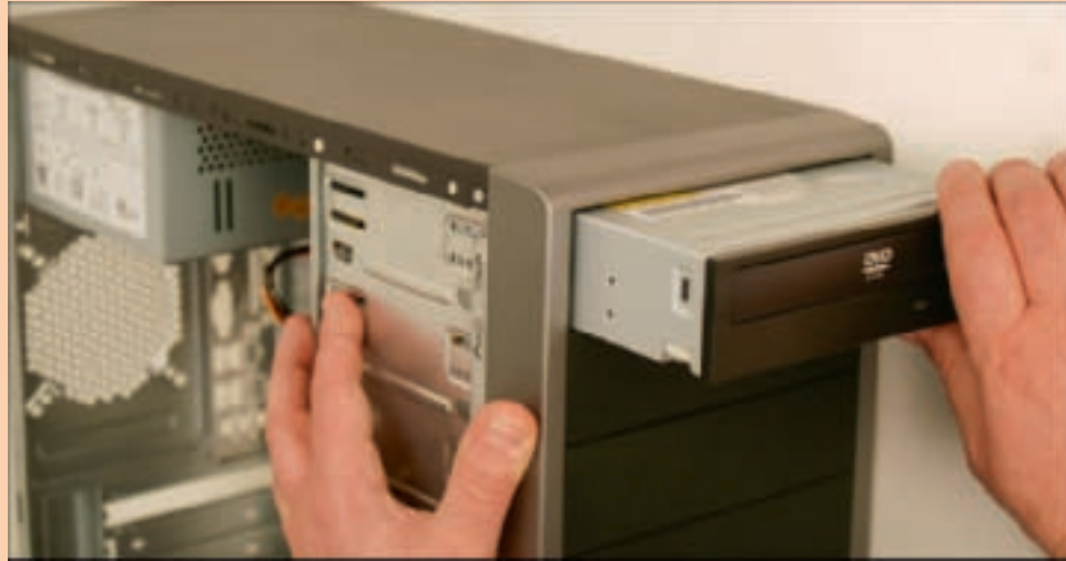
Figure 10-39 Slide the drive into the bay flush with the front panel Courtesy: Course Technology/Cengage Learning
