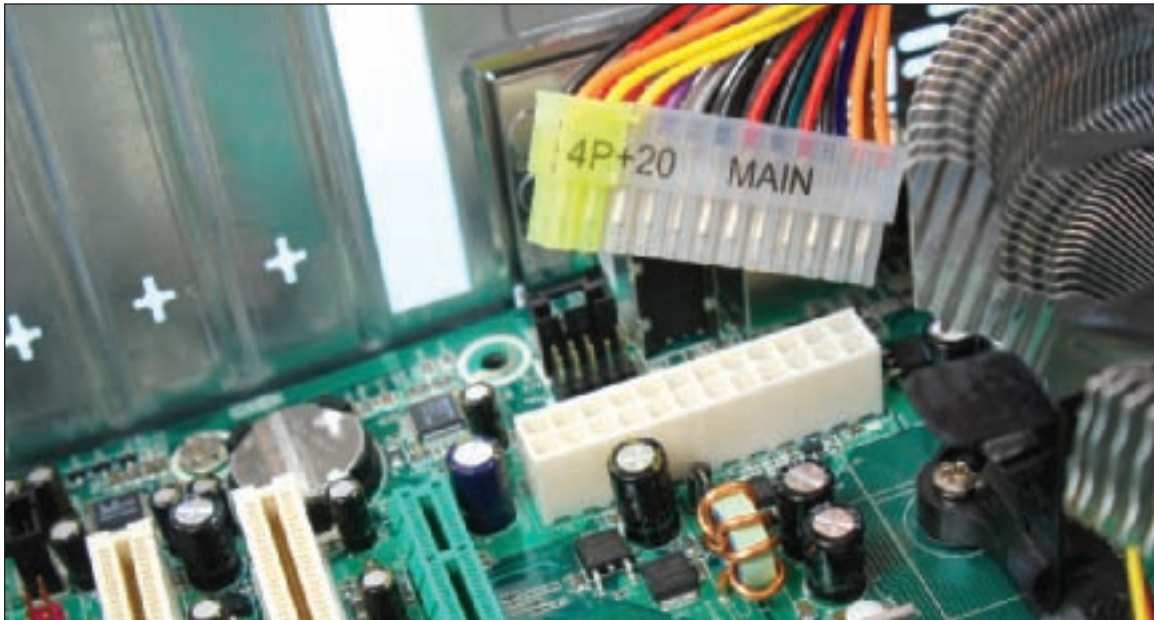
Figure 5-49 The 24-pin connector supplies power to the motherboard Courtesy: Course Technology/Cengage Learning
