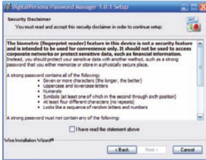
Figure 9-48 The setup program for this fingerprint reader warns to not rely on the reader to protect sensitive data Courtesy: Course Technology/Cengage Learning
