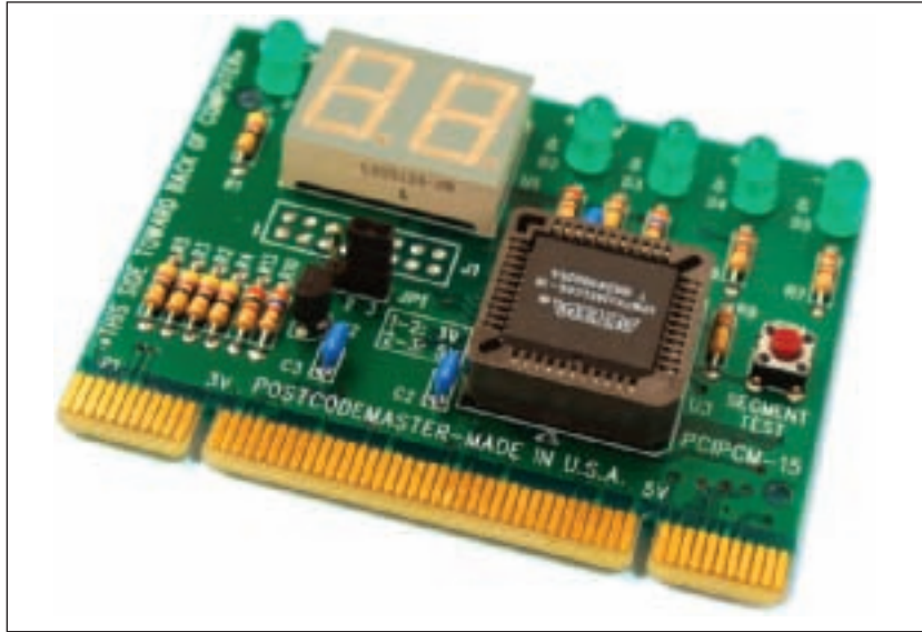
Figure 4-32 Post Code Master diagnostic card by Microsystems Developments, Inc. Courtesy: Course Technology/Cengage Learning
