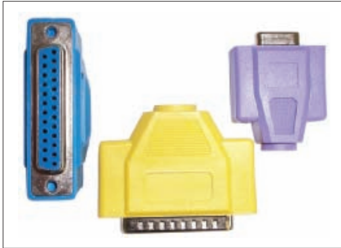
Figure 9-86 Loop-back plugs used to test serial and parallel ports Courtesy of Smith Micro Software, Inc.
