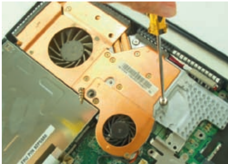
Figure 21-77 Remove the screws holding the CPU fan assembly in place Courtesy: Course Technology/Cengage Learning
