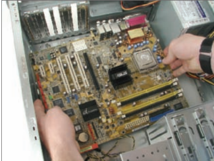
Figure 4-52 Remove the motherboard from the case Courtesy: Course Technology/Cengage Learning
