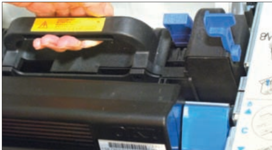
Figure 22-43 Remove the fuser Courtesy: Course Technology/Cengage Learning
