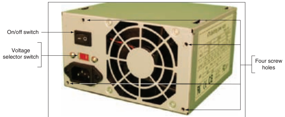
Figure 4-21 Holes in the rear of an ATX power supply match up with holes in the ATX case to anchor the power supply to the case Courtesy: Course Technology/Cengage Learning
