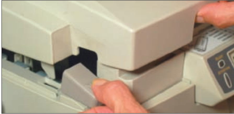
Figure 22-36 Open the printer cover Courtesy: Course Technology/Cengage Learning
