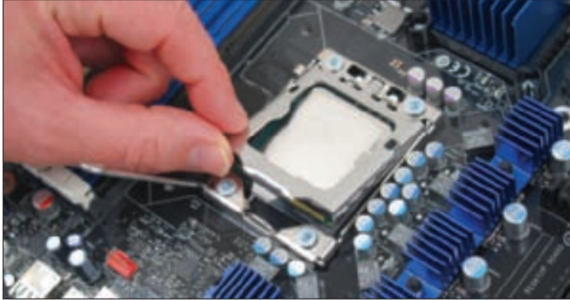
Figure 6-25 Close the socket load plate Courtesy: Course Technology/Cengage Learning
