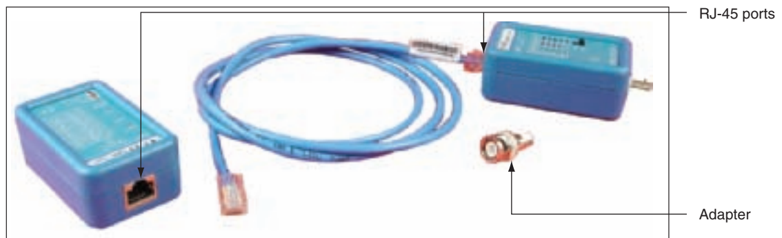
Figure 18-47 Use a cable tester pair to determine the type of cable and if the cable is good Courtesy: Course Technology/Cengage Learning
