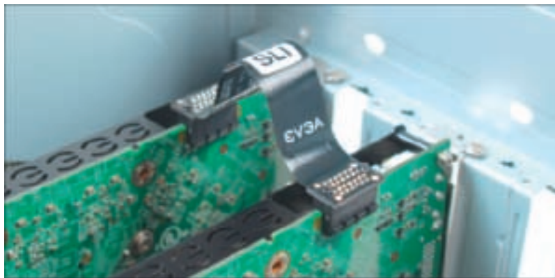
Figure 9-80 SLI bridge is used to improve communication between two SLI video cards Courtesy: Course Technology/Cengage Learning
