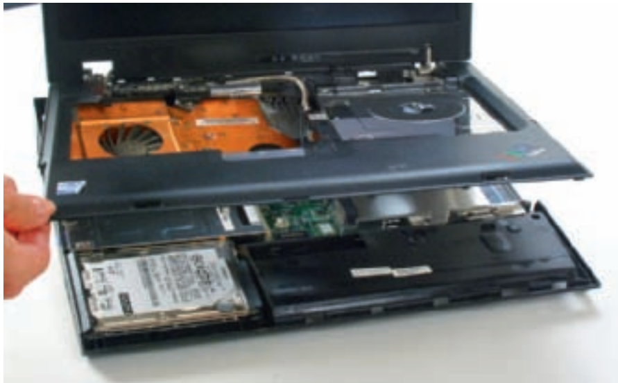
Figure 21-75 Lift the assembly to locate the two cable connections Courtesy: Course Technology/Cengage Learning
