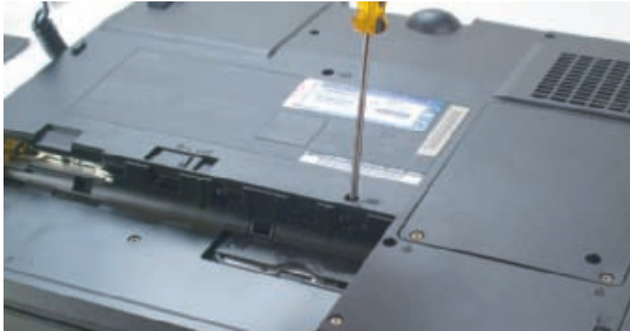
Figure 21-62 Remove screws on the bottom of the notebook Courtesy: Course Technology/Cengage Learning
