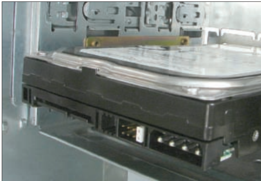
Figure 8-46 Hard drive installed in a wide bay using a universal bay kit adapter Courtesy: Course Technology/Cengage Learning
