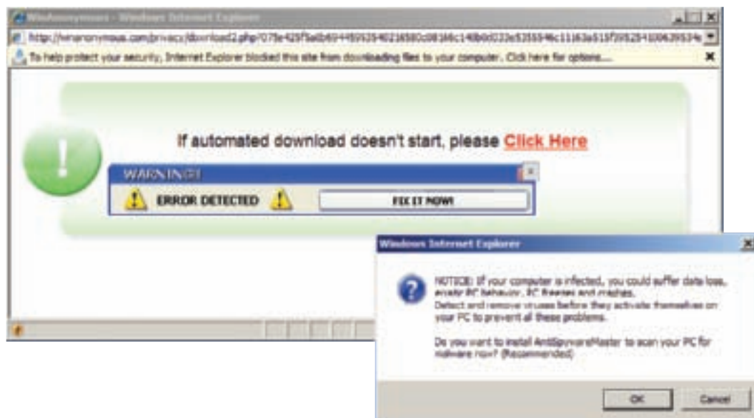
Figure 19-34 Clicking an action button on a pop-up window might invite a Trojan into your system Courtesy: Course Technology/Cengage Learning
