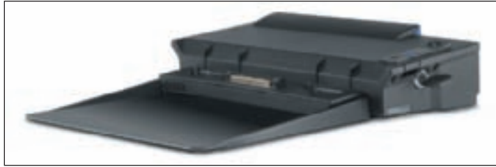
Figure 21-11 A docking station can provide extra secondary storage for a laptop Courtesy of IBM Corporation
