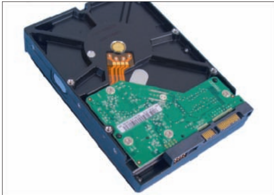
Figure 8-5 The bottom of a hard drive shows the circuit board that contains the firmware that controls the drive Courtesy: Course Technology/Cengage Learning
