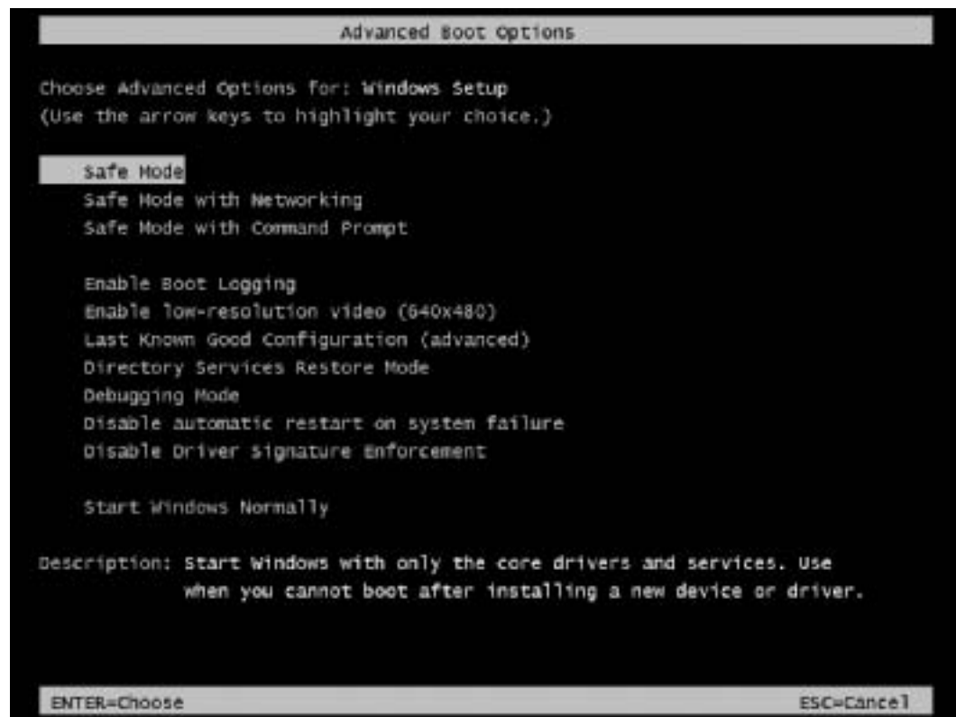
Figure 14-59 Windows Advanced Boot Options menu allows you to launch Safe Mode Courtesy: Course Technology/Cengage Learning
