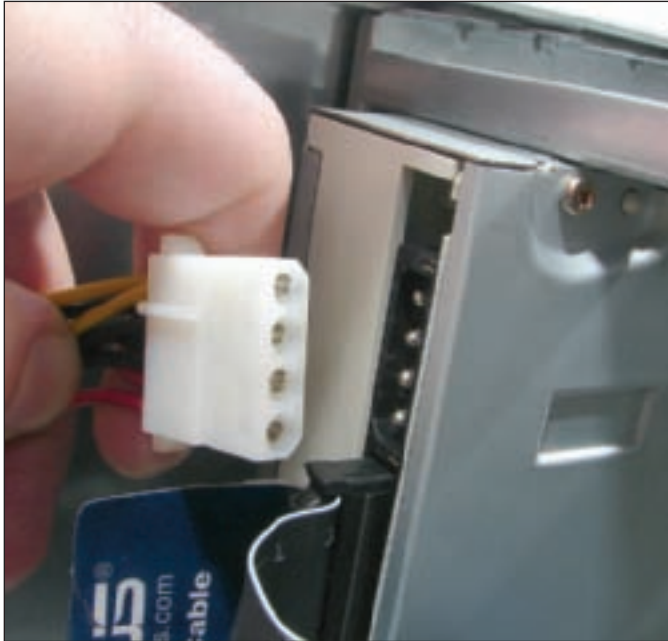
Figure 4-46 Molex power connector to a drive orients in only one direction Courtesy: Course Technology/Cengage Learning
