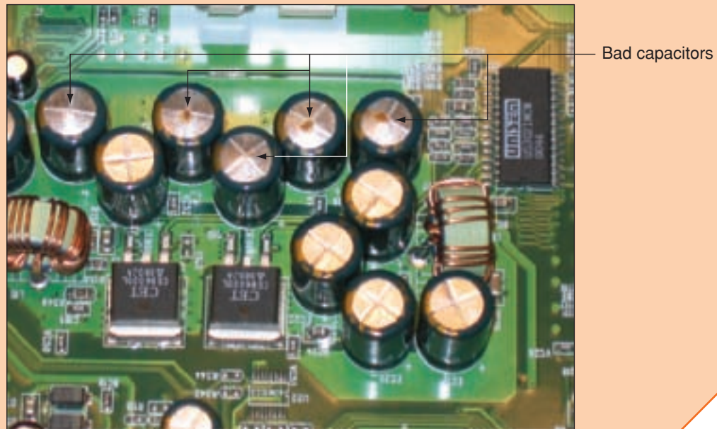
Figure 6-58 These five bad capacitors have bulging and discolored heads Courtesy: Course Technology/Cengage Learning
