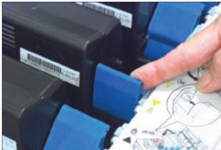
Figure 22-39 Push the blue lever forward to release the toner cartridge Courtesy: Course Technology/Cengage Learning
