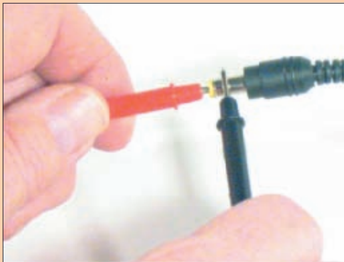
Figure 21-28 To use a multimeter to test this AC adapter, place the red probe (which, in the photo, is in the person's left hand) in the center connector and the black probe on the outside Courtesy: Course Technology/Cengage Learning
