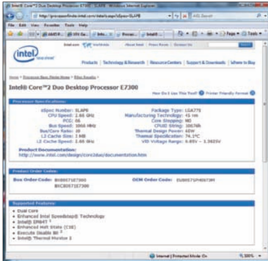
Figure 6-7 Processor Spec Finder using the Intel Web site Courtesy: Course Technology/Cengage Learning
