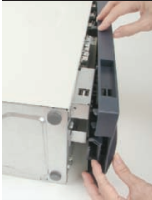
Figure 4-38 Newer cases require you to remove the front panel before removing the side panel of a computer case Courtesy: Course Technology/Cengage Learning
