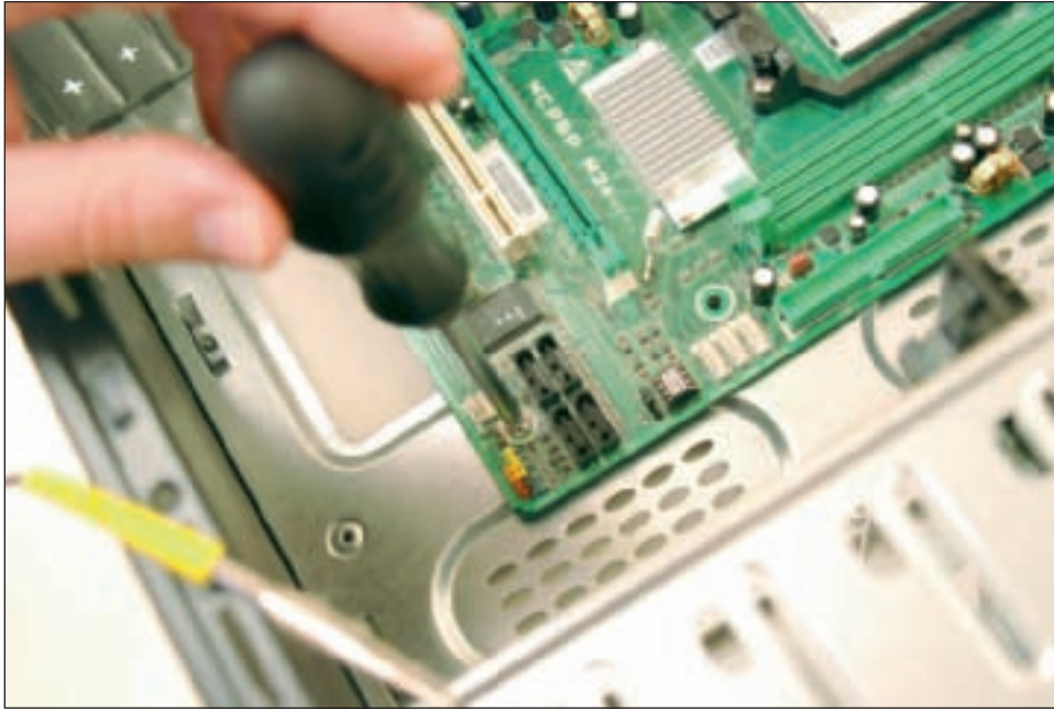
Figure 5-48 Use one screw in each screw hole on the motherboard Courtesy: Course Technology/Cengage Learning
