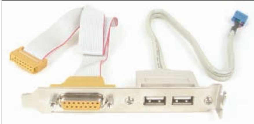
Figure 9-62 This connector provides two USB ports and one game port Courtesy: Course Technology/Cengage Learning
