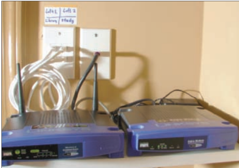
Figure 17-30 A router and cable modem are used to provide Internet access for a small network Courtesy: Course Technology/Cengage Learning
