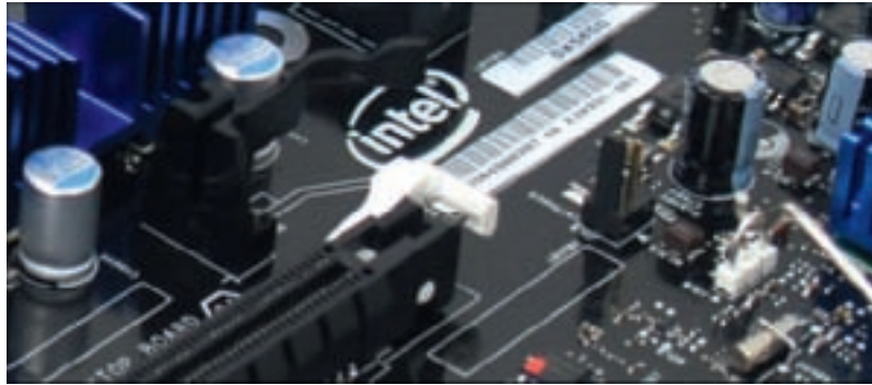
Figure 9-70 A white retention mechanism on a PCIe x16 slot pops into place to help stabilize a heavy video card Courtesy: Course Technology/Cengage Learning
