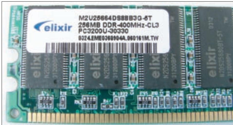
Figure 7-13 Use the label on this DIMM to identify its features Courtesy: Course Technology/Cengage Learning
