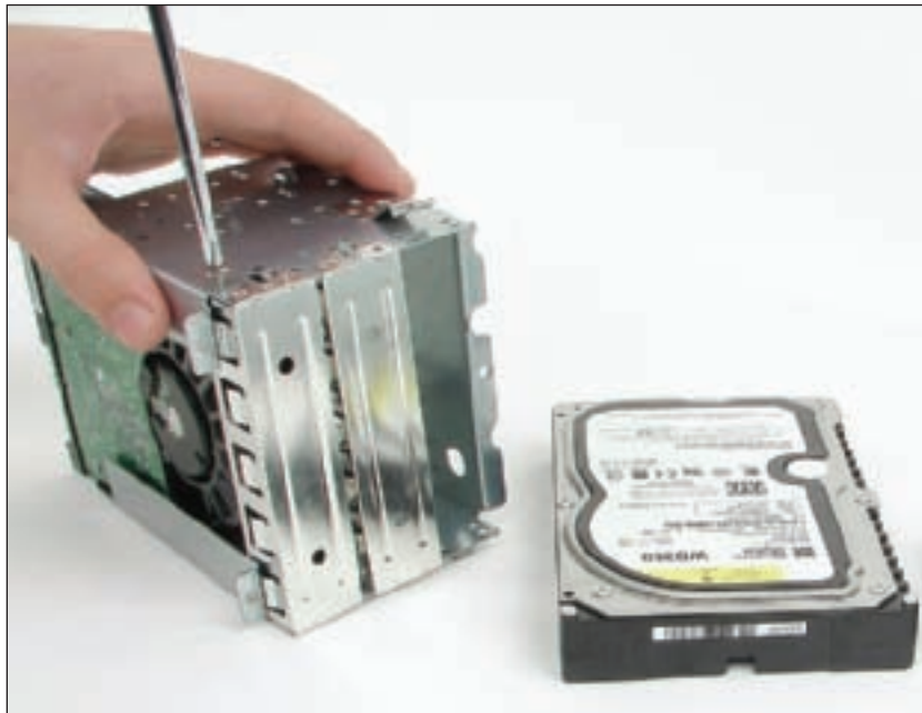
Figure 4-56 Drives in this removable bay are held in place with screws on each side of the bay Courtesy: Course Technology/Cengage Learning
