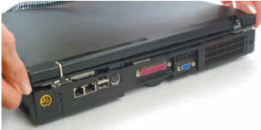
Figure 21-74 Cracking the notebook case Courtesy: Course Technology/Cengage Learning
