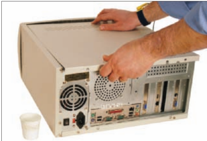
Figure 4-37 Slide the panel to the rear of the case Courtesy: Course Technology/Cengage Learning
