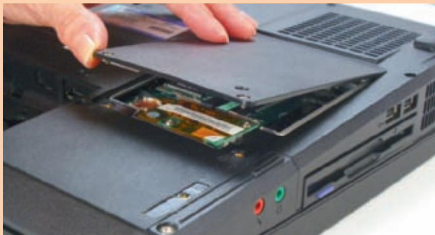
Figure 21-46 Raise the DIMM door on the bottom of the notebook Courtesy: Course Technology/Cengage Learning
