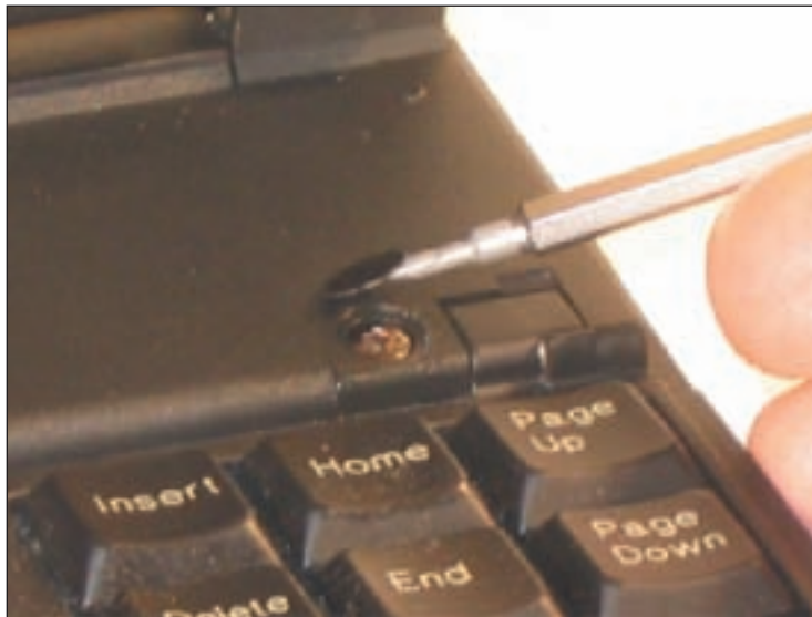
Figure 21-57 Use a small screwdriver or dental pick to pry up the plastic cover hiding a screw Courtesy: Course Technology/Cengage Learning
