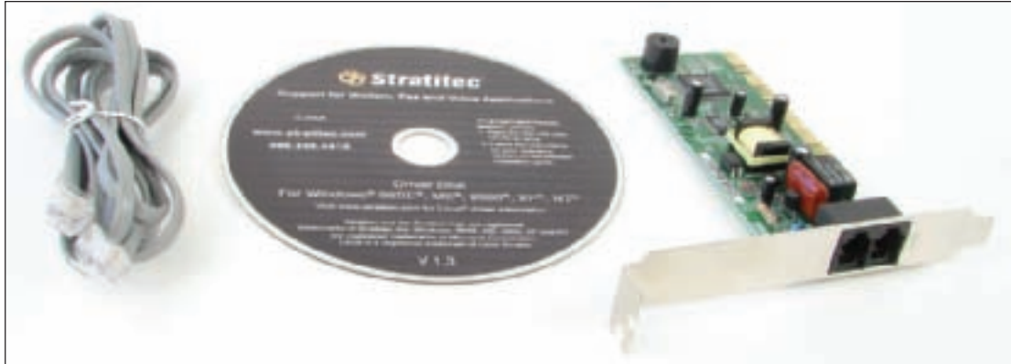
Figure 17-11 This 56K V.92 PCI modem card comes bundled with a phone cord and setup CD Courtesy: Course Technology/Cengage Learning
