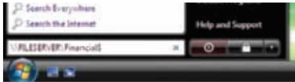
Figure 20-14 Accessing a hidden, shared folder on the network Courtesy: Course Technology/Cengage Learning
