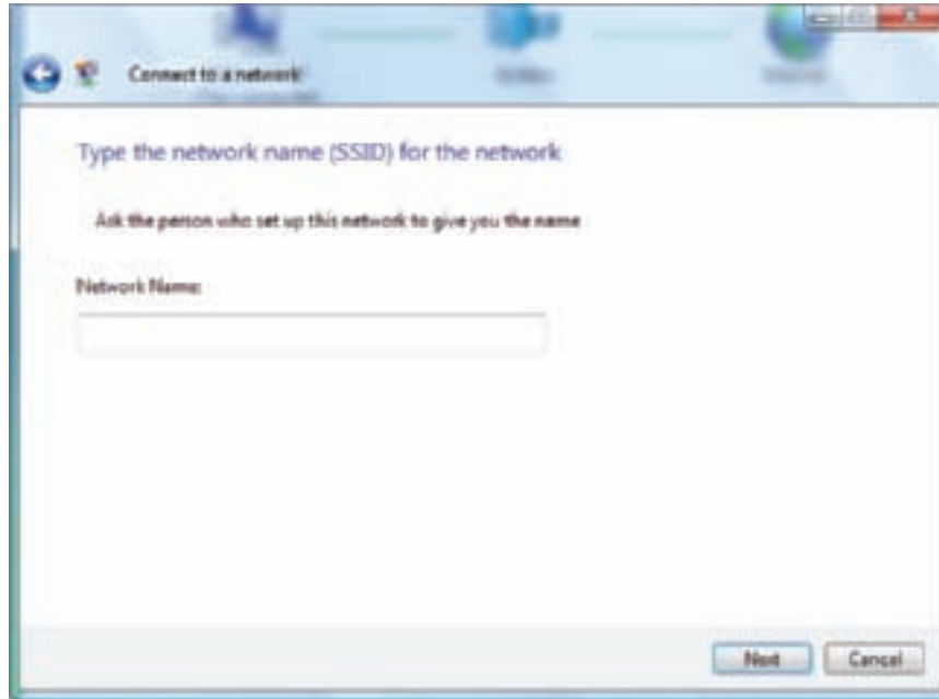
Figure 18-44 Enter the SSID of a wireless network that is not broadcasting its SSID Courtesy: Course Technology/Cengage Learning
