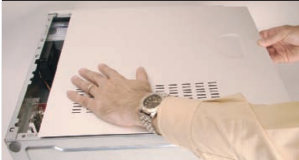
Figure 4-40 Slide the side panel to the front of the case and then lift it off the case Courtesy: Course Technology/Cengage Learning
