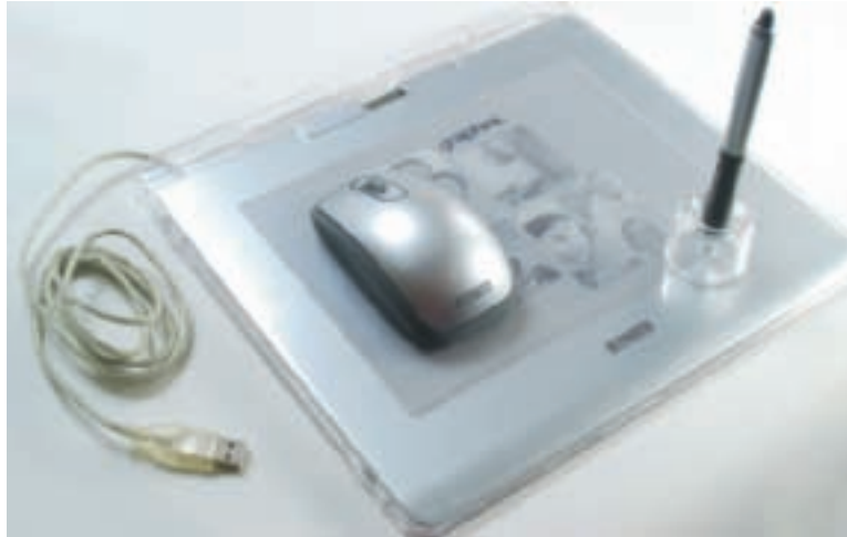
Figure 21-39 A graphics tablet and stylus are used to digitize a hand drawing Courtesy: Course Technology/Cengage Learning
