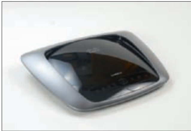
Figure 18-29 This router by Linksys allows computers on a LAN to share a broadband Internet connection and is an access point for computers with wireless adapters Courtesy: Course Technology/Cengage Learning
