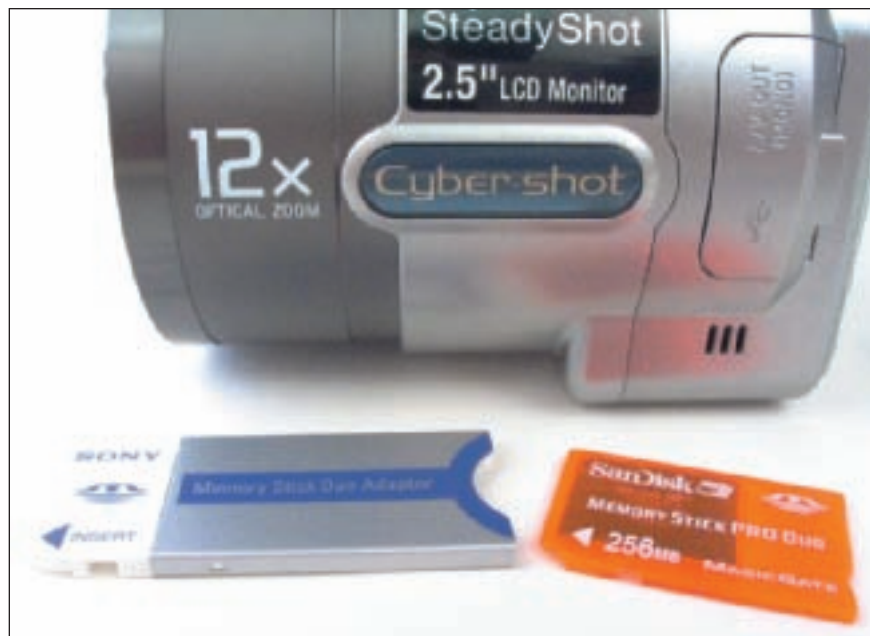
Figure 10-19 This Sony digital camera has a Memory Stick PRO slot that can accommodate a Memory Stick PRO Duo with adapter; images upload by way of a USB cable Courtesy: Course Technology/Cengage Learning
