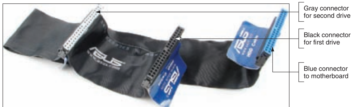
Figure 8-34 80-conductor cable connectors are color-coded Courtesy: Course Technology/Cengage Learning
