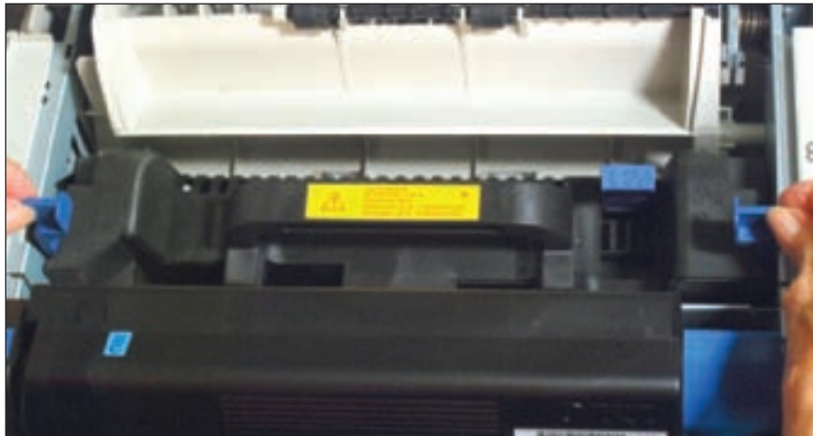
Figure 22-42 Pull the two fuser levers forward to release the fuser Courtesy: Course Technology/Cengage Learning
