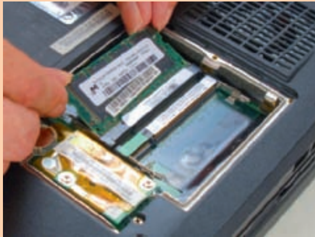
Figure 21-49 Insert a new SO-DIMM into a memory slot Courtesy: Course Technology/Cengage Learning
