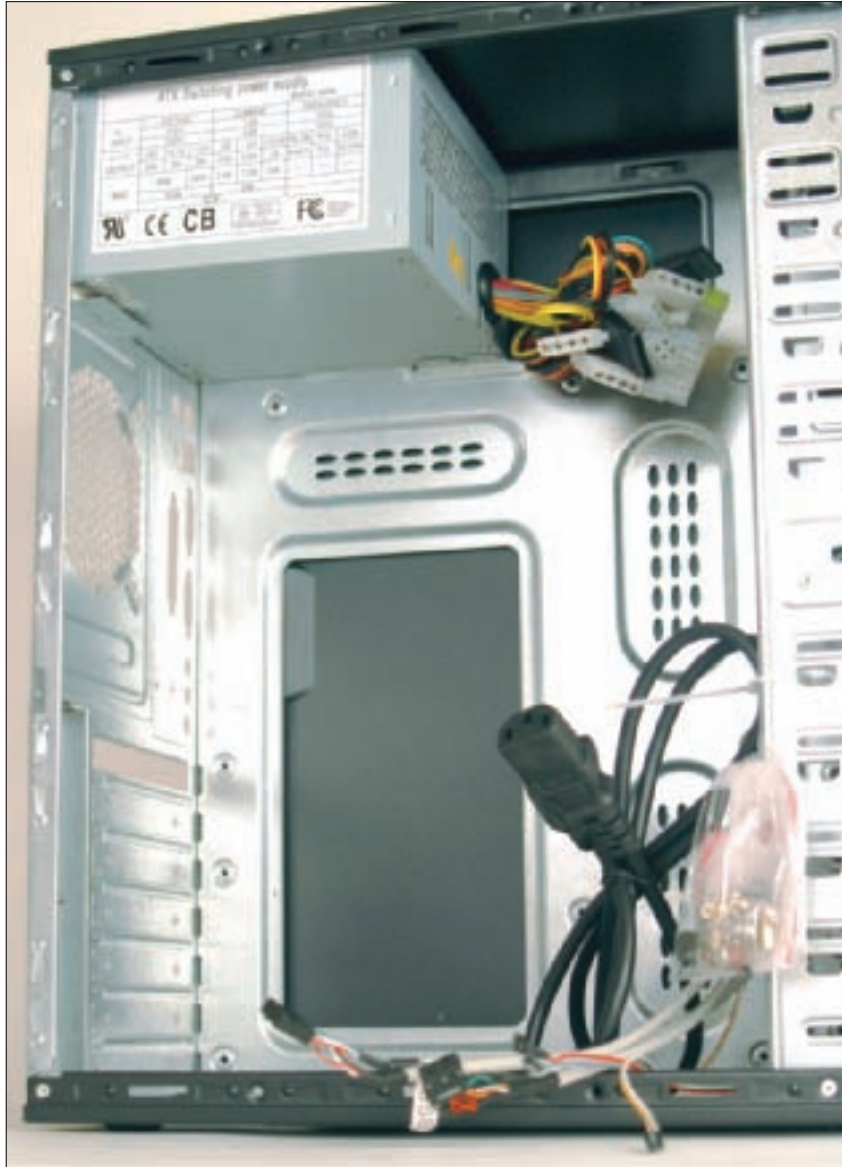
Figure 4-20 This case comes with a power supply, power cord, and bag of screws Courtesy: Course Technology/Cengage Learning
