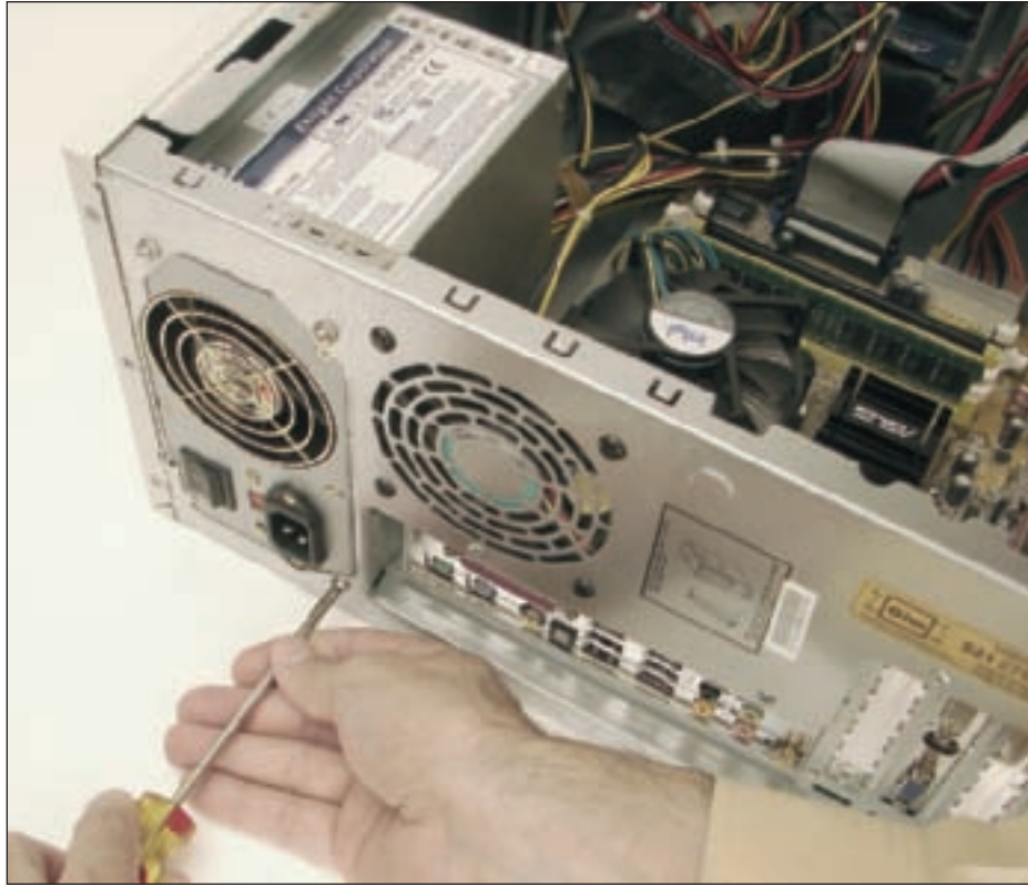
Figure 4-53 Removing the power supply mounting screws Courtesy: Course Technology/Cengage Learning
