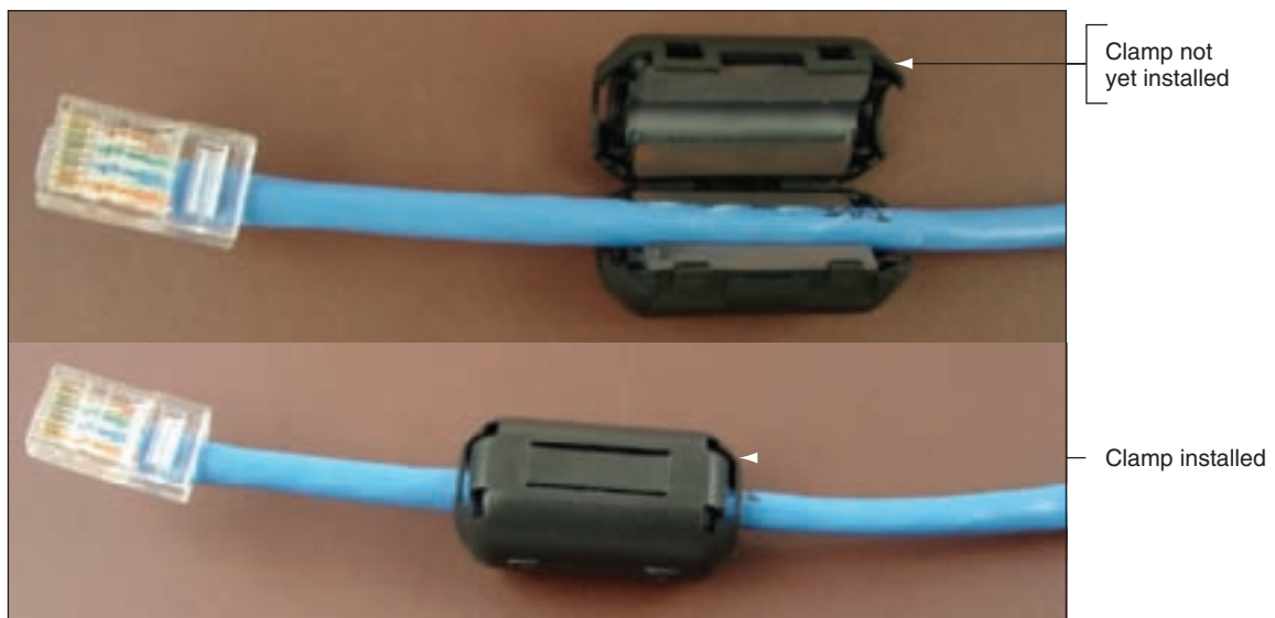
Figure 18-78 Install a ferrite clamp on a network cable to protect against electrical interference Courtesy: Course Technology/Cengage Learning
