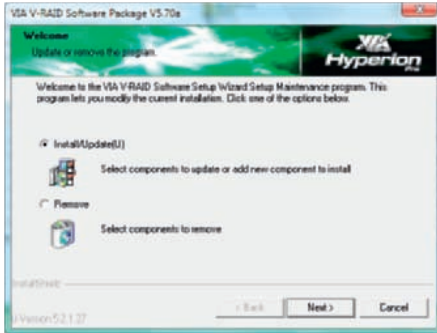
Figure 9-89 Use the Setup program on CD to uninstall the adapter card drivers Courtesy: Course Technology/Cengage Learning
