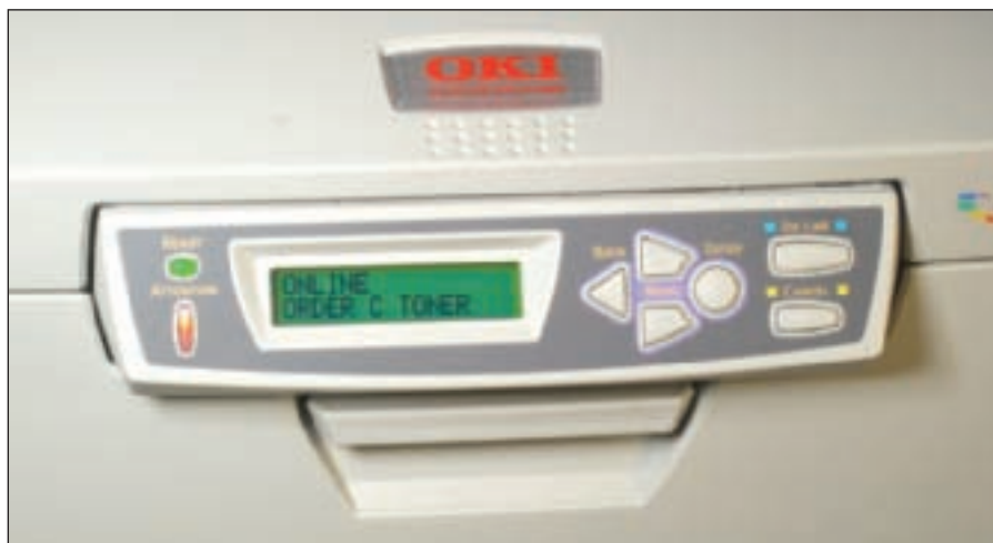
Figure 22-35 Use buttons on the front of the printer to display information, including the page count Courtesy: Course Technology/Cengage Learning
