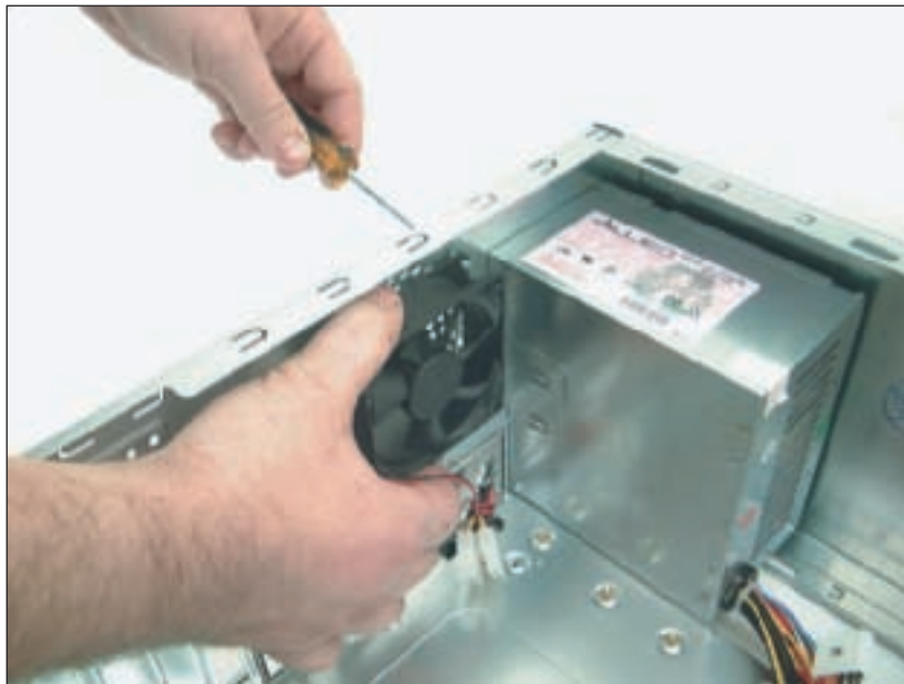
Figure 6-51 Install one exhaust fan on the rear of the case to help pull air through the case Courtesy: Course Technology/Cengage Learning
