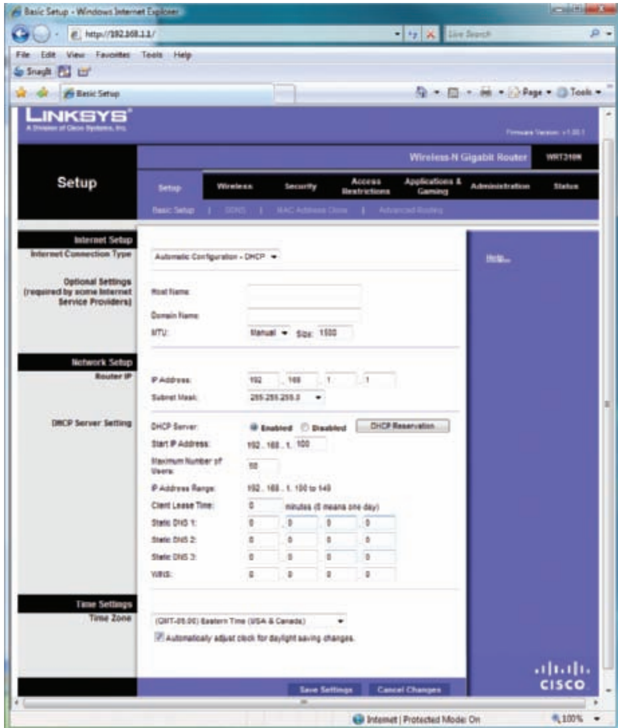
Figure 18-31 Basic Setup screen used to configure the router Courtesy: Course Technology/Cengage Learning
