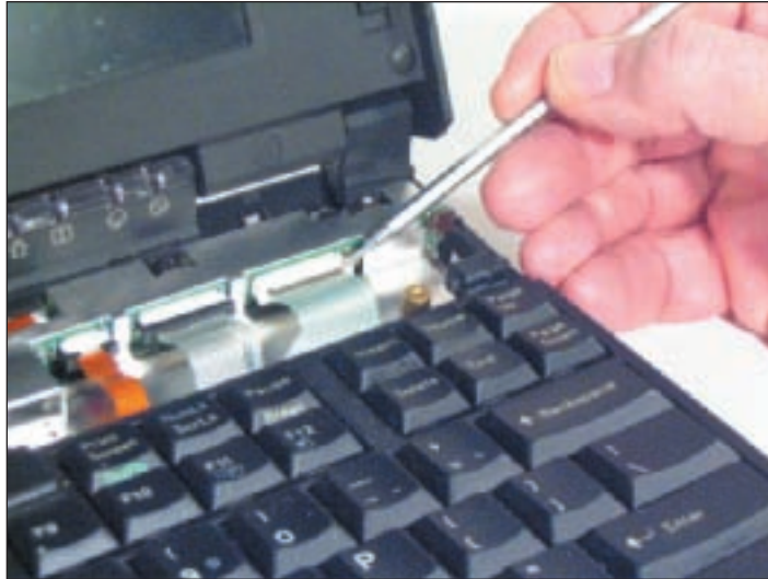
Figure 21-61 Three ZIF connectors hold the three keyboard cables in place Courtesy: Course Technology/Cengage Learning
