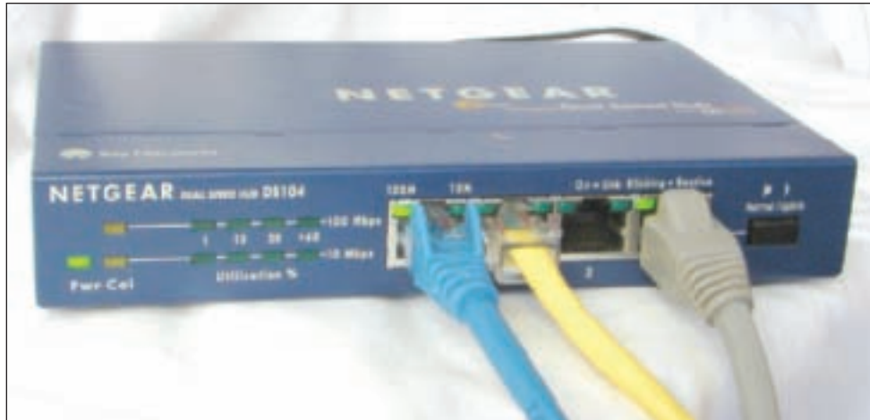
Figure 17-22 A hub is a pass-through device to connect nodes on a network Courtesy: Course Technology/Cengage Learning
