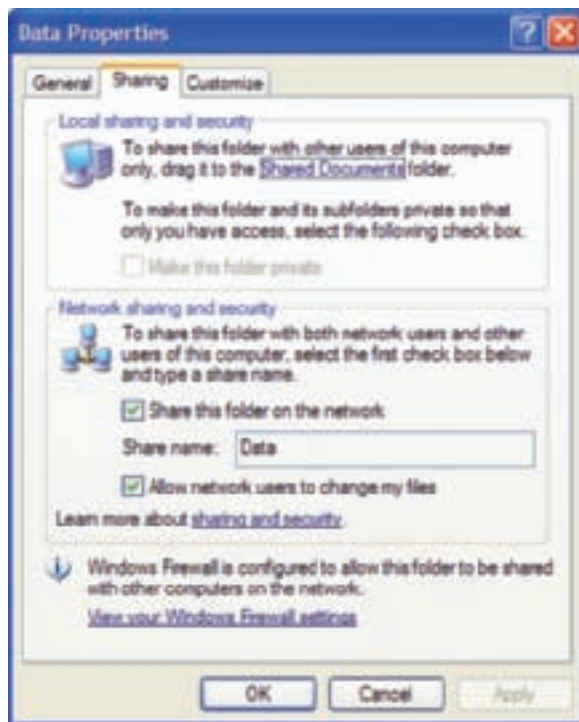
Figure 19-23 A user on a network can share a folder with others on the network Courtesy: Course Technology/Cengage Learning
