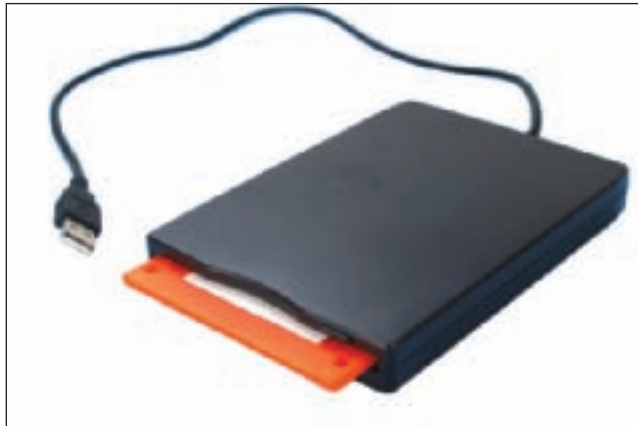
Figure 8-54 An external floppy drive uses a USB connection Courtesy: Course Technology/Cengage Learning
