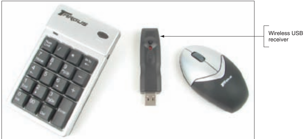
Figure 21-9 This wireless mouse and keypad use a receiver that connects to a USB port Courtesy: Course Technology/Cengage Learning
