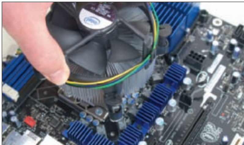
Figure 6-29 Align the cooler over the four holes in the motherboard Courtesy: Course Technology/Cengage Learning
