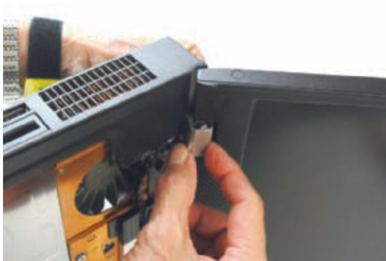
Figure 21-87 Remove the hinge cover from the notebook hinge Courtesy: Course Technology/Cengage Learning
