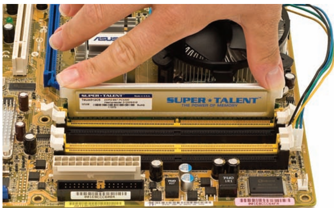
• Figure 7.34 Inserting a DIMM
