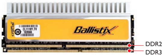
• Figure 7.17 DDR2 DIMM on top of a DDR3 DIMM
