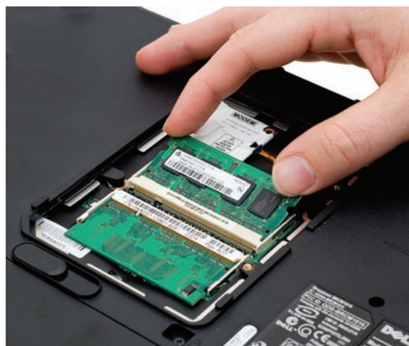
• Figure 7.40 Snapping in a SO-DIMM
