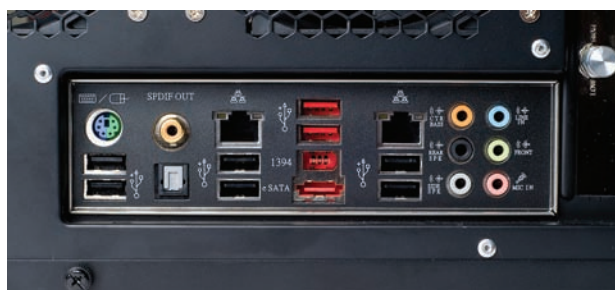
• Figure 3.33 Onboard connections
