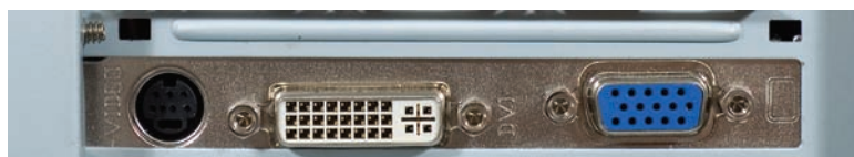
• Figure 3.20 Video card with (from left to right) S-Video, DVI, and VGA ports
