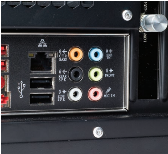
• Figure 3.22 Typical bank of 1/8-inch audio jacks
