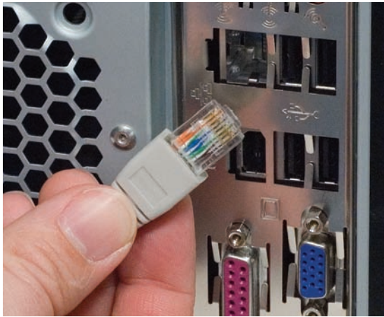
• Figure 3.25 Typical network connection
