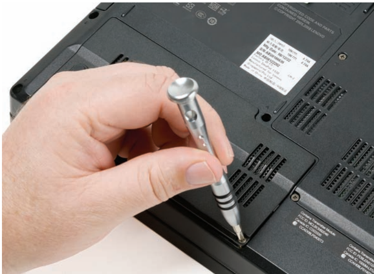
• Figure 26.49 Removing the drive compartment cover
