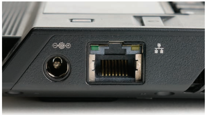
• Figure 26.20 Ethernet port on laptop
