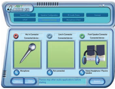
• Figure 25.25 Autosensing software detecting connected devices
