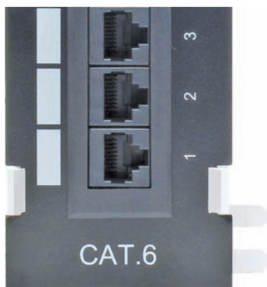
• Figure 22.21 CAT level on patch panel
