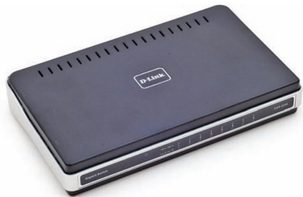
• Figure 22.6 Typical switch
