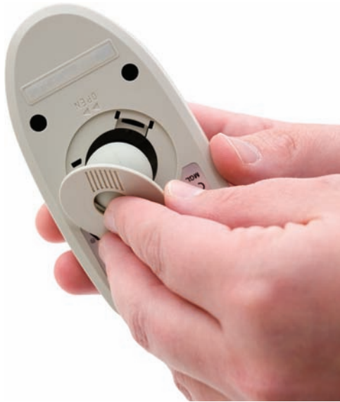
• Figure 20.26 Removing the collar on a ball mouse
