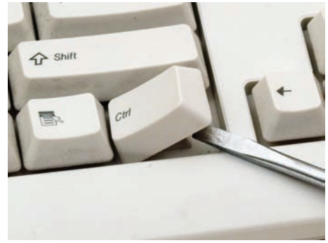
• Figure 20.24 Prying off a key
