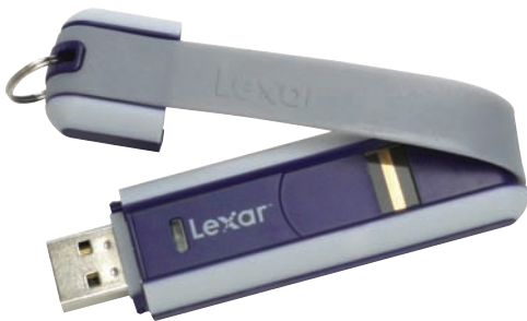
• Figure 20.35 USB thumb drive with fingerprint scanner (photo courtesy of Lexar Media, Inc.)
