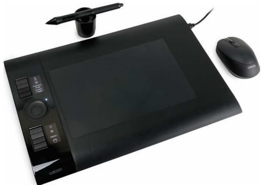
• Figure 20.43 A type of digitizer known as the Wacom pen tablet
