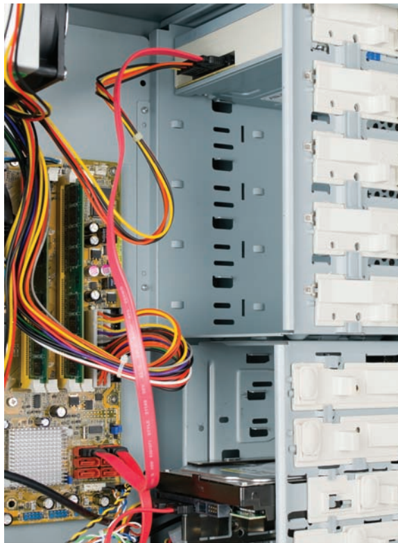
• Figure 13.30 Typical DVD installation
