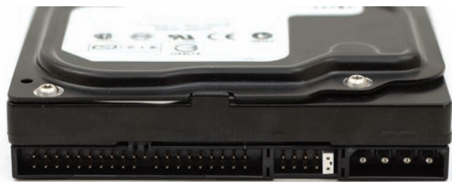
• Figure 11.8 Back of IDE drive showing 40-pin connector (left), jumpers (center), and power connector (right)
