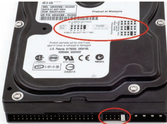
• Figure 11.10 A typical hard drive with directions (top) for setting a jumper (bottom)
