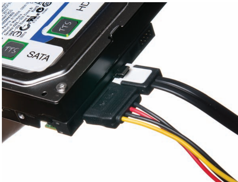
• Figure 11.43 Properly connected SATA cable
