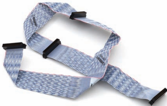
• Figure 11.27 Typical 68-pin ribbon cable
