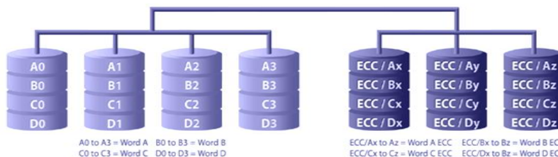
RAID LEVEL 2 : Hamming Code ECC
