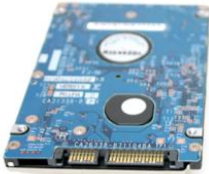
SATA drive (has card-edge connector)
